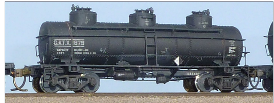
35. An assembled but undecorated Tangent model was painted and lettered with Black Cat decals to represent a car repainted before 1946 with lines above and below the reporting marks and numbers. Weathering includes dirty wheels with treads polished, rust stains around the tank bands, chalk marks, spillage on the domes, and rusty couplers. Model and photo by the author.
