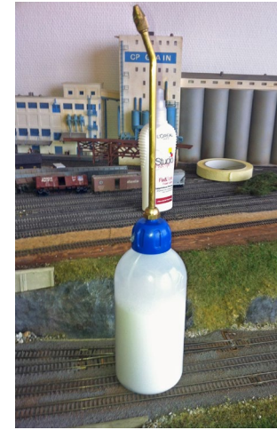
4. Oil can with fully extended nozzle. The hair spray can in the background holds "wet" water. Andy Kesselkaul photo
