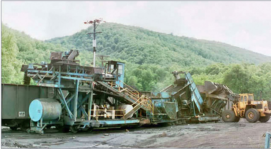
2. Photo of a prototype machine from the left front. The coal is loaded into the receiving hopper with a front end loader.
