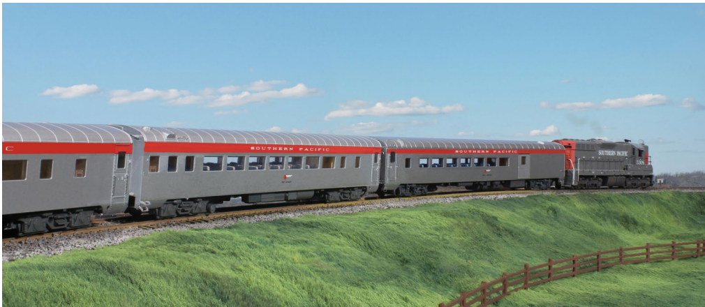
18. In its last years, the Sacramento Daylight consist was usually all lightweight with rebuilt Daylight-type chair cars and baggage chair, here approaching Lathrop circa 1966.
