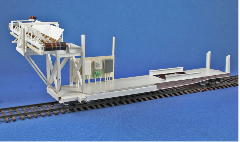
28. Machine deck with transfer conveyor added.
