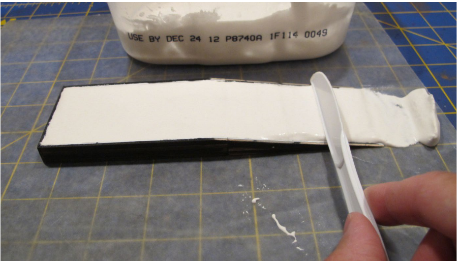
15. Once the frame was filled I used a plastic knife to gently level the Hydrocal on top of the ramp.
