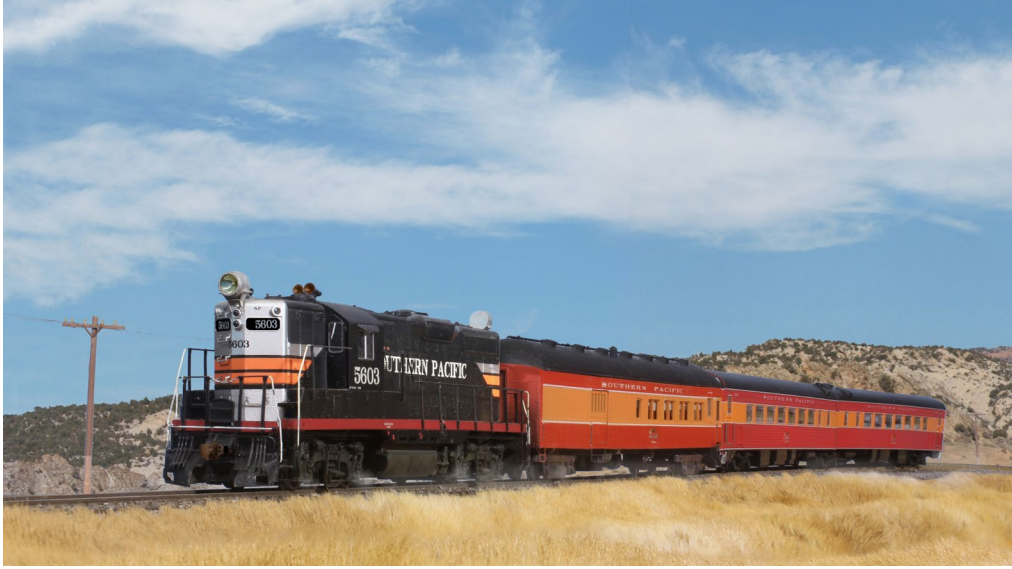
16. By the mid '50s the Sacramento Daylight was dieselized. It is shown here with passenger-equipped GP9 5603, a combine, and an articulated chair car pair.
