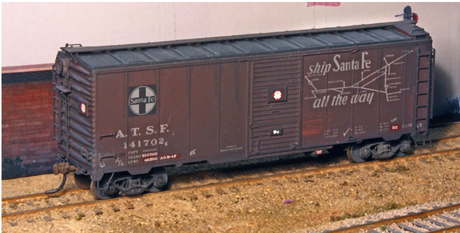
9. Santa Fe's biggest class of steel boxcars was Bx-37, 5,010 cars strong. This is an Innovative Model Works kit product, built and weathered by Richard Hendrickson. Note door and end placards, and scraped paint next to the door.
