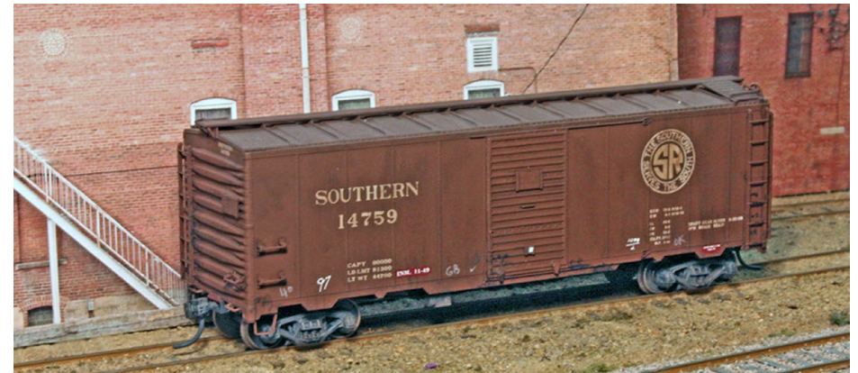
22. This model, built from an Innovative Model Works (IMWX) kit, represents one of the Pullman-Standard-built cars among the 8,500 cars purchased by Southern before World War II, all with only 40 tons capacity. It carries the pre-war Southern emblem.
