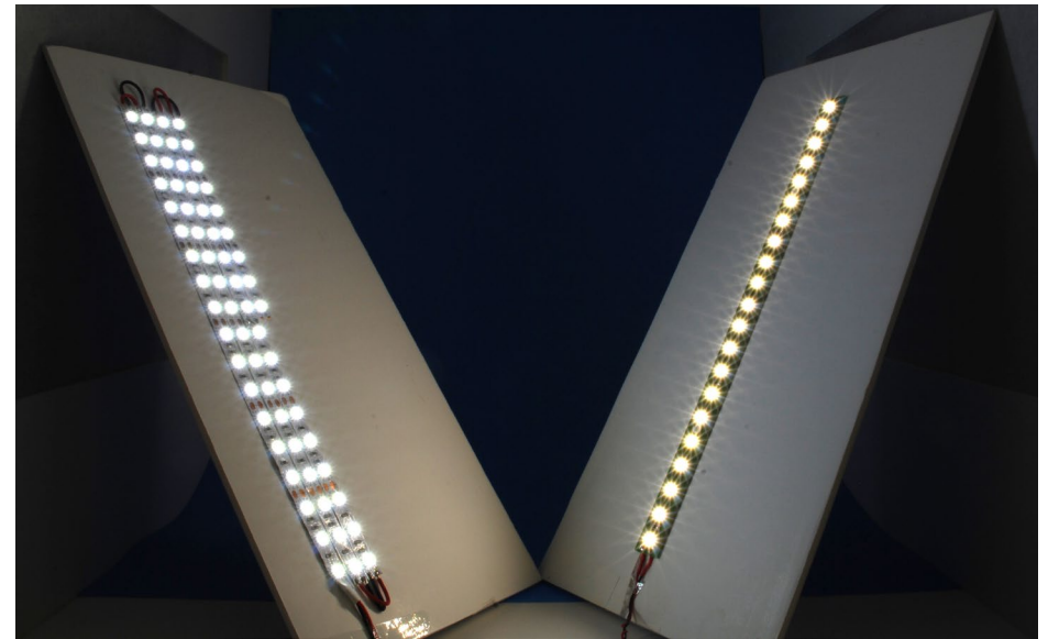
2. Comparison between 5050 LED strips, and the LED board.
