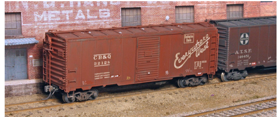
17. This model represents one of the 5,000 cars built by the Burlington at its Havelock shops during 1940 through 1944, all with W-corner-post ends. It is an InterMountain ready-to-run model.
