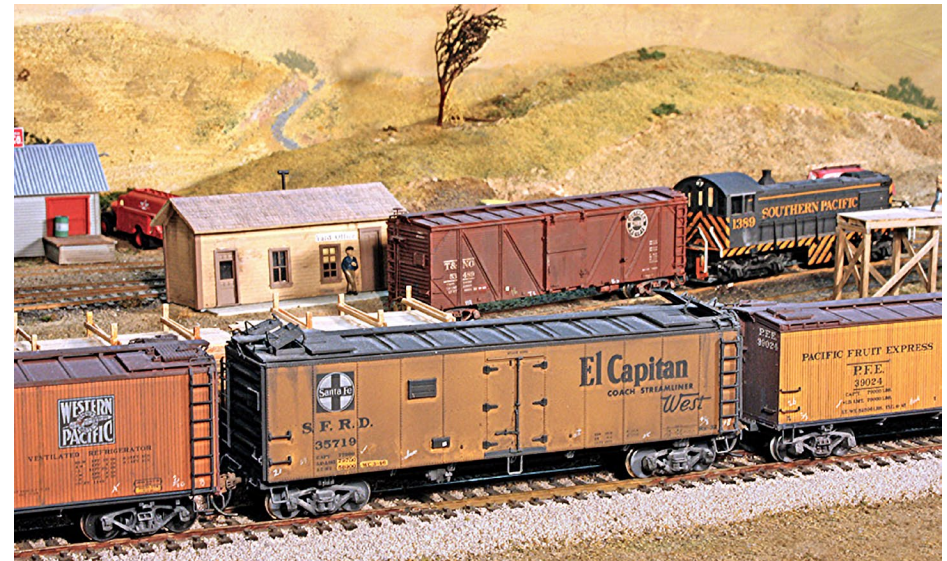
10. A representative of 18,000 refrigerator cars operating under SFRD reporting marks, this model of class RR-32 shows the inward-opening ice hatches standard in SFRD practice until the 1950s (they were later reversed to accommodate icing machines). It was built from an InterMountain kit by Richard Hendrickson.
