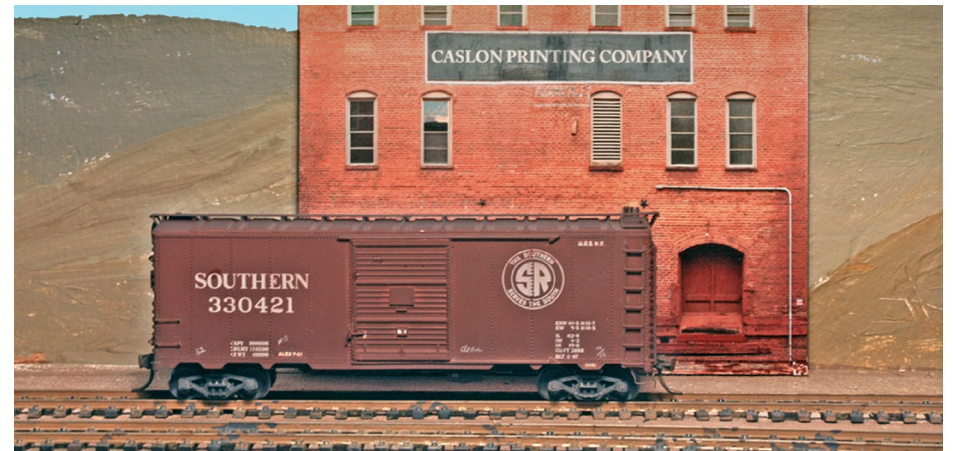
23. After World War II, Southern was among the pioneers of the 8-foot door on boxcars, as represented in this model. It was built from a C&BT Shops kit with upgraded details, and is lettered (top right corner) for one of Southern's subsidiaries, the New Orleans & Northeastern (NO&NE). It also has the 1945 emblem.
