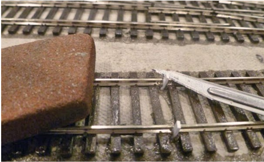
7. Trimming the top and sides of the styrene strip.
