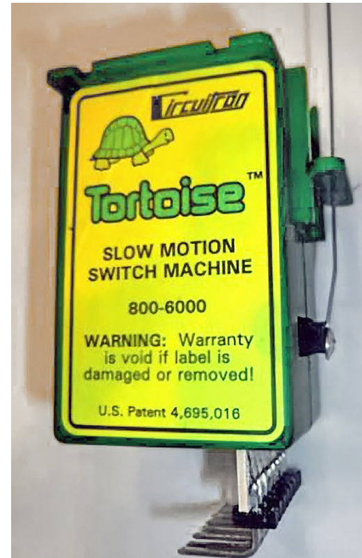
16. Tortoise switch machine assembled with header installed.
