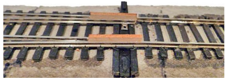
29. Place strip wood between the point and stock rail on each side.
