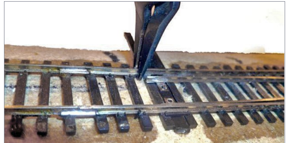
23. Making a slight bend in the stock rail.
