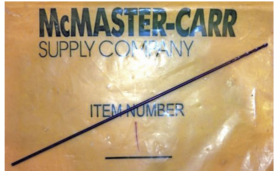
3. Six-inch drill for feeder wires.
