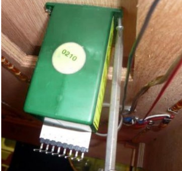
21. Driving mounting screws for the tortoise.
