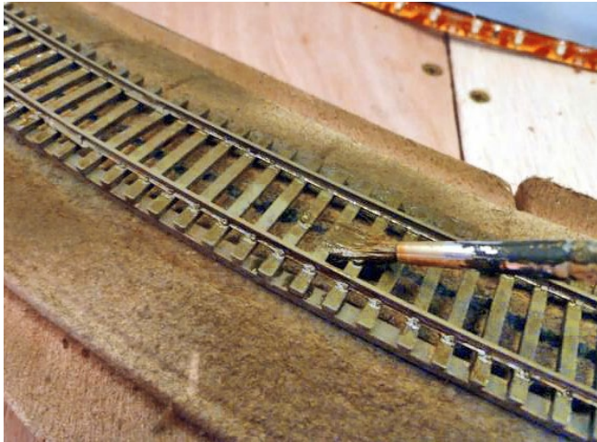
34. Paint all the ties with Oak Stain.
