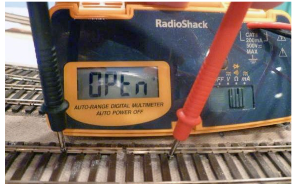
4. Checking for shorts.
