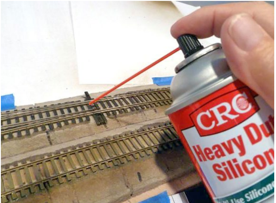
28. Applying silicone oil to the throw bar.
