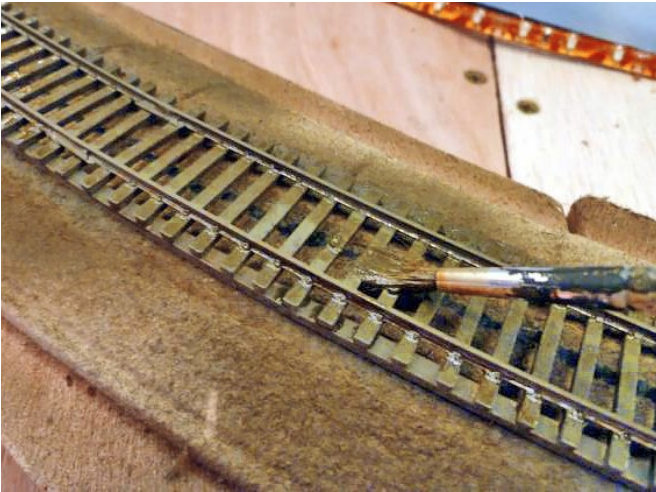
34. Paint all the ties with Oak Stain.
