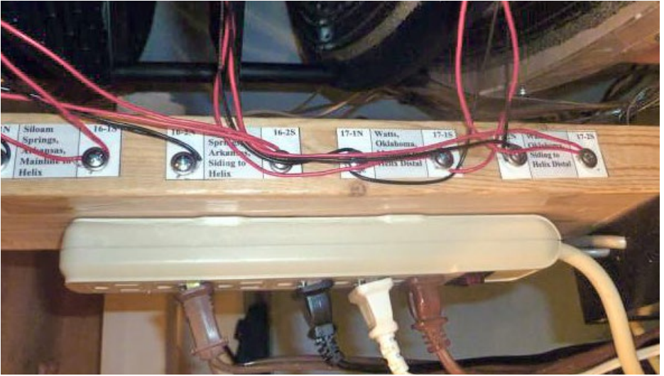
13. Terminal board for the helix and return loops.
