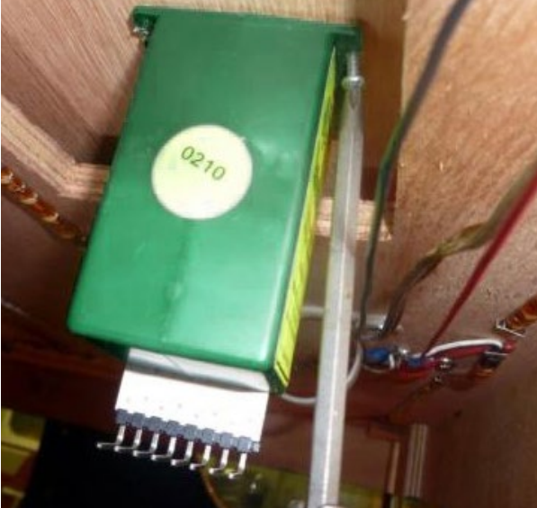
21. Driving mounting screws for the tortoise.
