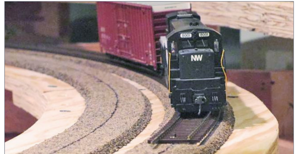
3. A 1/32" shim at the outside edge of the ties the rail produces a less obvious effect in HO. Paul Krentz photo
