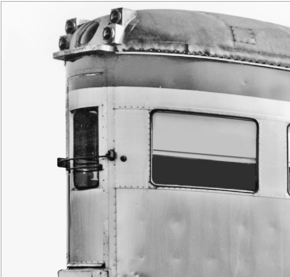
10. Lighting array of car SP 2951 with platform after car is rebuilt with flat stainless steel panels in the 1960s.
