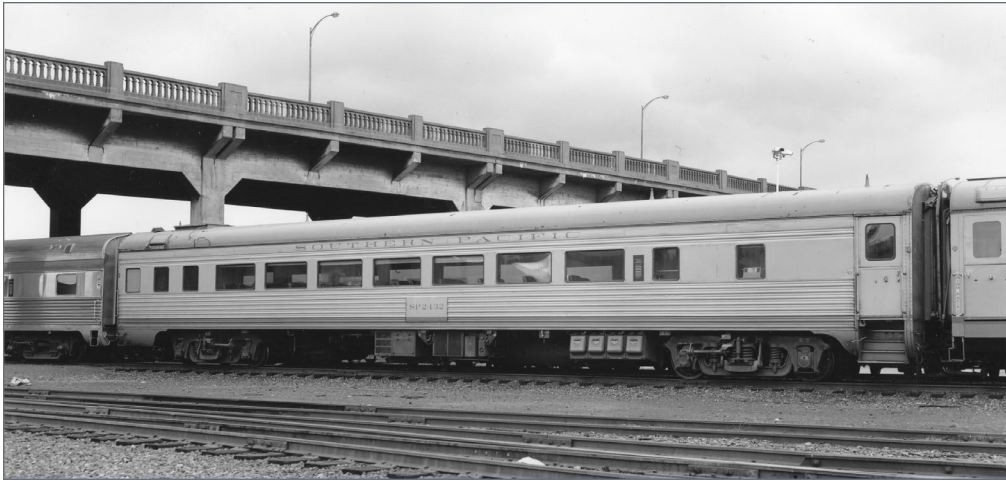
17. Chair car in the later lettering for Overland service, car 2432 in class 77-C-3. The drop-equalizer type trucks are replacements, usually taken from a scrapped sleeping car. The car still has its original fluted sides. Courtesy Bob's Photos
