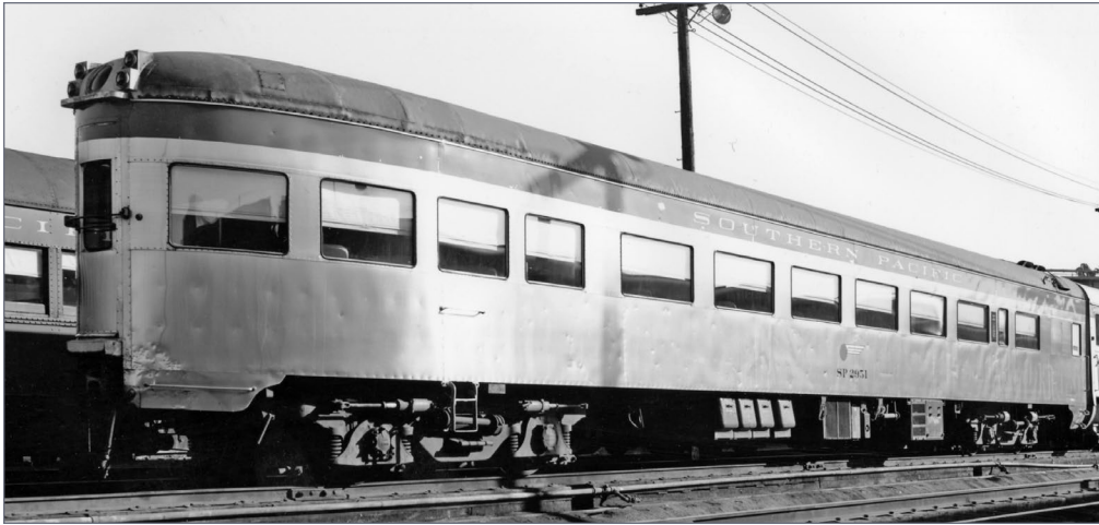
19. Parlor car 2951, class 77-PRO-1 parlor observation in its final configuration shown in San Francisco as of April 1971. The car has late box type rear lighting array, flat stainless steel sides with red letterboard stripe, and Waukesha air conditioning. Propane bottle containers show under the car. This car still has its triple bolster trucks.
