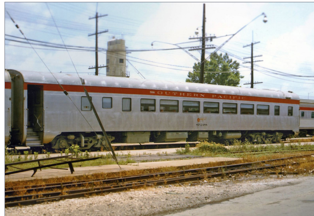
21. Prototype chair car 2488 (class 79-C-2) in 1969 as rebuilt with flat stainless sides, but with its original triple bolster trucks.
