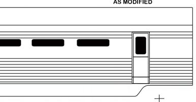
As built, there was a single kitchen door and two loading windows. This was changed with an additional door replacing each loading window.
