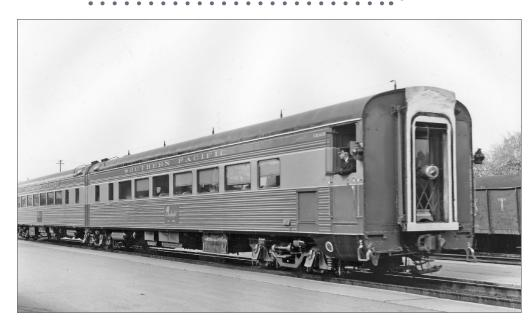
14. SP 2471+2472 articulated chair car pair, class ACW-66+ACM-66, shown in 1955. The retracted staircase in the rotating unit is shown, and at left is the baggage elevator door. *Courtesy Bob's Photos*
