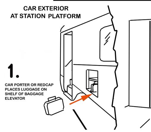
13. Baggage elevators were used to prevent delays at stations. In lowered position they could be accessed from the outside sliding door, and when raised, the carry-on luggage was accessible for passengers in the car.
