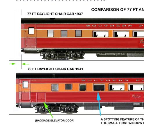
22. Comparison of 77 foot cars built 1937 and 79 foot chair cars built 1939-41. The additional length accommodated the new baggage elevators. Articulated cars were also longer when constructed with baggage elevators. Before World War II, there were no established standards for the length of lightweight cars.
