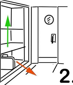
LUGGAGE SHELVES ARE RAISED AND CARRY-ONS CAN BE ACCESSED BY PASSENGERS IF DESIRED The railroad developed electric baggage elevators (dumbwaiters). Passengers would hand carry-on luggage to redcaps on the platform. Luggage was placed on shelves of the baggage elevator, and was raised. The shelves could then be accessed by passengers inside their car at any time. No other railroad used baggage elevators.
