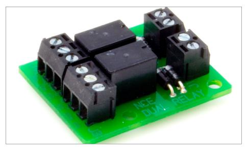
16. An NCE Dual Relay board is a way to control higher power items from your throttle or computer.
