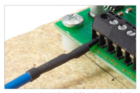
13. Large gauge (16 AWG) stranded bus wire pigtailed with smaller gauge (20 AWG) solid wire to connect to a stationary decoder.
