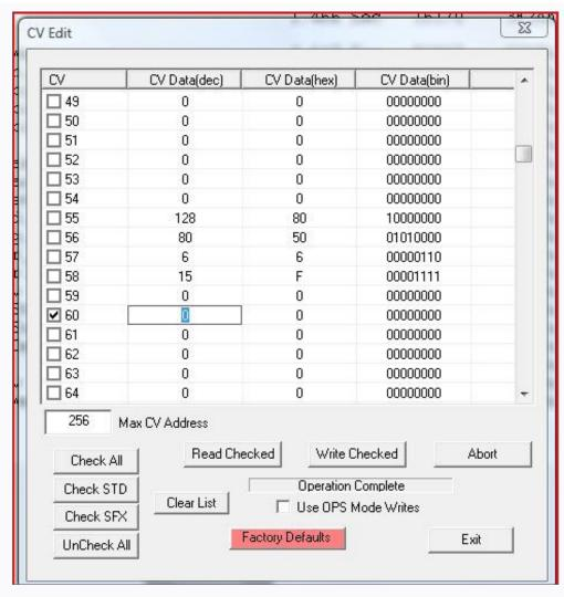
E The CV Editor can be used to read and write most configuration variables (CVs). In this screenshot, I am about to change CV60 from 0 to 1 to test the diesel sound scheme. The CV Editor can also be used to accomplish a factory reset with the use of the Factory Defaults red button. This restores the CV values, NOT the sound project file. ☑
