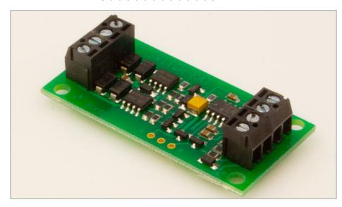
9. The NCE Switch-Kat is for single coil snap motors, like Kato or LGB.
