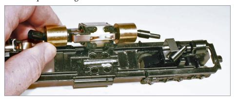
10. Electrical power to the motor was designed to flow from the unpainted strip on the chassis to the copper strip on the bottom of the motor. The motor must be isolated from the frame for DCC. The lower motor lead must be connected to the motor output lead from the decoder, not to track power via the frame.
