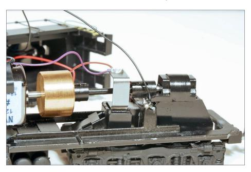
13. A solder connection is made to the chassis for providing track power to the decoder (black wire). A small set screw could also be used, by drilling and tapping a hole in the chassis. The purple wire, connected to the other truck, and the red wire to the decoder provide power from the other set of wheels.
