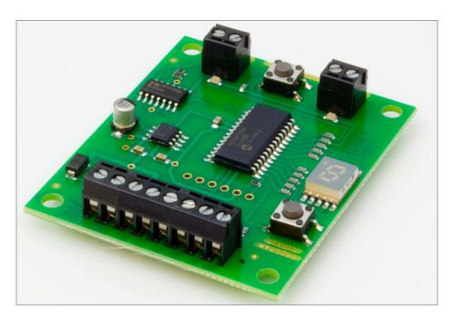
5. NCE's Switch-It MK2 decoder for two stall motors.
