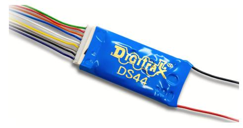
1. Stationary decoder: the Digitrax DS44 looks a lot like an HO mobile decoder, just with more wires. It handles four stall motors. Digitrax photo
