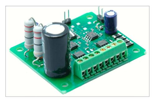
8. Digitrax has the DS52 for any style snap motor or two stall motors. Notice the large storage capacitor in the front. Digitrax photo
