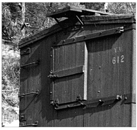
5. A close-up of 612 shows the details of the end door in the A end. ORER entries list end doors on all three of the cars. Guy Dunscomb photo
