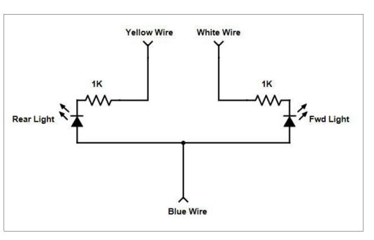
5. Wiring schematic for the front and rear headlight LED lighting circuit.
