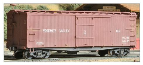
16. Based on prototype photos, this car was completely repainted and relettered after arrival on the YV. The lettering includes safety appliance lettering above the left truck, the road name initials and car number on the side door, and capacity data above the right truck.
