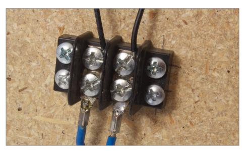
14. Large gauge (16 AWG) stranded bus connected through a barrier terminal strip to a smaller gauge (20 AWG) solid wire.
