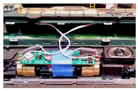
48. Here's the RailMaster 1425-8 speaker installed, and headlight wiring in place. After testing the headlights one more time, shrank the heat-shrink tubing. I perform assembly like this on a Bowser foam locomotive cradle, with the chassis in the gully and the body shell sitting above and behind the chassis. I leave enough extra wire to easily make the solder connections. If the need to disassemble arises, it's easy to remove the shell and set it out of the way on the Bowser cradle.
