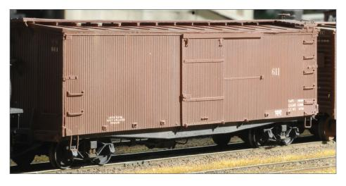
15. Like the prototype, this car was not lettered with the road name. The ends of the horizontal tie rods are readily visible. These cars were not allowed in interchange service so there are no "chalk marks" on them indicating routing and other information typically added by clerks or other railroad workers.
