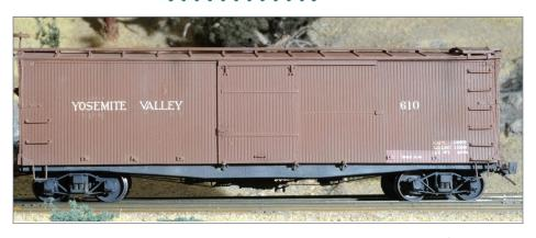
14. YV box car 610 along the line. Based on photos of the prototype, I suspect the YV repainted this car when they bought it, but did not overpaint the dimensional data on the bottom right side of the car. I therefore painted this area of the car a light box car red. This area was then masked while I painted the rest of the car before applying the decal lettering.
