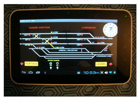
6. Quaker Junction local panel on an Android tablet.
