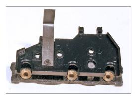
7. Electrical transfer is made from the wheels' axles through the brass contact plates on the outside frame, and then via the L-shaped bracket which originally rubbed the headlight/top of motor connection strip.
