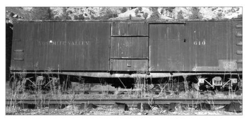
2. YV 610, one of the three ex-SP B50-1/2/4 box cars on the roster, at El Portal. The black side sill is very light, suggesting that it was not repainted by the YV after purchase. The rest of the car was repainted by the YV. The area with the capacity data on the bottom left of the car appears to have been left untouched. Stanley Snook photo
