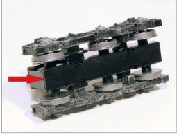
3-4. The upper and lower clips hold the truck assembly together. Use of a thin blade screwdriver along the edge of each will pop the clips off.
