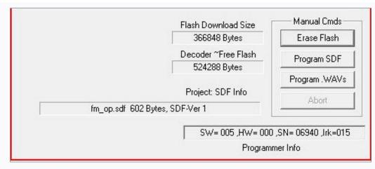
D. Lower right corner of SoundLoader main screen after accomplishing an Erase Flash command. Note that the available (free flash) memory is 524,288 bytes.
