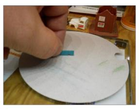
4. Use sandpaper on a self-adhesive orbital sander disk, laid against a piece of glass, to get a totally flat and true surface.
