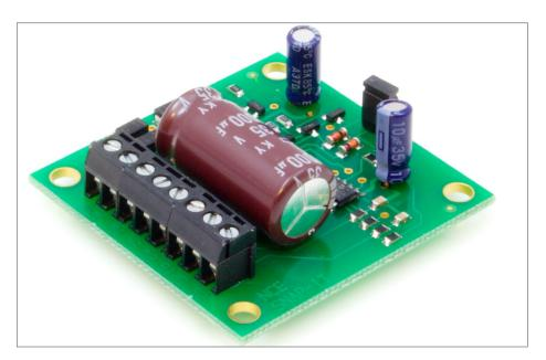
10. NCE's Snap-It will handle one dual-coil snap motor.
