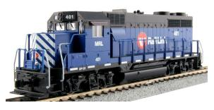
Features include directional headlights, all-wheel electrical pickup, blackened metal wheels, and preinstalled handrails. The DC models come with an 8-pin plug for instal-
