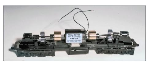
12. Reassembled drive train with replacement motor. Clear silicone adhesive and sealant was used to attach the motor to the frame.
