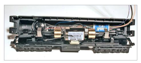
3. Prior to installing the lights, check the positioning of all the components in the hood to ensure adequate clearance for the drivetrain.
