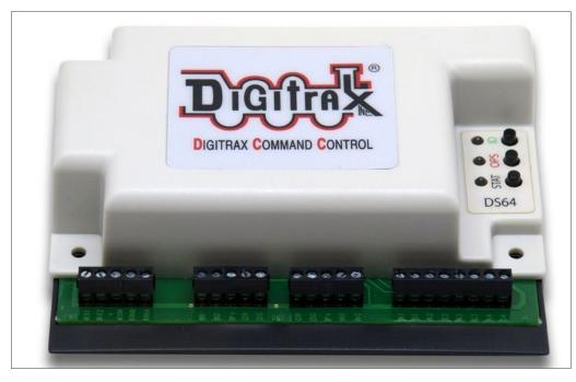
3. Digitrax DS64 has it all. It will work with any turnout motor except a servo, accepts fascia switch inputs and provides LocoNet feedback. Digitrax photo
