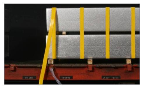
28. Once you are satisfied with the placement of the tape, pull it aside from the stake pockets and permanently glue it with CA onto the face of the stake pocket.
