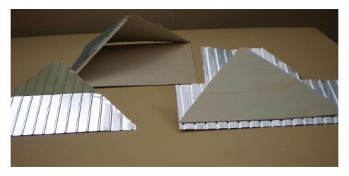
5. Progressive assembly of the pyramidal roof for the house. The right section has the ribbed seam roofing glued in place waiting for trimming. The left roof piece has been trimmed and one section painted ready for installation. At the back is the roof with two sections already installed, but still requiring it to be tacked into place.
