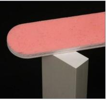
9. After trimming the excess styrene the rough edges on the sides and ends can be smoothed with a file.
