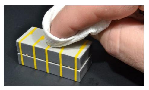
17. After the CA cement is applied, spread it with a paper towel. This will soak up any excess cement.
