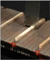
23. Any high spots found, once the runners are mounted to the flatcar deck, can be fixed by gently whittling on the soft wood of the offending runner.
