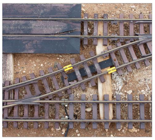
7. Rail gaps on the RMP before painting the yellow joiners. Note: black plastic strip screwed to ties to hold gaps together. Note, also: black feed wires connected to Split Jaw clamp with stainless steel socket head screws.
