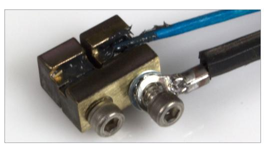
11. Connection of the feed wire to the Split Jaw rail clamp. Ox-Guard has been applied to the mating surfaces with the blue toothpick, shown.
