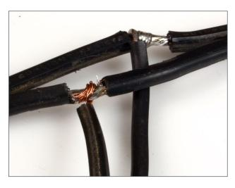
12. Connection between drop wires and bus wire. Two joints are shown in the photo. In the upper right is a completely soldered one – note the bright and smooth surface, indicating that enough heat has
