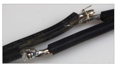
14. Butt splice in bus wire. Lower left has been wrapped with smaller solid wire and soldered. The
