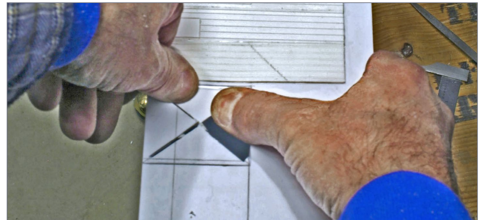
24. Once the X is cut, scribe the top, bottom and sides of the opening to snap out the waste pieces.
