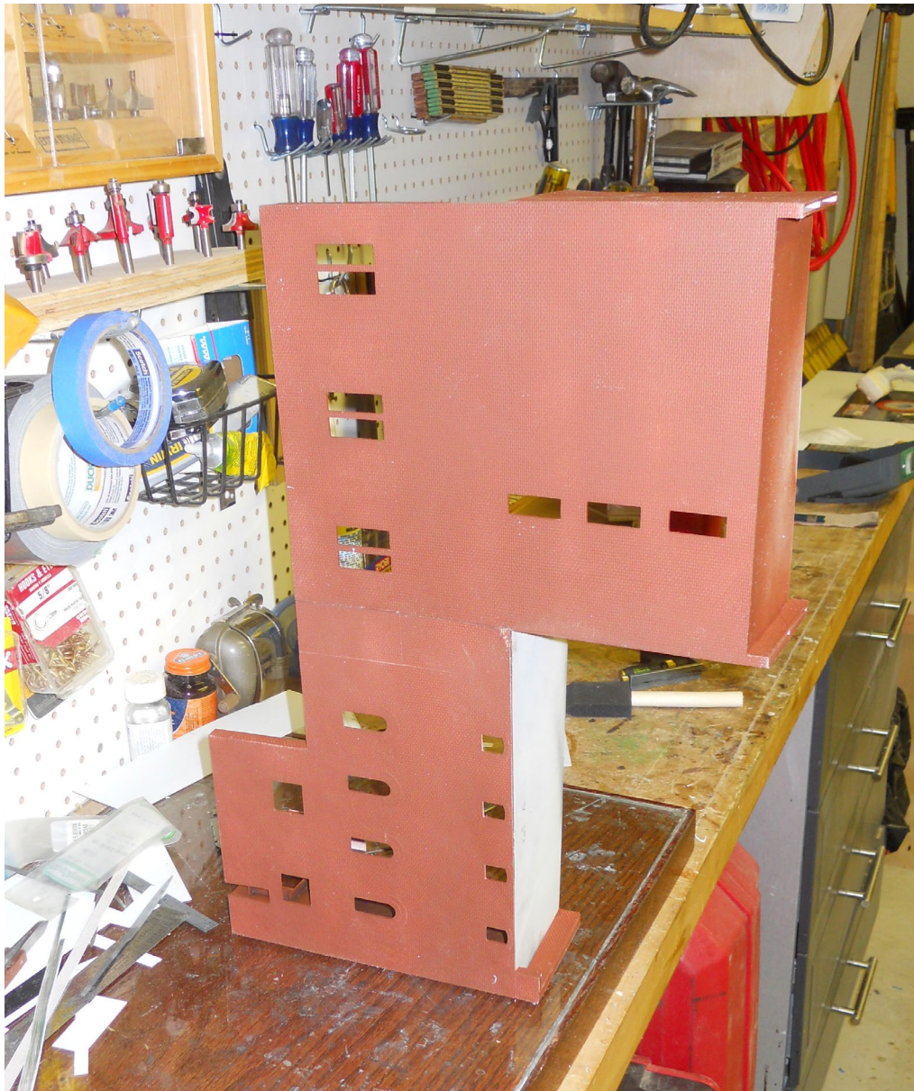
26. The center section has been cemented to the right wing. The structure is becoming rather large and awkward at this point, requiring a little creativity to glue things together.
