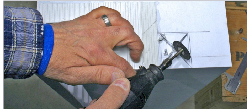
23. A Dremel tool and cutting disc make quick work of prep- ping the door openings.
