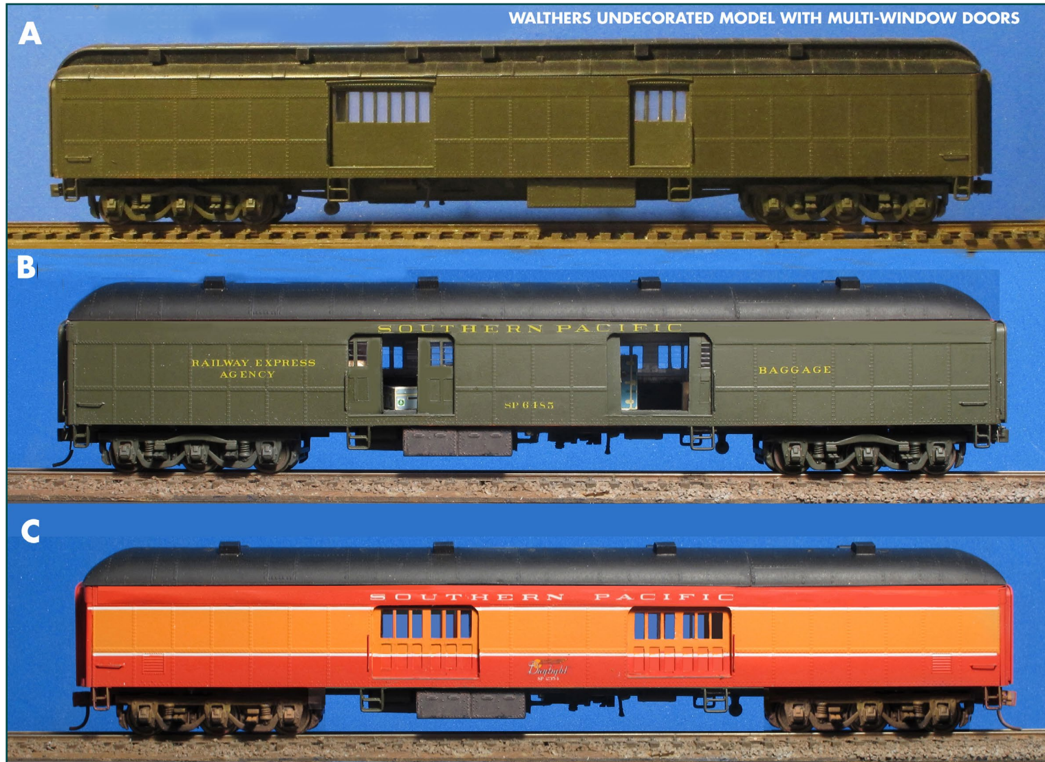
2. Walthers ACF Missouri Pacific Baggage Express car (932-10500) in panel A. Panel B shows my conversion to an SP 70-B car. Panel C shows a conversion in Daylight colors. Fortunately, detailed resin kits of this car are available from Southern Car and Foundry.
