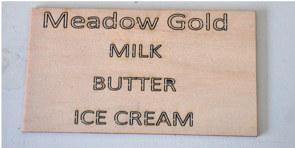
37. Lettering for the big display signs was custom-cut by Brian Banna using a laser cutter.
