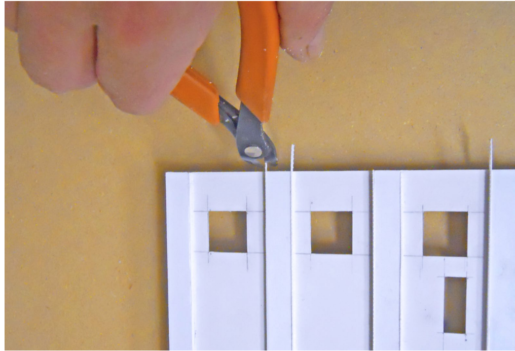
13. I began by adding the 12" wide vertical pieces of brick to the inside of the pilasters. I cut the pieces long, and trimmed them to fit.
