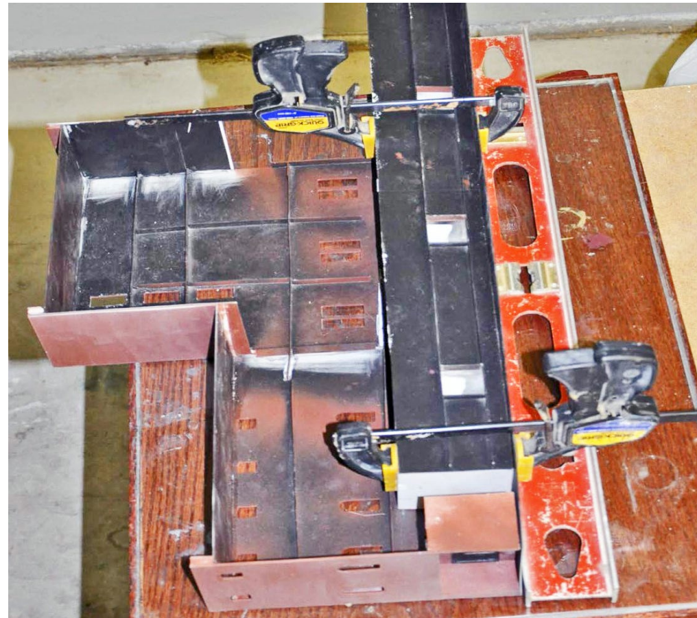
27. The rail dock sub-section is being mated with the right wing and center section. To ensure a good joint I used a 2' steel level and some of my woodworking clamps to align the pieces and hold them in place until the glue had dried overnight.
