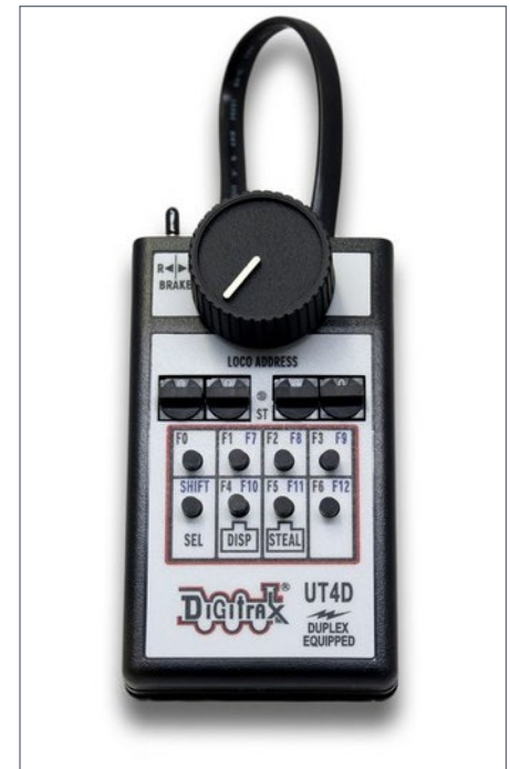
1. Digitrax UT4D (duplex radio) potentiometer style throttle – direction selector switch is on the top left, here in the center-off (brake) position.
