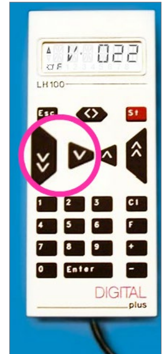
3. Lenz LH100 button control throttle – the down speed controls are circled, the up speed controls are the buttons on the right.
