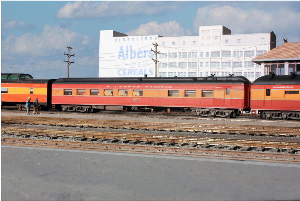
9. Model of a clerestory roof SP dining car (77-D-9) aisle side.
