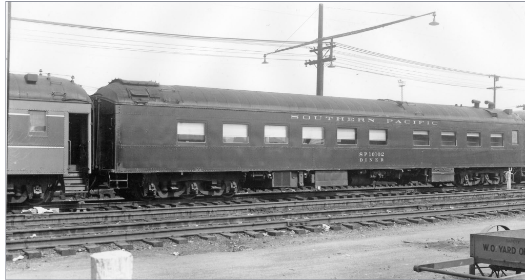
10. Prototype SP diner Class 77-D-3 10102, aisle side. Courtesy Bob's Photos
