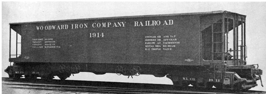
12. 100-ton cars built for Woodward by Pressed Steel Car Company in the late 1920s. John Stewart Collection
