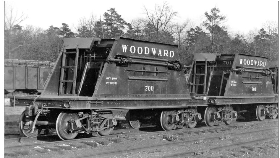
13. Home-built 20-ton ore cars used at the short-lived Vance Mine in Franklin County, near Russellville, AL. John Stewart Collection
