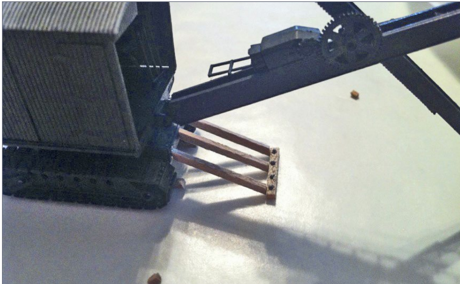
16. The bracing in the front of the steam shovel.
