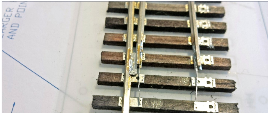
35. The hinge block is soldered in place. It is important to make sure it's sitting on the top of the rail base.
