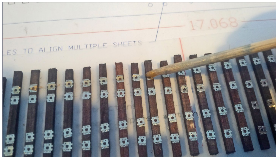
25. Pliobond is added applied to the tie plates. Be careful of the strings created by the Pliobond and remove them.
