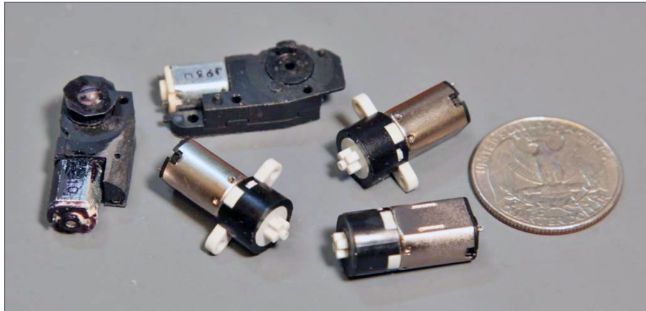
38. The planetary-gear drive motors for crane 19. The quarter gives you a good idea of how small these motors are.
