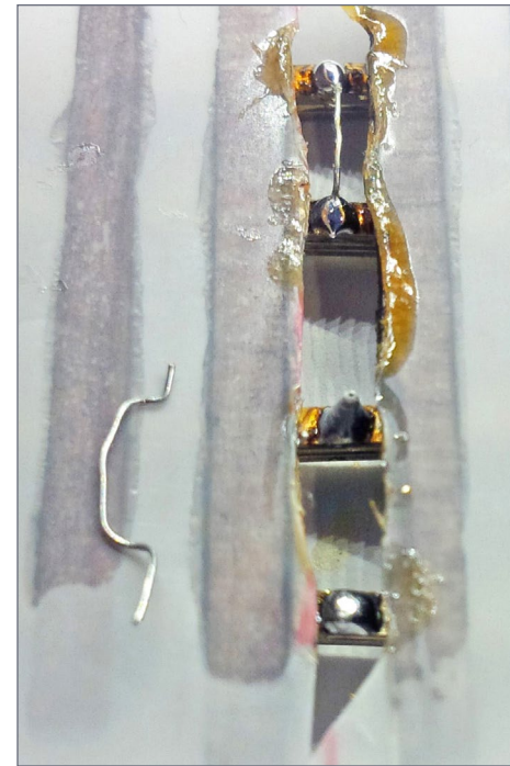
42. I turned the assembly over, cut away some of the plastic sheet and soldered on jumper wires between the stock rail and the closure rail on both sides of the turnout.
