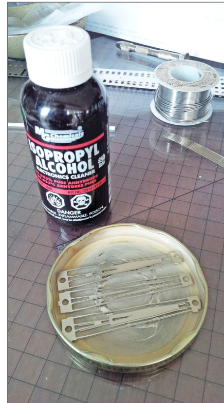
15. Clean the parts of the frog using 99% isopropyl alcohol and a paper towel and set them aside.
