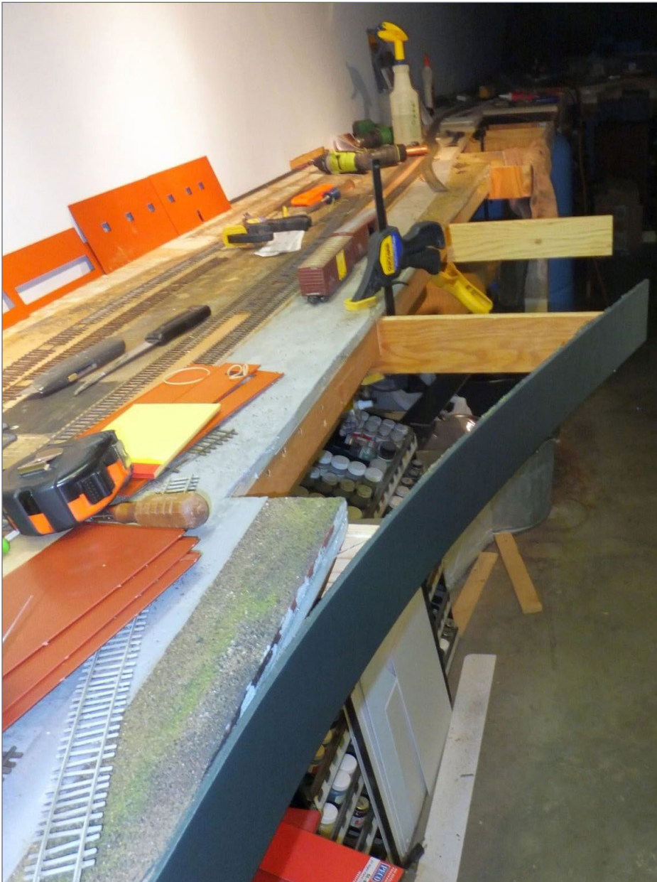
46. The existing fascia is curved out to accommodate the bump-out, and it defines the areas to be filled.
