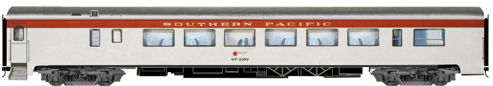
83-C-5 CAR AS REPAINTED AFTER 1958 WITH IMITATION STAINLESS WITH RED STRIPE. CARS RECEIVED NEW ALUMINUM FIXED STEPS AND THE BAGGAGE ELEVATORS WERE REMOVED.
