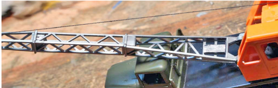
33. Weights have been added to the boom to help stabilize it.
