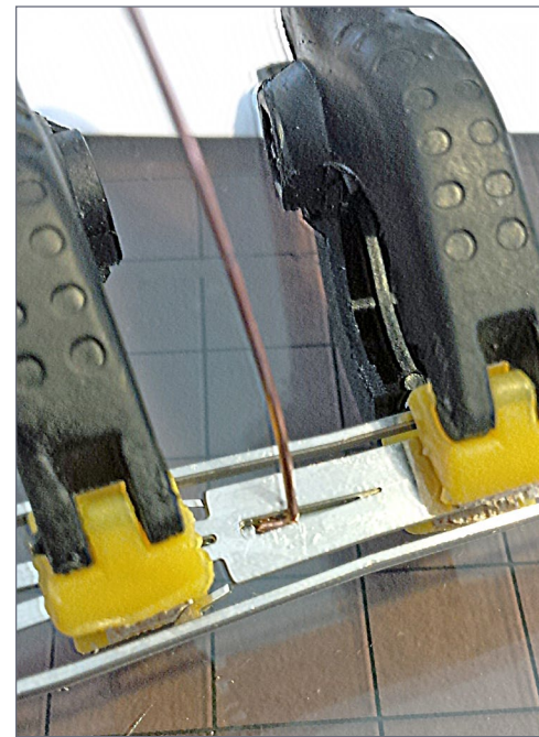
18. Test-fitting the feeder wire on the frog.
