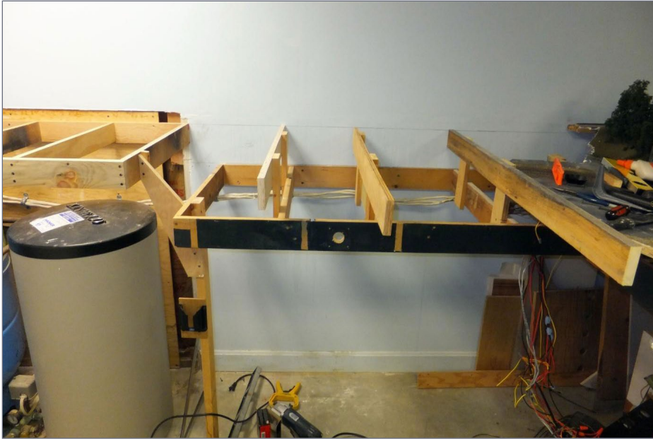
13. The former South Towanda needed to be raised. The old benchwork ran off to the right and under completed layout areas, so it was easier to leave it in place and extend new risers and joists to support the new Tunkhannock.
