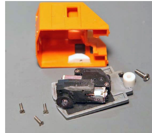
27. The motor drives have been mounted on cab floor.
