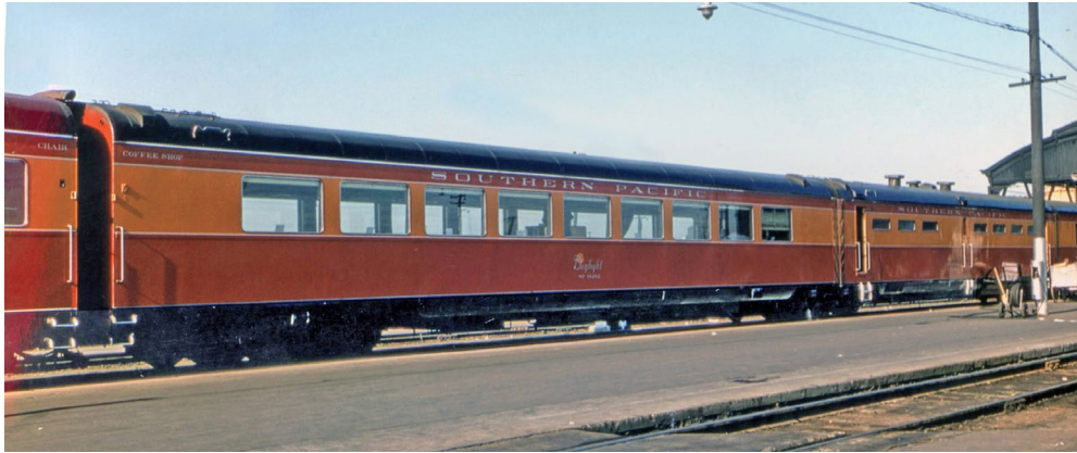
13. The coffee shop portion of a Shasta Daylight triple car food service unit illustrating windows that are 1/3 taller than most lightweight car windows. Postwar SP lightweight cars were recognized by these extra tall windows. Courtesy Bob's Photos
