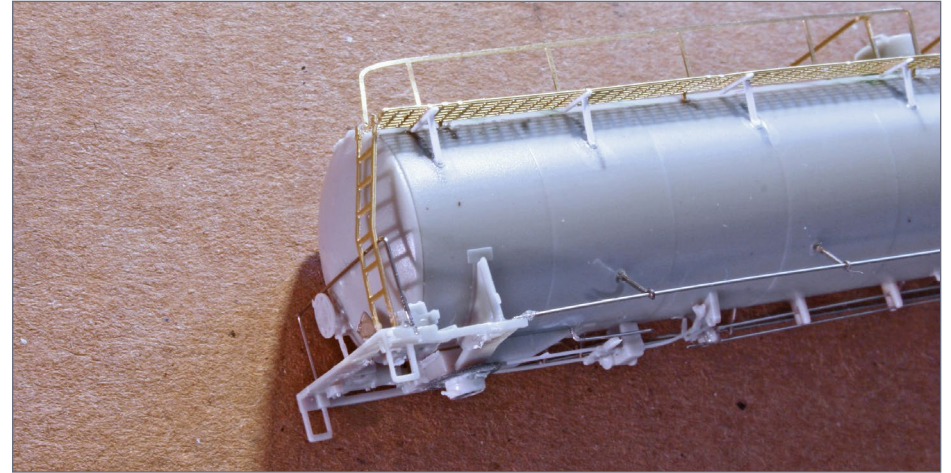
11. Bracing to support the catwalk is made from .010" x .020" styrene. The braces are then cemented into place. In this photo you can also see the end handrail I made from 0.012" stainless steel wire.
