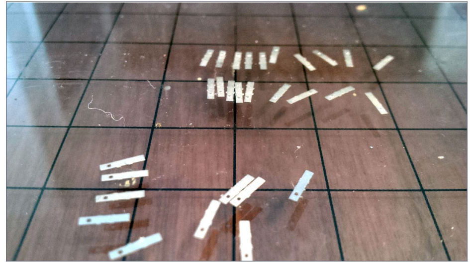
29. The frog tie plates have been cut out and readied for installing.
