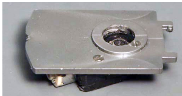
23. Cab turntable drive viewed from the bottom.
