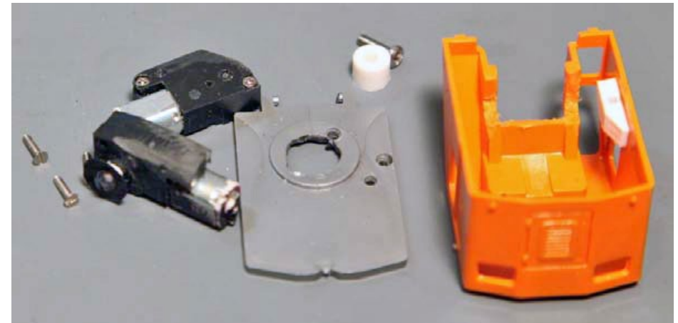
17. Parts for the cab-turntable drive and mounts.
