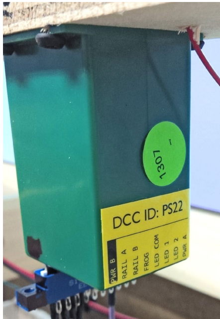
52, 53. I apply a label on the Tortoise marking the purpose of each connection and then duplicate the labeling at the terminal strip.
