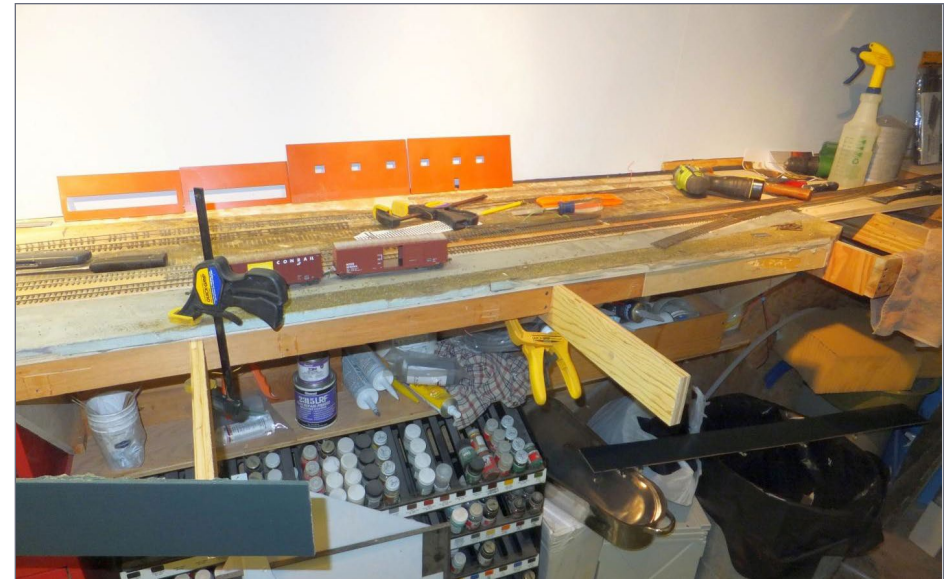
45. One of the attractive things about the Ransom plant was that it was on both sides of the main line, with the buildings connected by an overhead pipe bridge. The pulp or stock prep portion of the plant was to be closest to the aisle. I needed a bump out to permit this. Benchwork joists are being extended to the proper length for support.
