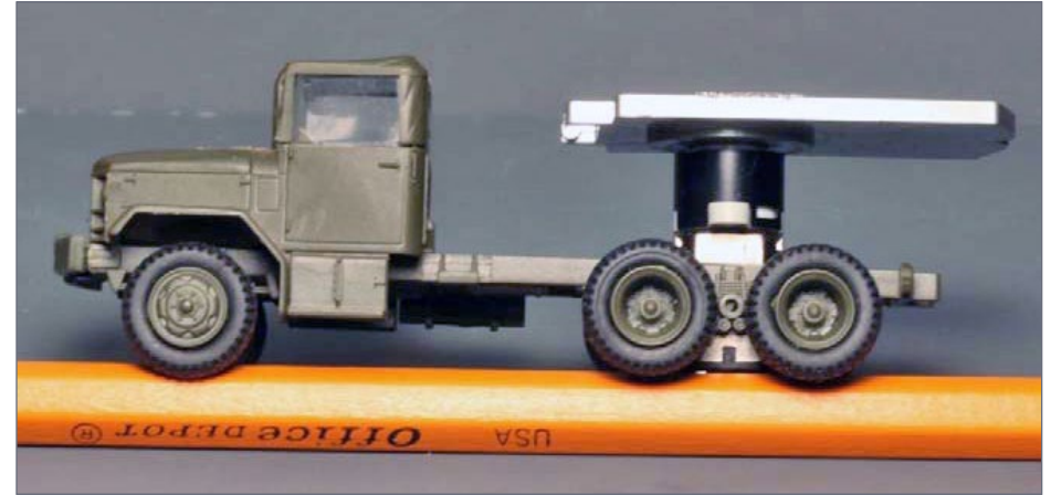
39. Crane 19 with the turntable motor mounted between the axles.
