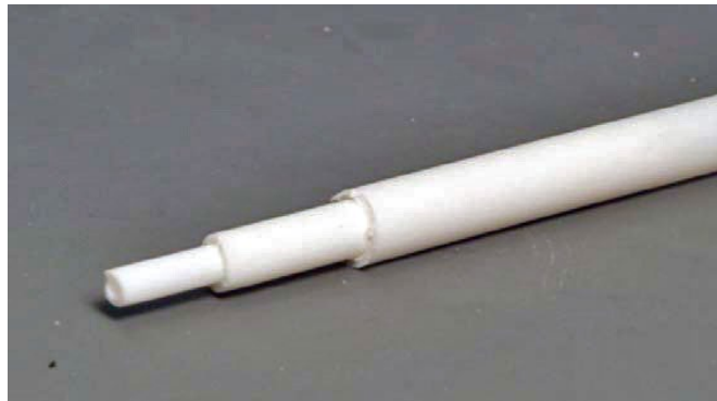
18. Forming the drive hub from tube styrene.
