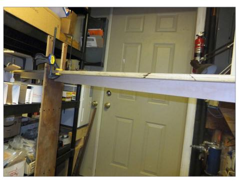
35. The latch is a simple barrel-bolt type. I wasn't certain this would be sufficient and was prepared to have one on each side of the bridge, but the single catch proved to be very solid. Note how the swing-down bridge also has a supporting "T" member for no-sag performance over time.
