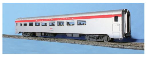
2. Former Daylight parlor car as rebuilt to chair car 2243 with flat stainless sides, vestibule end.
