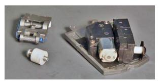
24. Cab turntable and cable drum motors.
