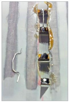
42. I turned the assembly over, cut away some of the plastic sheet and soldered on jumper wires between the stock rail and the closure rail on both sides of the turnout.
