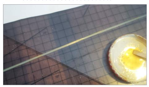
24. Pilobond has been applied to the bottom of the rail. The rail needs to be set aside till the glue becomes tacky.
