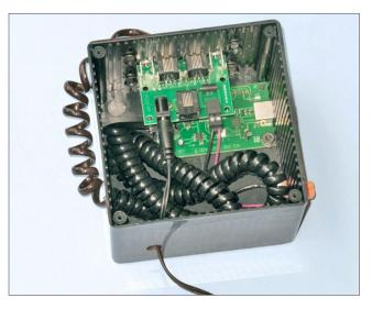
7. I passed the power cable from the "wall wart" for the throttle socket board through a hole I drilled in the case and plugged it in.
