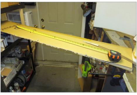
22. The footprint and shape of the actual bridge could not be totally straight and had to accommodate the curve coming off the existing benchwork. I chose cardboard to create a template for the needed plywood.
