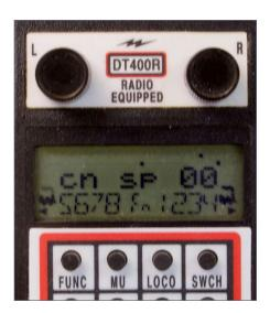
3. UniVersal consisting on a Digitrax DT400R throttle -1234 is in the lead and 5678 is in the rear, with locos facing away from each other. Yes, they read from right to left. The right button is the "master" and that's where the consist starts. This screen shot is what it looks like after pressing the MU button and then the + button.
