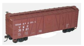
Three different styles of boxcar have also been released including a T&P single-sheathed car with outside bracing. The wood car has Murphy steel ends and Youngstown corrugated steel doors.
