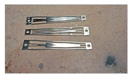
13. Here are the three parts of the frog, separated and ready to be stacked.
