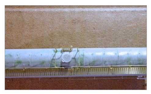
8. The dome hand railings mounted to the top of the car.
