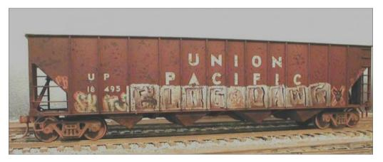
1. Here is lettering faded with an airbrush. For chipped and rusted lettering, sand the letters first or add rust colored spots during the weathering, as on this Union Pacific hopper. *Dave Branum photo*
