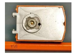
40. Crane 19 hub glued to the cab floor.
