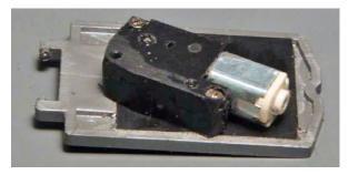
22. Cab-turntable drive motor mounted.
