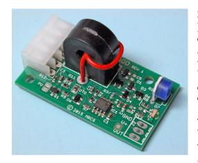
indicating a track/block has current flowing in it. The occupancy signal is logic low and can be tied to a computer input port or current limited LED. The unit draws 5mA @ 5V and supports up to 60A of track current. It is available with either a 3-position screw terminal block or
