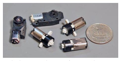
38. The planetary-gear drive motors for crane 19. The quarter gives you a good idea of how small these motors are.
