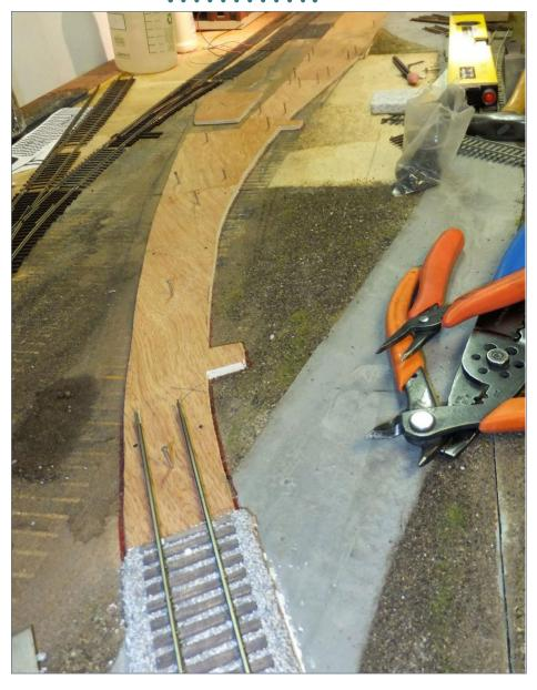
41. Once I was sure of my track locations I slipped a sheet of 1/4" lauan plywood under the tracks, traced their locations, and cut away the unwanted material to make roadbed.
