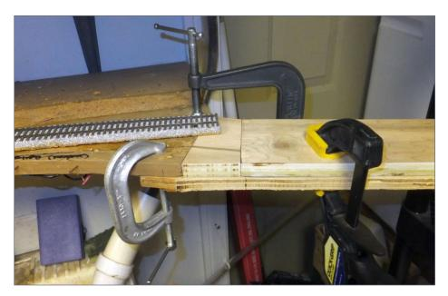
27. The splice plate and filler are ready to be screwed in place outside of Pittston staging.
