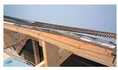
47. Caulk was applied to the cork roadbed under the turnout and the turnout set in place.
