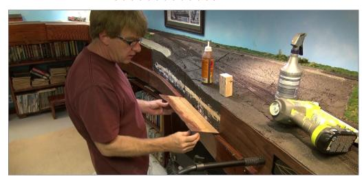
35. Quarter-inch oak plywood cut to shape and stained with red oak stain covers the sides. It is finished with three coats of polyurethane varnish, sanded between coats with 1500 grit wet sandpaper.
