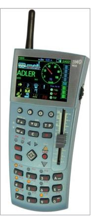
The older system (MX1 box with MX31 [11] throttle) automates universal consisting. The key with the label T P on it is used to add the active loco to the consist or to remove it from the consist.
