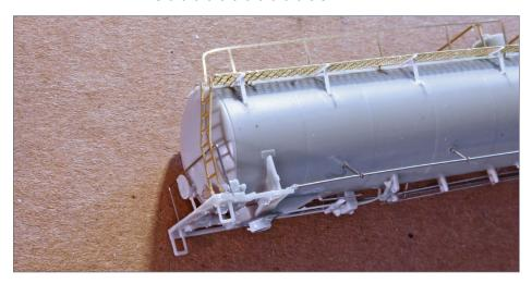
11. Bracing to support the catwalk is made from .010" x .020" styrene. The braces are then cemented into place. In this photo you can also see the end handrail I made from 0.012" stainless steel wire.
