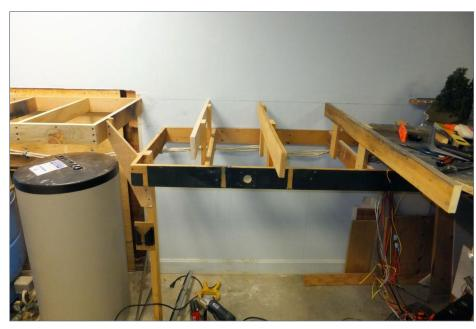
13. The former South Towanda needed to be raised. The old benchwork ran off to the right and under completed layout areas, so it was easier to leave it in place and extend new risers and joists to support the new Tunkhannock.
