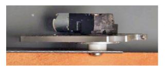
25. Crane cab turntable drive bushing test. I checked the hole to make sure it was centered and perpendicular to the drive.
