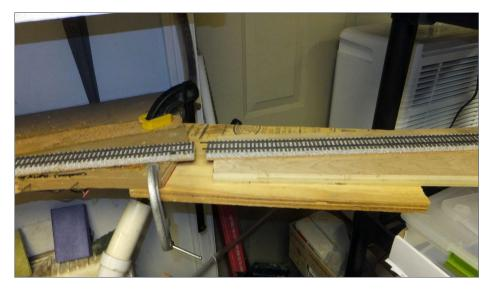
23. From staging, I needed a new alignment. The plywood that's clamped here will become the splice plate, and I'm moving some new 3/4" birch ply in from the right to get to the bridge location. Once that is in place, I'll clamp it, trace it onto the splice plate, and then remove excess material.
