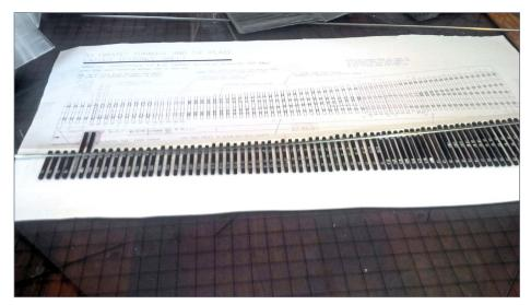
23. Test fit the rail on the tie plates to make sure that it will sit properly. By carefully using the templates the rails fit perfectly.
