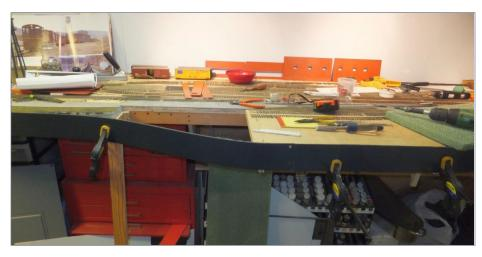
48. With the fascia clamped to the new bump-out, foam can be traced to fill in on either side of the plywood that supports the building and tracks.
