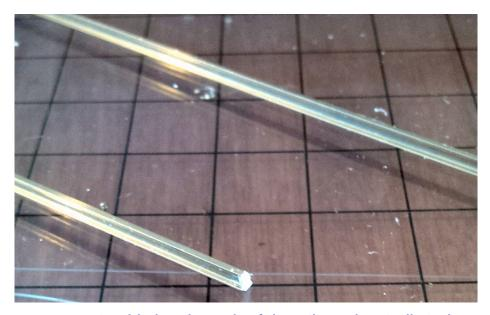
30. Styrene is added to the ends of the rails to electrically isolate the frog from the closure rails.
