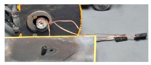
26. A shot of the crane cab bushing through crane bottom.
