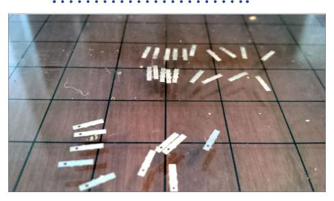
29. The frog tie plates have been cut out and readied for installing.
