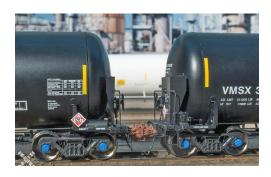
Both versions of the ready-torun model come with metal SE Type safety double-shelf knuckle couplers (above), and ASF motion-control 110-ton trucks with 36-inch wheelsets with rotating bearing caps. The Operator series model
