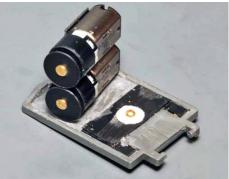
45-46. Stacked hoist drives on the cab floor.
