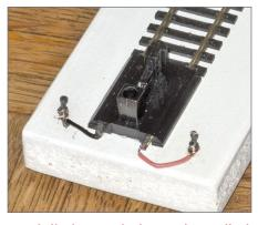
4. I drilled some holes and installed a couple of nails, then soldered wire to them to allow easily attaching feeder leads to the track.
