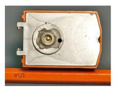
40. Crane 19 hub glued to the cab floor.
