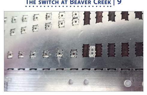
8. Here's a guard rail tie plate as it comes in the kit. Note the hole is bigger for the wider flange ways that HO requires instead of the Proto:87.
