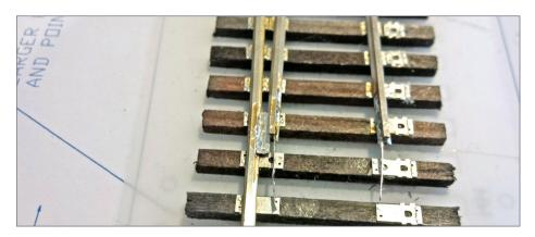
35. The hinge block is soldered in place. It is important to make sure it's sitting on the top of the rail base.
