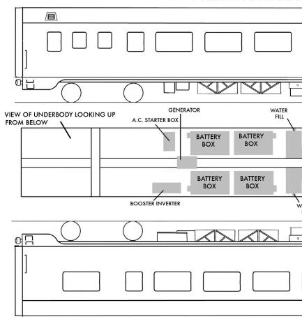
12. Drawing of 83-C-5 chair car showing arrangement of the Pullman electromechanical air conditioning unit on these cars. Class 83-C-5 was built of welded steel construction in 1954. The configuration was the same as one of the earlier class 83-C-1 chair cars built for the Shasta Daylight, which were built of riveted aluminum. Both classes has extra tall
