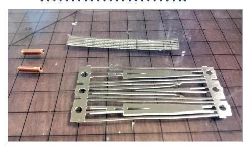
12. Here are the parts needed to build the frog: 1/8" copper tubing, the bolt detail bars, and the frog itself.
