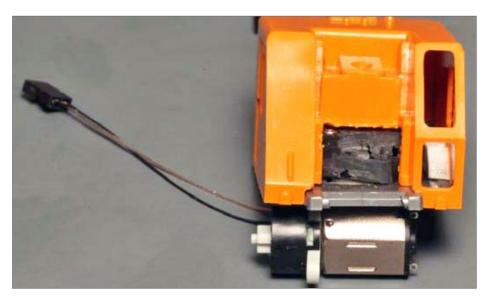
49. Wire lead extended for the DCC decoder.
