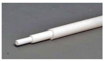
18. Forming the drive hub from tube styrene.
