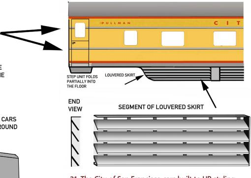
21. The City of San Francisco cars built to UP styling standards for Overland service were fitted with aluminum strips above and below the window pier panel. Most of these cars had louvered skirts built as shown.
