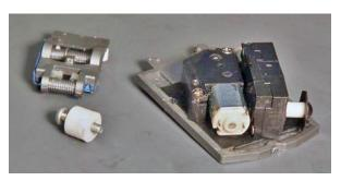
24. Cab turntable and cable drum motors.
