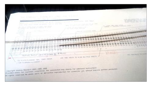
22. The template is used to mark the bends in the rail of the diverging route.
