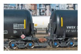
Both versions of the ready-torun model come with metal SE Type safety double-shelf knuckle couplers (above), and ASF motion-control 110-ton trucks with 36-inch wheelsets with rotating bearing caps. The Operator series model
