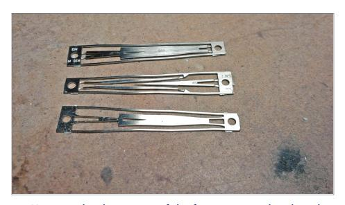
13. Here are the three parts of the frog, separated and ready to be stacked.
