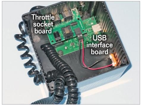
5. I mounted the NCE throttle socket board and USB interface board into a plastic electrical project box to keep things all neat and tidy.
