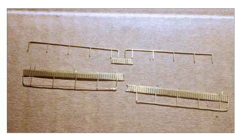
5. This picture shows the cuts made for the outside-railing on the UTLX car.
