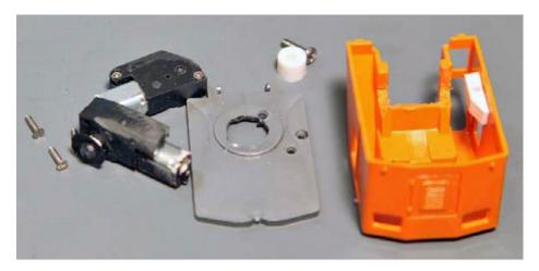
17. Parts for the cab-turntable drive and mounts.
