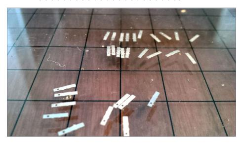
29. The frog tie plates have been cut out and readied for installing.
