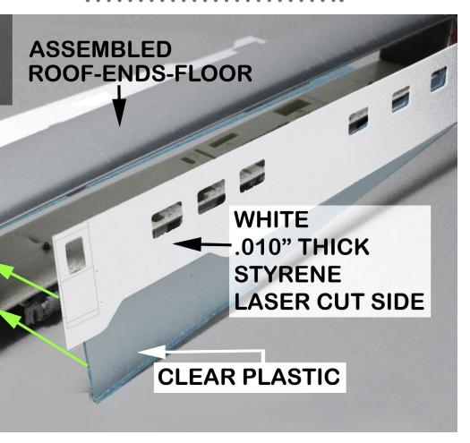
18. Assembly of a car core kit.
