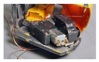
28. Cab turntable drive motor (left) and hoist motor (right).
