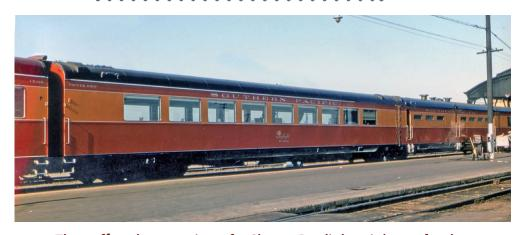
13. The coffee shop portion of a Shasta Daylight triple car food service unit illustrating windows that are 1/3 taller than most light-weight car windows. Postwar SP lightweight cars were recognized by these extra tall windows. *Courtesy Bob's Photos*
