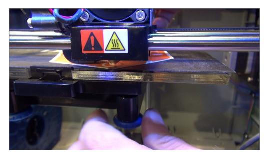
28. One of the first steps in setting up is to level the printer table to the head position in three locations, using a gap tool supplied in the package.
