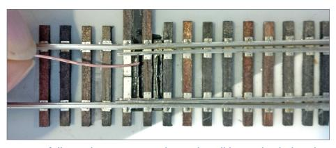
40. Carefully apply some CA to the push/pull bars. Check that the points still move after adding the .020" x .030" styrene.
