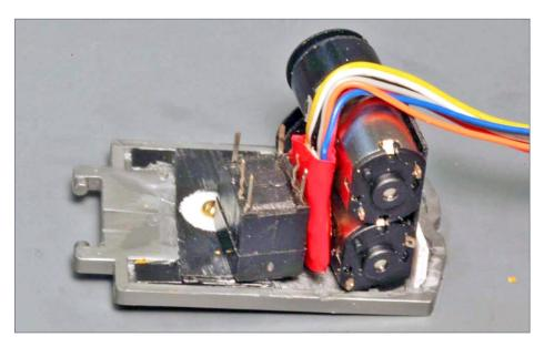
47. An SPDT relay and DZ126 decoder are installed on the cab floor next to the stacked drum drives.
