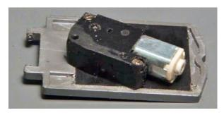
22. Cab-turntable drive motor mounted.
