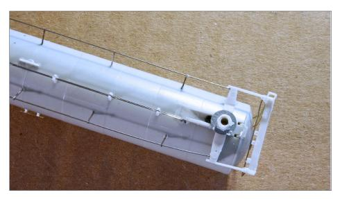
2. I add a Kadee fiber washer to my standard Micro Trains car. I attach it to the bolster pegs. You can also see my putty mix applied to the bolster pin to bring it up to the same diameter as the Micro-Trains trucks.
