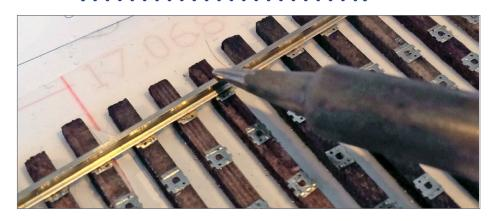
26. A soldering iron is used to heat the rails and set the Pliobond.
