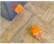
10. The track feeders with the alligator clips plug into the box here. The alligator clips on the other end connect to the test track as shown in [1].
