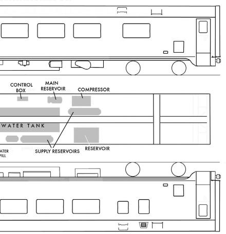
windows. Union Station Products kit #7571A for the 83-C-1 class car can be used to simlate the 83-C-5. (NOTE: There were other window and seating arrangements of the 83-C-1 cars for the Shasta Daylight, all classed 83-C-1.)
