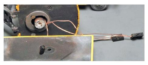
26. A shot of the crane cab bushing through crane bottom.
