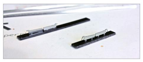
34. Here are the completed push (rear) and pull (front) bars.
