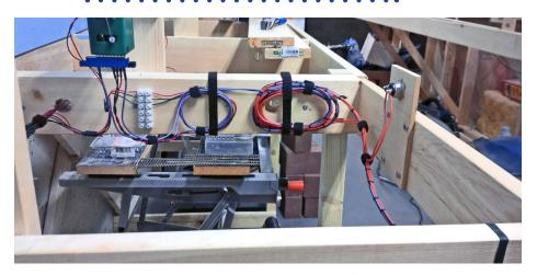
52. The Tortoise is wired and the push button for control is on the right. You can see the loops of wire that I added to allow for future maintenance if needed.
