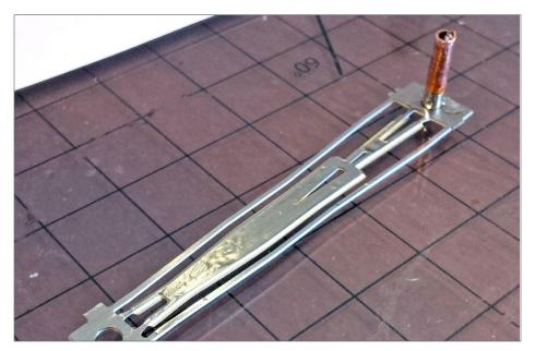
14. Test fit the copper alignment pin in each hole.
