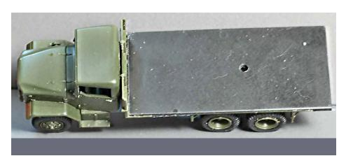
11. Flatbed extension with pivot hole drilled.
