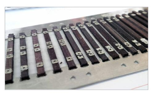
9. The installed guard rail tie plates on the ties.
