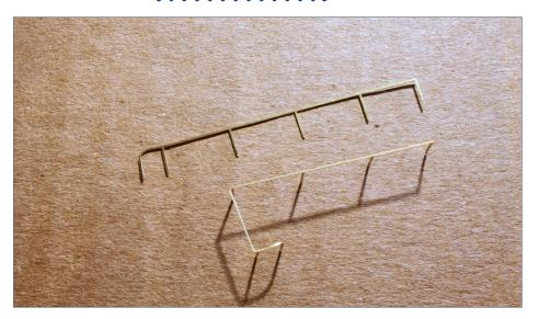
7. The dome railings are bent and trimmed for the inside railing.
