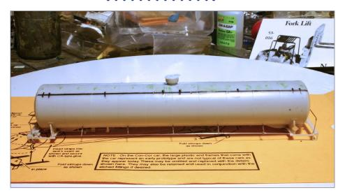
3. I marked the location of the walkway on the side of the tank body. For clarity in the photo, I used a marker instead of a pencil.
