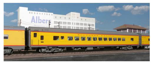
19. Walthers model of the 2215. Model features the tinted windows of the prototype. Minor detail variation is the notch over the truck which appeared only on the Union Pacific-owned cars.
