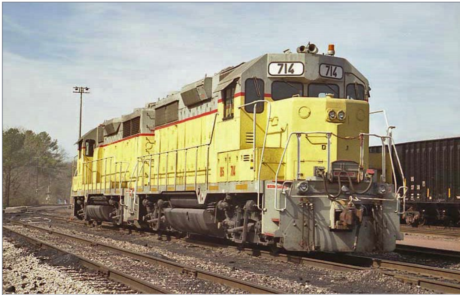
5. BSRR (Former Cedar Rapids & Iowa City Railway) GP38-2s 714 and 711 rebuilt from GP35s are sitting at Fairfield, AL awaiting their next assignment. William Davis photograph, posted at rrpicturesarchives.net
