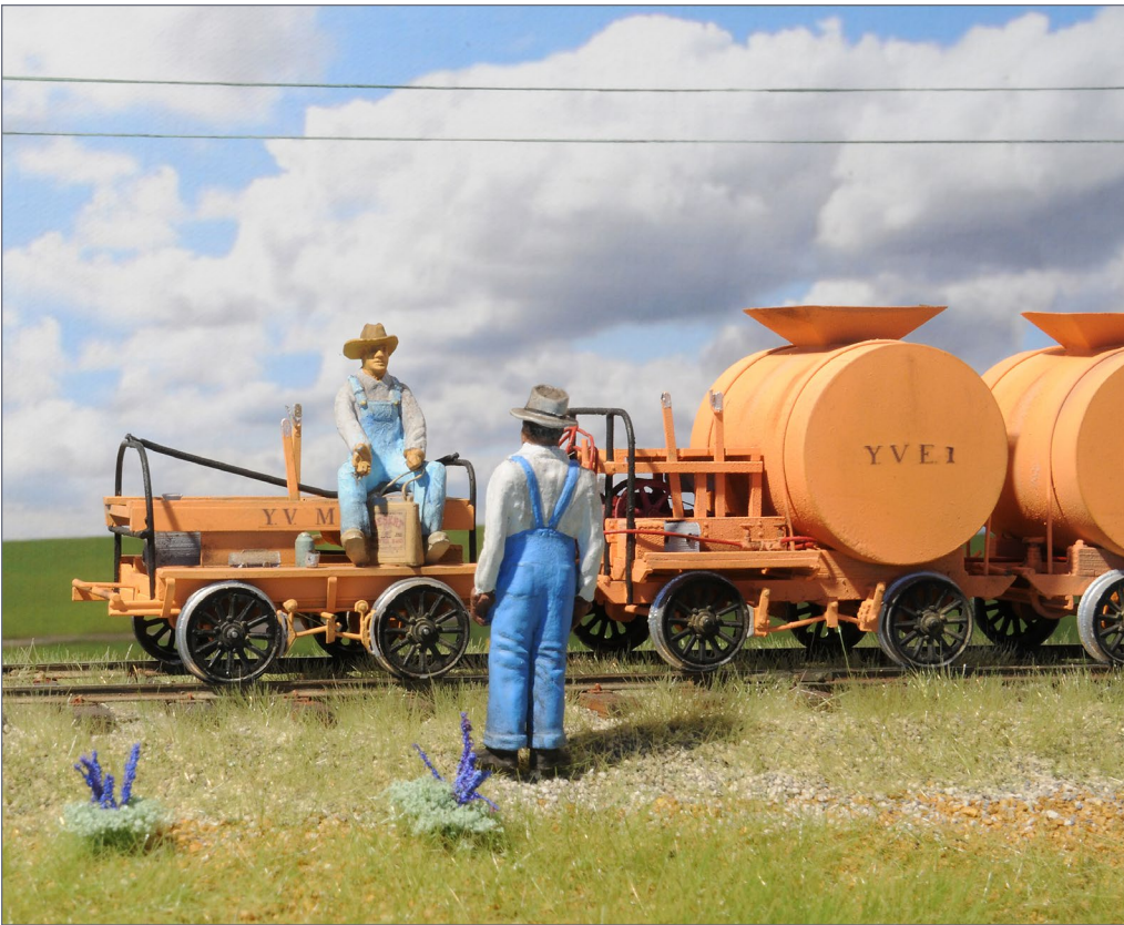
25. A closer view of the speeder and extinguisher car. The operator of the speeder is talking to one of the "hosemen" who ride on the extinguisher car or trailer, putting out fires from the weed burning operation. The wildflowers next to him are brush lupines.
