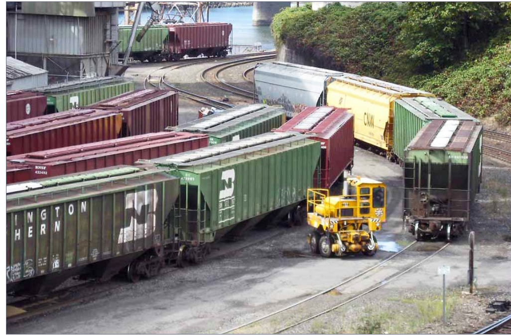
1. Hopper cars at a modern rail-to-water transfer are moved by a Trackmobile which can maneuver on and off the rails as needed. Graham Line photo
