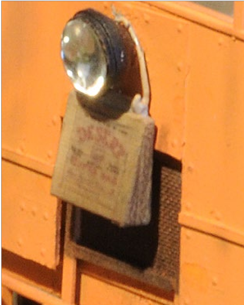
21. This Desert water bag measures about 1/4" square and is another detail made using rapid prototyping. Wire was added for the rope and the part painted before adding a decal made from a photo of a real Desert water bag found on the Internet.
