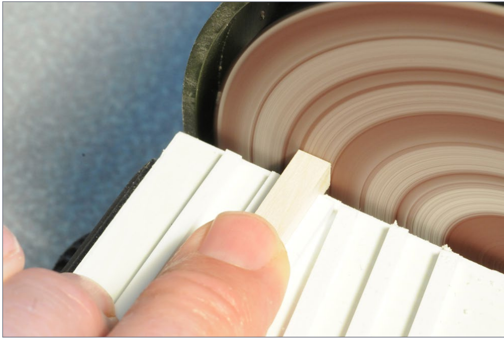
10. One end of each of the posts for one bent are first sanded square or angled.
