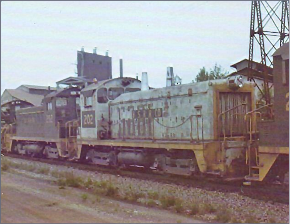
10. BSRR 202 SW7 still in Woodward Iron colors. Formerly WIRR 50, in 1974 rebuilt by EMD and renumbered 302. Glenn Marsh photo Hank Stephens collection Posted on rrpicturesarchives.net
