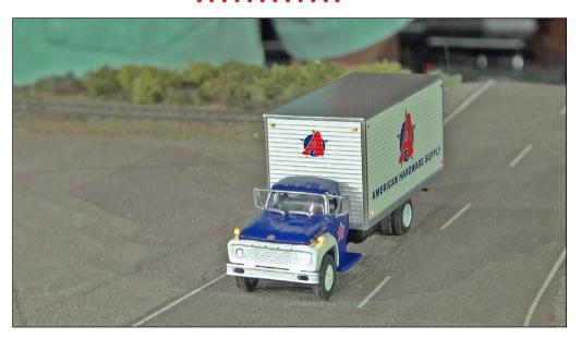
10. John installed a servo, a battery, receiver and gearbox to make this Athearn truck drive. He buys the parts he needs from a website in Germany, mikromodellbau.de. There you will also find videos showing how to install all the inner workings to make the models drive at scale speeds. I have watched some of the videos, and it seems to be relatively easy and straightforward.
