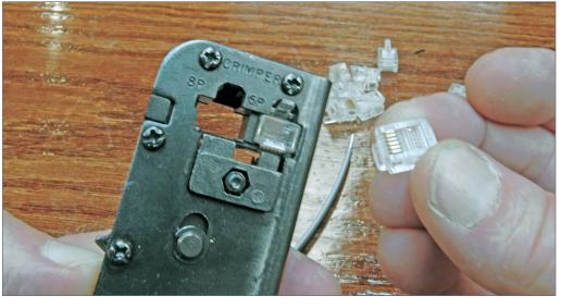
4. To use the crimper tool, first place a six-conductor plastic phone jack in to the tool's six-wire slot as seen in this photo.
