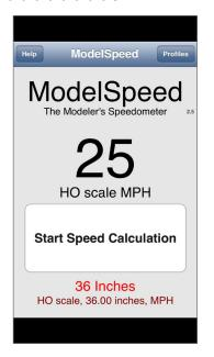
5. ModelSpeed app to calculate scale speed through a set distance by measuring the elapsed time. Costs 99¢.
