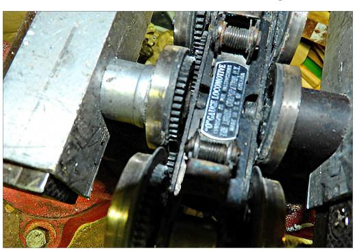
5. Old speaker magnets hold wheels in place and protect metal castings. *Murray Miller photo*
