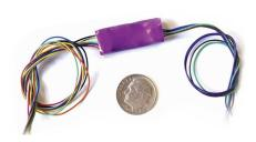
**SoundTraxx** has introduced a new generation of digital sound decoders. Identified as the TSU-1100, the new decoders measure 27mm x 10.5mm x 5mm. They are intended primarily for HO and N scale locomotives.
