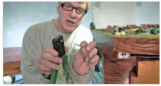
5. Then, with the insulation stripped about 3/16ths of an inch, place this wire into the plastic jack in the crimper's slot.
