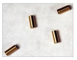
4. Machined adapter bushings allow old flywheels to be mounted on more modern can motors, and other solutions are possible. A-Line/ Proto Power West photo
