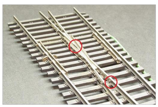
1. The rail just before the frog has a bracket that would seem to catch on a wheel's flange (see lower circle on picture). Another concern is the depth of the flangeway at the frog (upper circle).
