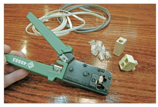
3. A crimper tool is necessary to clamp on six-conductor phone jacks to the wire to daisy chain the Digitrax loco net panels around the layout room. The crimper tool will also work with eight-wire phone accessories as well, essential if you use NCE's DCC system with its eight-wire system. I also like the line splitters and straight connectors seen in this photo. All are simple plug and go parts.
