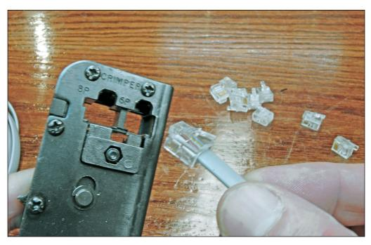
6. Squeeze the tool's handle to clamp the phone jack to the six-wire cable. Pull it out and you have a complete and professional jack connected permanently to the six wires.
