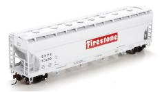
Also just released is a Roundhouse ACF 5250 cu. ft. four-bay covered hopper car. In addition to the SHPX-Firestone scheme shown here, the HO scale ready-to-run model comes decorated for
