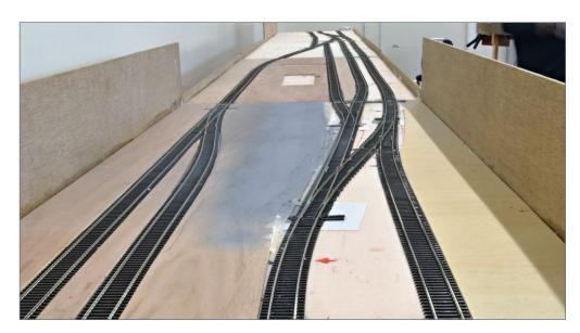
13. 3mm ply was used to raise the surrounding land to nearly track level on much of the layout.
