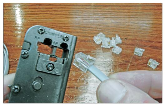
6. Squeeze the tool's handle to clamp the phone jack to the six-wire cable. Pull it out and you have a complete and professional jack connected permanently to the six wires.
