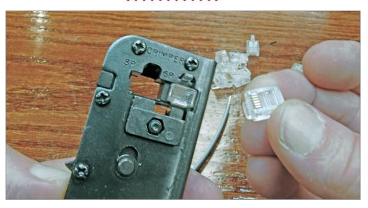
4. To use the crimper tool, first place a six-conductor plastic phone jack in to the tool's six-wire slot as seen in this photo.
