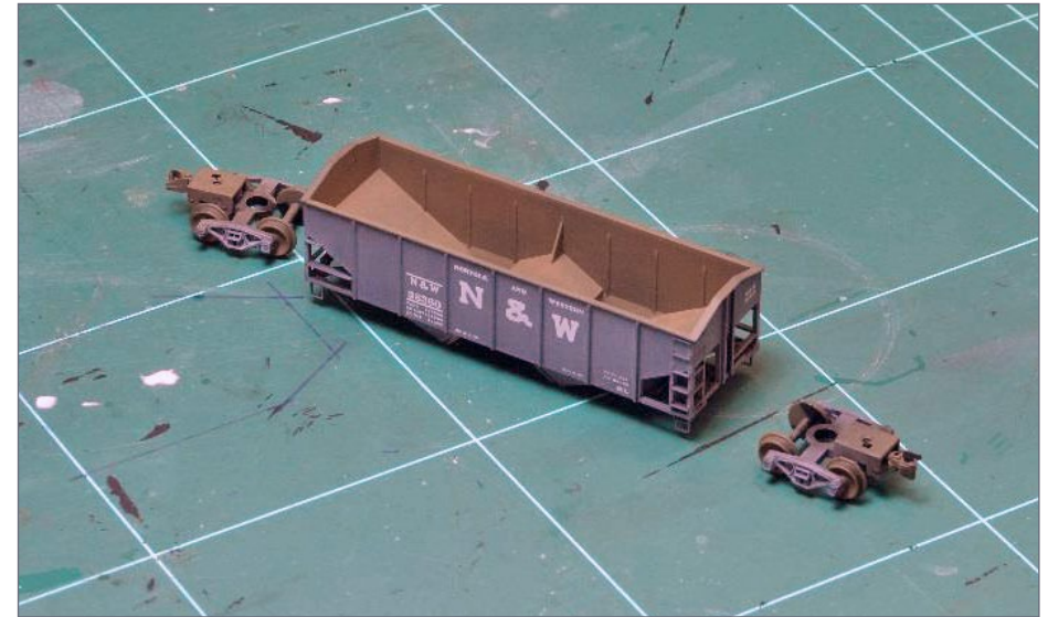
16. With all parts airbrushed I reassemble the trucks. They are also airbrushed with dark gray paint. The overall lighter colors will be toned-down with powders in the next step.
