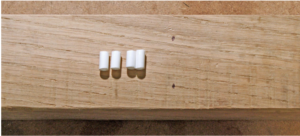
3. I use mostly QSI Titan decoders for my large scale engines. I marked the decoder mounting slots and cut styrene tubing to 3/8" length for elevating the decoder.
