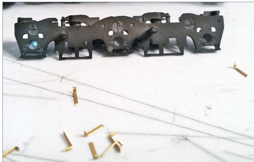
1. The formed brass flat stock pieces ready to add to the side frame.
