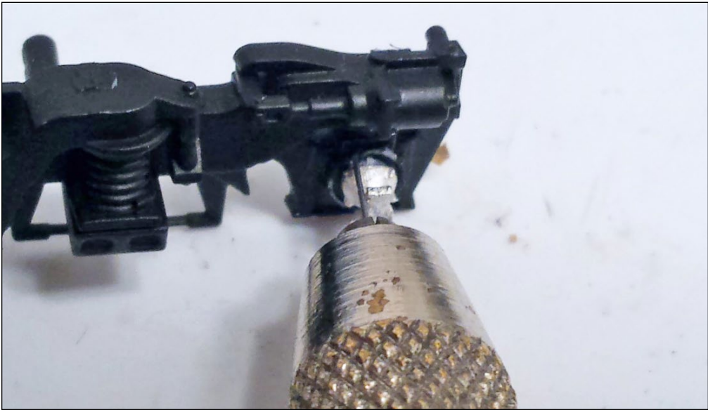
4. A #79 hole is being drilled just to the left of the wheel-slip indicator to allow installation of the 0.010" cable.
