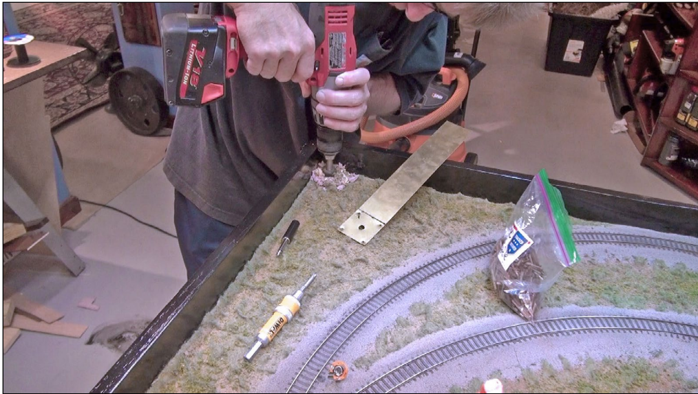
12. I drilled a hole in the corner of the layout to pass the wires from the mounting jack to the surface of the layout.
