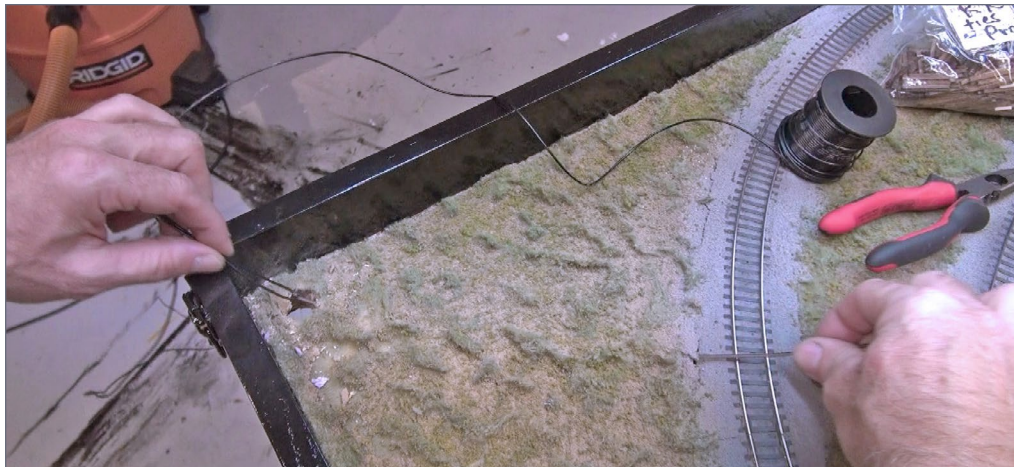
13. I then snaked the power feed wires from the corner of the layout under the fake fur to the track, using a piece of bent code 70 rail as a wire snake.
