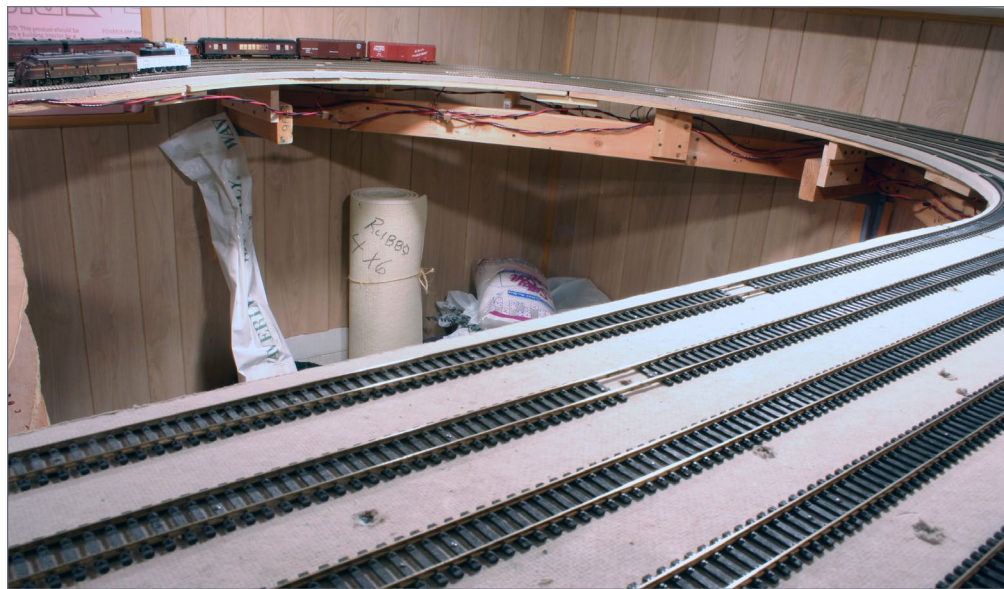
28. Andy Rubbo’s helix stretches from wall to wall in a seven foot wide room. The outer two tracks are the ascending (westbound) grade. With an outer curve radius of slightly more than 40 inches, the grade figures out at roughly 1.5 percent.
