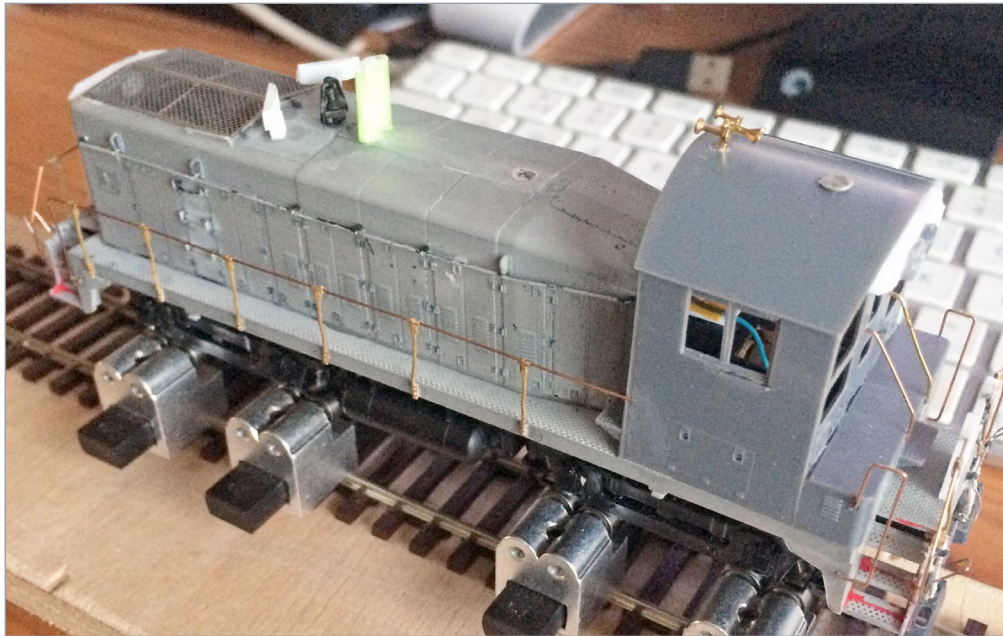
11. Koos used Smokey Valley handrail stanchions and brass wire for the handrails on this loco.
