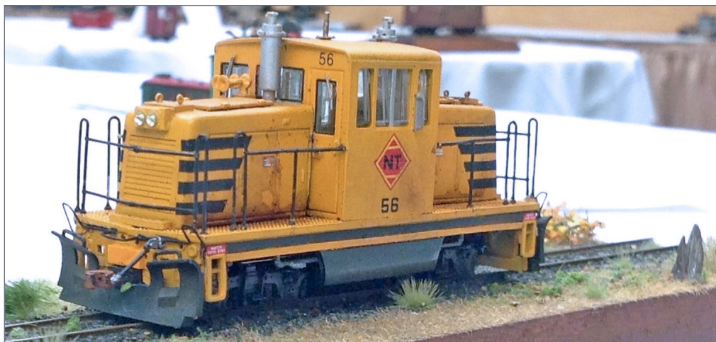
17. Ted Alexander kitbashed a 45-ton body to HOn3 by narrowing the walkway and cab. He then mounted it to an Atlas N scale drive.
