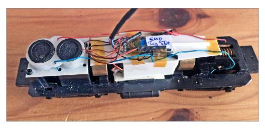
15. Here is what the sound install looks like inside this loco. By going to a much smaller Mashima motor [14], Koos got enough extra space to easily fit sound into this loco.
