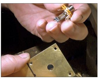
11. Using a thin piece of brass stock, I made a face plate to hold a guitar jack mount. The jack allows the layout to have power when
