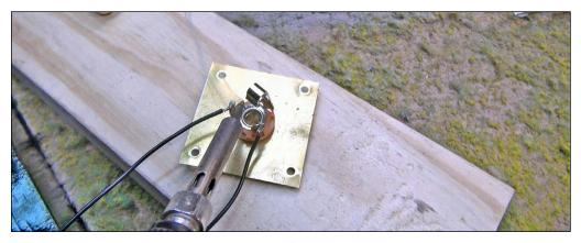
14. Power wires soldered to the female microphone jack connect to the outside of the rails on the Bachmann EZ Track. Note how I use clamping tweezers to hold the wire in place on the rails during soldering.
