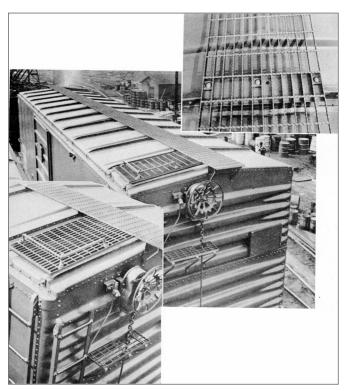
they used a spiral rod to hold the serrated metal strips in position [36]. The Kerrigan, Blaw-Knox and Tri-Lok running boards were all composed of 12 rows of edge-mounted serrated steel. It is difficult to distinguish among the three.
