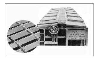
32. Apex Tri-Lok metal running board.
