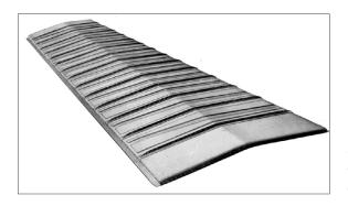
26. Stanray riveted diagonal panel roof circa 1970.
