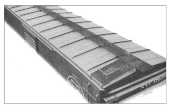
23. Pullman standard welded roof on a PS-1 boxcar.
