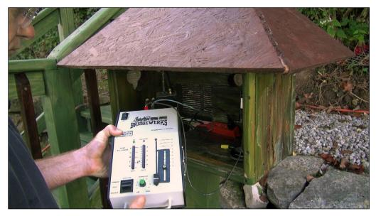
10. I chose to install a powerful Bridgewerks power supply with a radio control key fob-size hand-held throttle. With the built-in fan and 20 amps of power, this unit will have no problem handling three Aristo-Craft Dash 9 engines with 12 motors in the trucks drawing seven amps.
