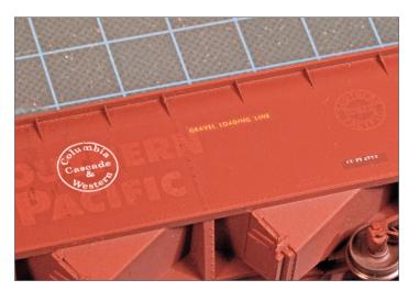
3. Rock is more dense than coal, so a smaller volume makes up a full load in a 70-ton car, and tops out several feet below the top chord. Cars assigned to aggregate loading are marked with a lettered notice or a 4-foot-long yellow line.
