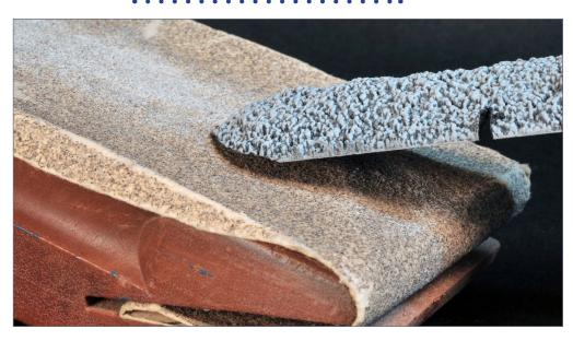
6. To make the load sit naturally in the car at the load line, taper the ends to match the angle of the slope sheets. A cutting tool with a disc, medium grit sandpaper, or a small belt sander will work. The precise modeler with a lot of loads to modify could build a jig and use a saw to cut or grind the angle.
