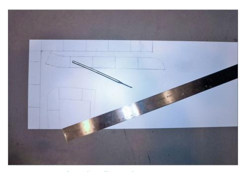
23. Laying out the sidewalks on sheet styrene.
