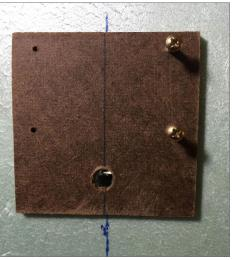
5-6. The needles must protrude through the bottom of the sub-roadbed. Place a small ruler against the needles under the layout and use a marker to draw the center line. Line up the mounting pad and hot-glue it in place.
