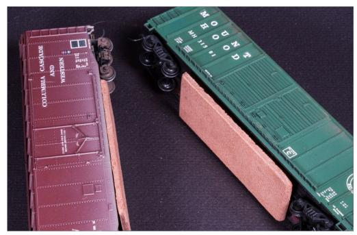
1. Masonite sliders do a good job of knocking dust and oxidation off railheads, but manual touch-up work is often needed on frogs, switch frogs, rerailers, and at grade crossings. *Joe Brugger photo*
