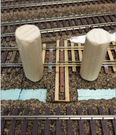
3-4. A pair of simple tools properly align a hardboard mounting pad under the nsulation foam layout. The tools are made by drilling a small hole in a pair of dowel rods and gluing a long needle in each. *Michael Anteau photos*
