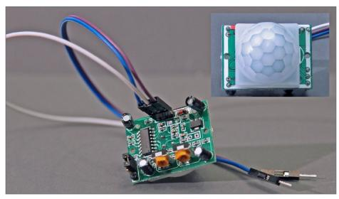
12. Here is a PIR sensor. Use the jumper on the lower left to set to retrigger each time, and adjust the yellow variable resistors to set the time delay and sensitivity.
