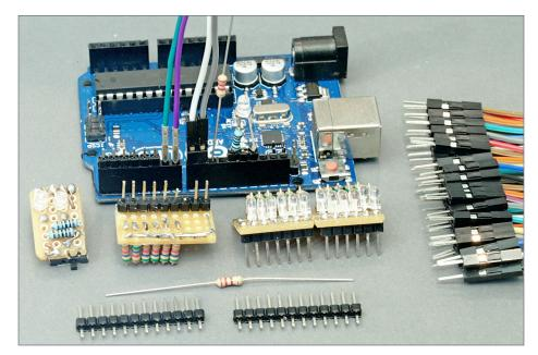
3. The larger Uno board has "header pin sockets" that easily allow plugging in wires and components like resistors to the board. Here I built some other plugable boards too using LEDs and resistors.
