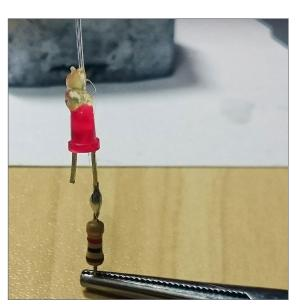
7. We will install two 2.8mm red LEDs, one in each cabin, to serve as the light sources. Solder a resistor to the positive pole of each LED to limit the inflow voltage. Cut two 100mm (about four inches) pieces of optical fiber and attach them to the LED housings with a drop of hot glue or superglue. Keep the soldering iron away from optical
