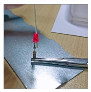
6. This procedure is very important and delicate. The ends of the optical fibers should touch the LED surface to ensure good uptake of light. Before gluing the fibers in place, do a couple of test fittings with a lighted LED to check the ideal position for bonding of fibers.
