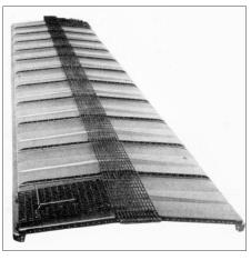
22. Pullman Standard riveted roof on a PS-1 boxcar.
