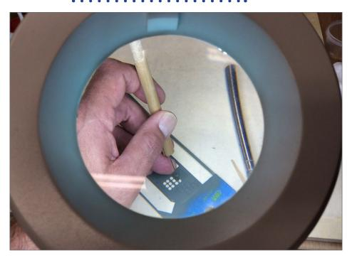
17. I use this tool a bunch – a needle glued into the end of a length of wooden round stock. The photo was taken looking through another essential tool, my illuminated magnifier.
