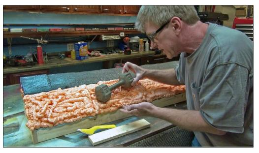
16. After the foam cured, I placed a 10-pound dumbbell to weight each section to see if it would hold up and could be used as a viable way to make scenery. All five sections held the weight without cracking.
