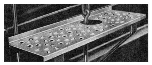
37. Stanray pressed steel brake step.
