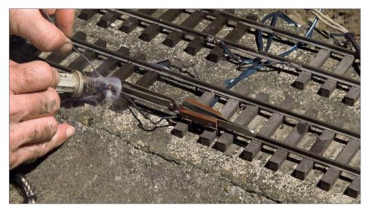
3. I added new power feed wires in eight spots on the 400-foot main line by using a resistance soldering rig to heat the large rail fast and minimize damage to the plastic ties.
