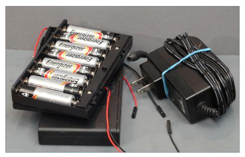
9. To source the power for your board, you can use either an eight AA battery pack (on left, 12V), or a 9V wall wart power adapter (on right) with an Arduino 5.5x2.5mm barrel plug.
