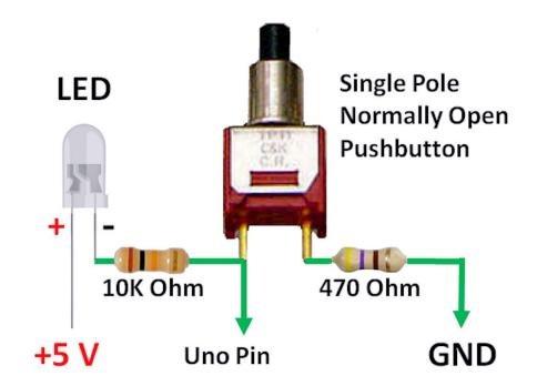
24. Push button and LED wiring diagram.
