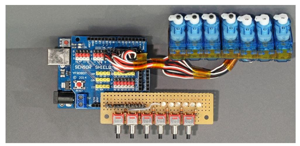
25. Servo setup 2, using an Uno and a Sensor Shield.
