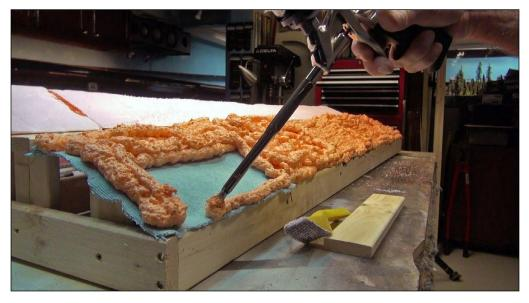
15. I covered the five sections with the Great Stuff foam and let this rise and cure for an hour. In the video, I set up a clock – more like a fan – so you can watch the foam rise in a timelapse video that plays for 20 seconds and covers one hour of real cure time.
