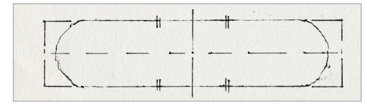
8. When the test load fits correctly and is easy to add and remove, trace a pattern on heavy paper to show the correct modified length. Because the load sits so deep in the car, matching the exact slope sheet angle isn't critical, but the curved ends should rest on the slope sheet. The end-to-end length of the car's interior is 40 feet, shown by the rectangular lines. The curved lines show the trimmed load, and the hash marks on the side are the positions of the internal braces.
