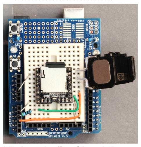
28. Sound setup 2, using an iPhone cell phone speaker. You can get an iPhone speaker for a few dollars on Amazon at this link: <a href="a.co/564x5AP">a.co/564x5AP</a>. Cut off the plastic housing extension and seal the small hole left with some epoxy or putty, leaving the rest of the speaker as shown here. These tiny speakers produce excellent sound.
