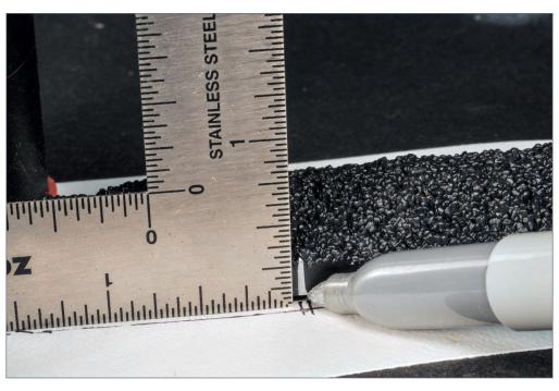
4. The loads must be trimmed to sit lower in the car. Locate the side brace positions and cut 1/8" deep slots into the side of the load. The slots will allow the dropped load to clear the car's internal bracing. Use a razor saw or cutting disc to reduce the depth of the loads sides to eliminate interference. Cut just below the top of the flat edge. Clean up the edge with sandpaper or a flat file.
