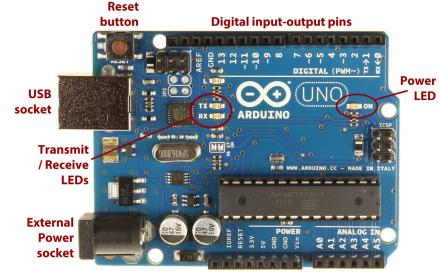
Power supply pins Analog input pins
