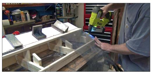
13. I started by stapling fiber window screen to a one-foot-wide segment of the hill. This screen will allow the foam to penetrate just a little, making for very strong foam hardshell scenery.
