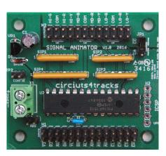
Circuits4Tracks has released a new product called the Signal Animator. It works in conjunction with their Quad Occupancy Detector. The product drives LEDs wired either common anode or cathode and implements speed restriction indications from switch machine inputs. It can be driven by an
