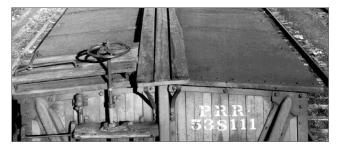
29. Wood running board, latitudinal, and brake step.
