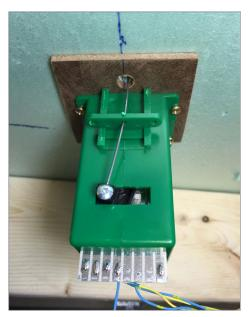
7. Pop the Tortoise in place, be sure the vertical throw bar goes through the switch rod hole, screw it down, and wire it up.
