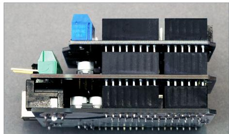
7. In this photo, you can see how the shield boards "stack" onto the Uno. In the top photo, I've aligned the pins, and in the bottom photo, I've pushed the boards all the way together. The Uno is on the bottom, the motor and sensor shields above.
