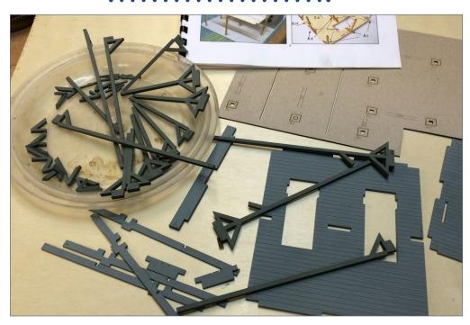
4. Paint all parts and panels with an airbrush before assembling
