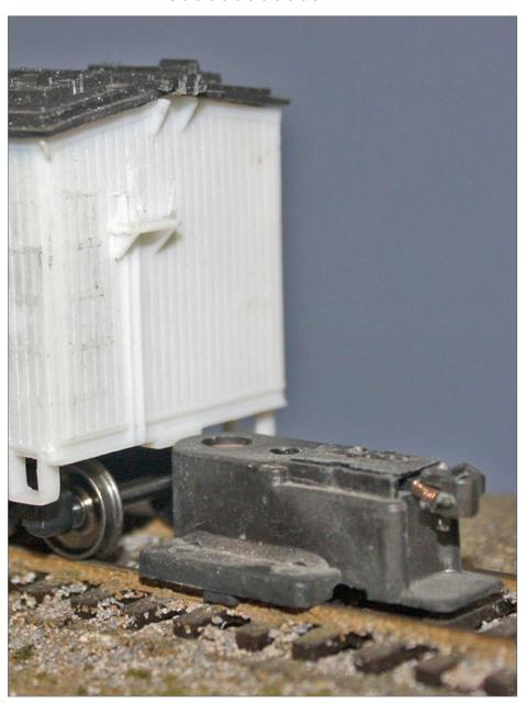
2. Here the back of the Kadee height gauge shows that the coupler pad on this car body is a little too low.
