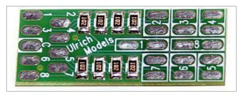
4. Ulrich Models resistor board allows connection of eight LEDs to "track level" decoder outputs. It comes with  $1K\Omega$  resistors, as shown. *Ulrich Models photo*
