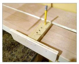
1. Bill made this marking gauge, which is basically a homemade T-square using scraps of plywood he had on hand. Bill drilled holes in the leg of the T to hold a pencil at the correct yard track locations, as measured from the front facia board.
