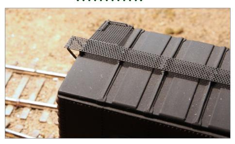
4. An example of a Morton etched metal running board, and wire corner grab iron.
