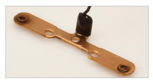
8. The truck side frames with wire soldered and shrink tubing providing some strain relief.
