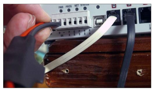
18. I hid most of the power wires' length under the shelf. They emerge just where they attach to the DCS240 terminals with screws. You can also see the five-amp automotive inline fuse covered in black shrink wrap.
