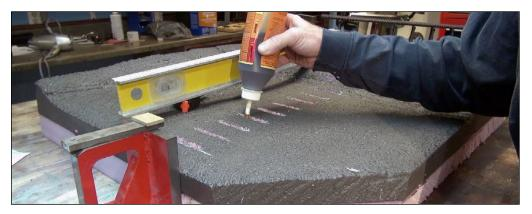
41. I filled the grooves in the foam with a bead of Gorilla Glue. I then placed the bridge on the scene, sinking it into the glue, and lining things up level and straight using a steel block on one end, and shimmed a little to make everything level.
