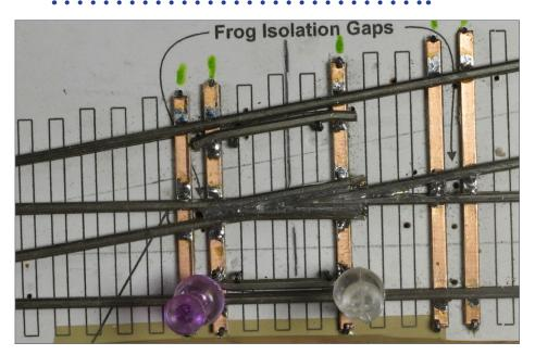
16. Soldering the guard rails in place.
