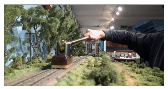
5. This worked really well, as you see in this photo with the gold breaker bar handle. This process lowered the center of gravity by half an inch, making it less top-heavy with the two and a half inch block of wood.
