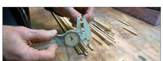
29. Going through my dowel rod stock, I looked for poles with a scale diameter of 13 or 14 inches. 3/16th-inch dowel rods fit this bill. I sanded the poles lengthwise with 80 grit paper, cutting wood grain into the dowels and decreased their diameter to about 12 scale inches.
