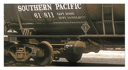
17. This detail from a photo of a Southern Pacific tank car with its reservoir readily visible shows the fresh stenciling for brake servicing. Tank cars often show brake stenciling very prominently because of the reservoir location. *Bruce Petty collection*
