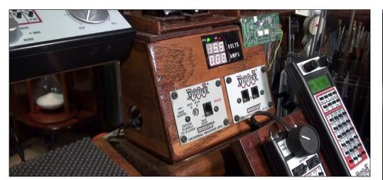
11. You will also notice the wood box with digital volt and amp meters. This was a project and article published in *Rail Model Journal* in December 2003. I built this box and added a Tony's Train Exchange RR-Amp meter and Digitrax face plates to have easy access to the LocoNet.
