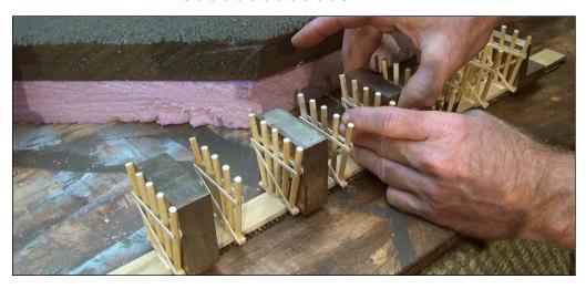
37. I glued the finished trestle bents to the bottom of the bridge deck on 14-foot centers using wood glue. I also used steel blocks to ensure everything was square as the glue dried.
