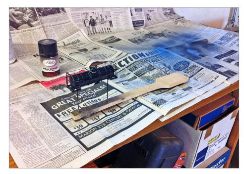
2. Douglas Dale Forbes' painting stand has a convenient grip at one end and allows access to all sides of the model.
