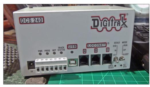
9. This month we look at the new DCS 240 power command station. I really like the new features included in this unit, like the USB port which will allow me to eliminate my Digitrax PR3 and all the wiring associated with that. It also comes with a built-in power booster for the programming track and means I can eliminate my Soundtraxx PTB-100 programming track power booster and all the wires attached to that. It is also convenient to have three Loco-Net jacks on the front panel.
