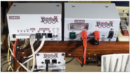
19. I attached the programming track wires, the LocoNet 6 conductor jacks, and the USB cable. That finished the hardware installation. With the power supply turned on, the DCS-240 lit up with colorful LEDS and sounds immediately started coming from my train on the main line. I turned the knob on my throttle and the train started running, just like that.
