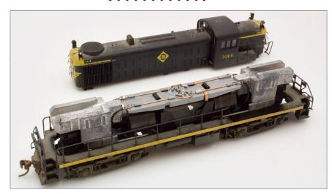
2. The interior of the Atlas RS3, showing the single centrally located bulb. The light pipes are inside the shell and not shown in this photo. The weights sitting on each end of the frame are not attached to anything. They are wedged into the shell when the loco is assembled. I call the assembly in front in this photo the "frame" and the one in back the "shell".
