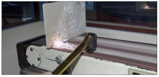
3. I had to redesign the tool to lower the center of gravity and did this by grinding down the square tip of the breaker bar to the spring-loaded ball. A belt sander or bench grinder will work for this. Keep a bowl of cool water on hand for this process.
