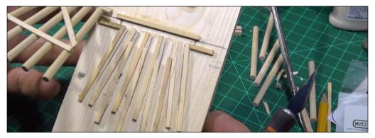
31. To build the jig, I glued HO scale switch ties to the jig surface, placing them on each side of the dowel rods leaving no space for movement or slippage. After the glue started to set up, I carefully removed the trestle bent from the jig, revealing my new trestle building tool.
