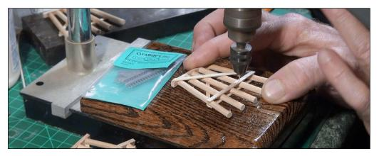
35. Using a #65 drill bit in a drill press, I drilled holes in 11 locations on each side of the trestle bents where the bolts would hold the structure together. I then glued Grandt Line  $2\frac{1}{2}$  inch bolt castings into each of the bolt locations.
