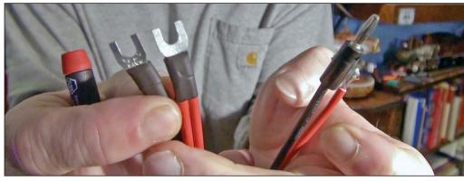
16. I modified the Digitrax power harness, removing two of the four wires but keeping the inline fuse in place. I cut off the crimped-on wire connectors and replaced these with banana plug jacks.
