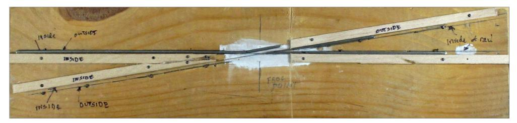
5. Frog assembly fixture with frog point and one closurewing rail.
