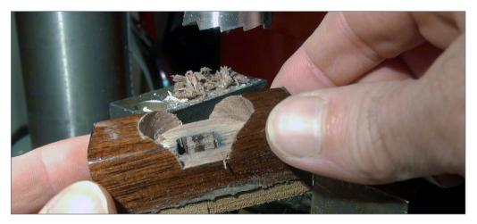
4. I then cut a bigger hole in the wood block to accept the breaker bar's round head. This lowers the tool's high pivot point and moves its center of gravity closer to the track.
