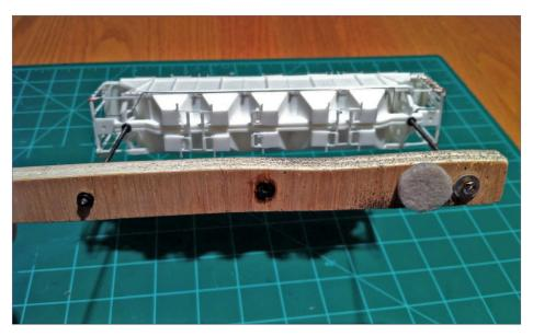
3. Threaded rods screw into the truck mounting bosses and can be spaced to fit different models by drilling new holes. The foam or fiber pad allows the holder to rest on the workbench.
