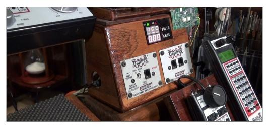
12. I also installed a Digitrax UR91 radio receiver in the wood box to allow good radio reception in that area of the layout room. I stained and varnished the control box to match the layout room decor.
