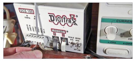
15. I pulled all the wires off the DCS 100's terminals They included the LocoNet six-wire connector, two track power leads, the two programming track wires and the two power supply wires. This unit will be programmed and used as a simple power booster to control another section of the layout as we add signals down the road.
