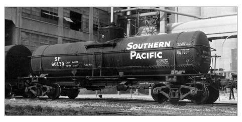
10. This SP tank car has a route card board (the pale rectangle above the running board, to the right of the ladder and above the brake cylinder), but the last clerk who attached a route card put it on the edge of the wood running board, above the left truck. The car, incidentally, is in cottonseed oil service and apparently empty; note the outlet pipe cap hanging from a chain under the car (this should have been closed). George Sisk photo at Kansas City, 1959, Charles Winters collection
