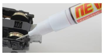
16. Applying Never-Stall **lubrication** to the rolling contacts on the loco trucks.
