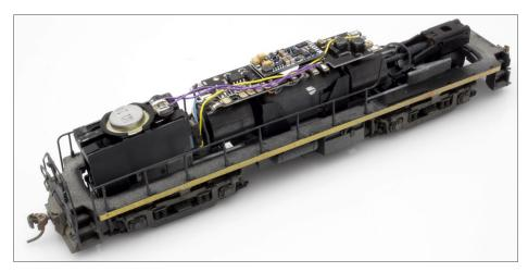
14. The finished frame, ready for shell installation. The lighting connector was plugged together with the white and yellow wires oriented to be together.
