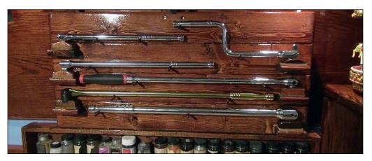
1. I have experimented further with this track cleaning tool concept by testing additional breaker bar handles of various types and shapes. Here you see a gun rack that I built holding the six sizes and types of track cleaners that have worked the best so far and are worth keeping. The gold breaker bar track cleaner with a dark varnished walnut head is simply a beautiful tool to see.
