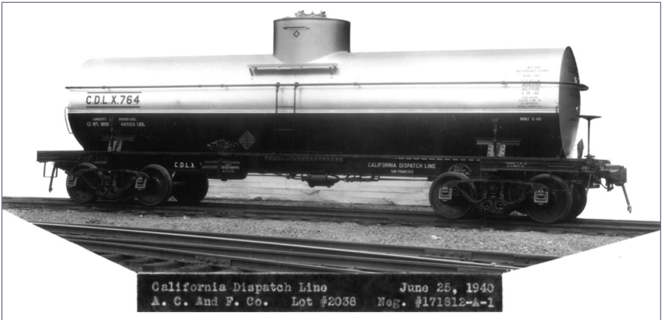
7. A California Dispatch Line insulated tank car, built for wine service, with National B-1 trucks. AC&F photo, courtesy Ed Kaminski
