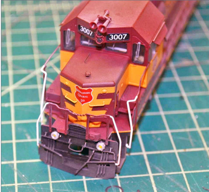
11. Installed ditch lights.
