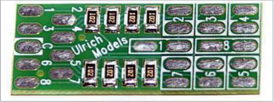
4. Ulrich Models resistor board allows connection of eight LEDs to “track level” decoder outputs. It comes with 1KΩ resistors, as shown. Ulrich Models photo
