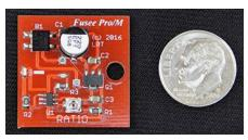
3. This gives you an idea of the Fusee PRO/M's size. It can sit across the rails from S through Z scale, and is powered directly from the rails. It will also work in O scale if you place it diagonally across the rails.
