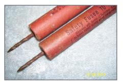
2. A railroad fusee typically has a spike in one end, so it's easy to embed upright in a railroad tie if desired.
