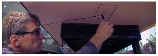
12. Underneath the layout, I used a Sharpie to draw a rectangle where the light hubs will be installed. I also drew a line from the auxiliary switch to the square where I will run the switch wires. Using a box knife, I cut a slot in the foam where the wire will run to the hubs. I used a screwdriver to press the wires into the slot, embedding them permanently in the foam.
