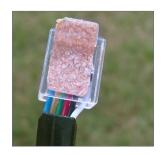
7. Attaching sandpaper holds the plug in place with friction and lasts much longer than the plastic locking clip.
