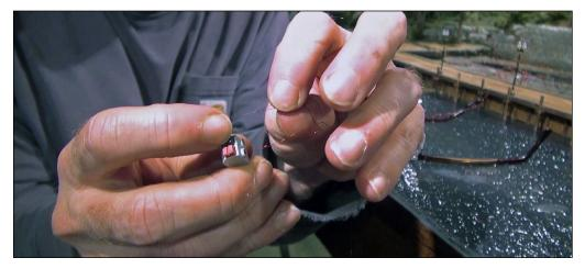
19. I twisted the fine wires, grouping three lights at a time and inserted these wires into the linker plugs supplied with the lights. Simply press down the buttons and insert the wires into the plug matching the color-coded polarity of red to red, and black to black.
