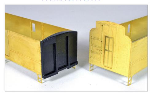
5. The two ends are joined to the basic box to finish the car body Note that the plastic end is attached to the shorter side of the car as measured from the small baggage doors.
