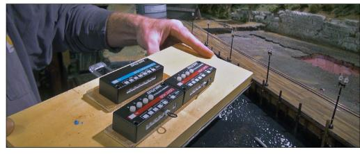
14. I used Gorilla Glue to attach two light hubs side by side in a piece of plywood. The expansion hub was also attached to its own piece of ¼-inch oak plywood. I set this aside for 30 minutes until the glue cured.
