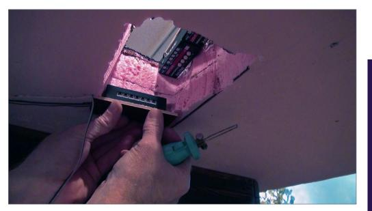
16. Using a hot foam cutter under the layout., I cut an additional space to install the expansion hub facing up, flush with the bottom of the layout.
