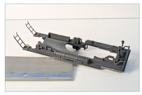
15. I cut off the cast air tanks and power reverse under the walkway on the fireman's side with a razor saw.
