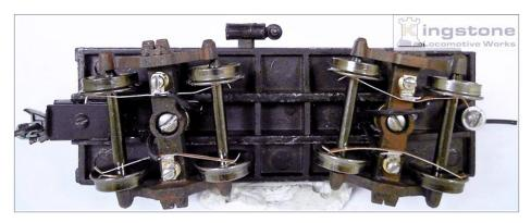
2. Bernd's design uses phosphor bronze wire and picks up directly from both wheels, creating a current path with as few wiping contact points as possible.
