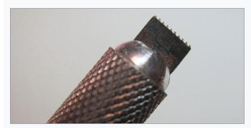
9. A 1/4" section of razor saw blade inserted in the handle of a hobby knife makes a great tool for creating wood grain in styrene siding.
