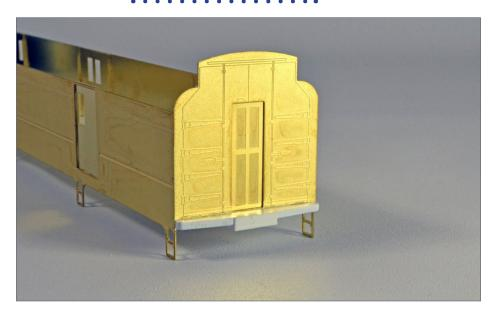
7. The fabricated end sill is capped with a piece of strip styrene cut to fit the width of the coupler mounting pad.
