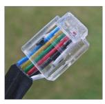
6. A damaged plug with the locking clip snapped off.
