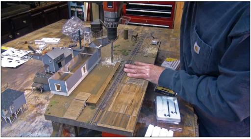
24. Using a 3/32-inch bit, I drilled eight holes through the <sup>3</sup>/<sub>4</sub>-inch plywood base to accept the lamps. I also drilled <sup>1</sup>/<sub>2</sub>-inch holes in the scene to feed the wires up to the buildings.
