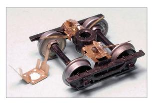
1. Harold Minky makes phosphor bronze wipers which contact the backside fillet of the wheel flange. Note the sprung contacts on top of the pickup panel to transfer electricity to the car body. Harold Minky photo
