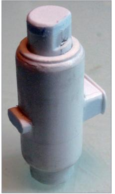
16-19. (Top and bottom left, and top and bottom right) Several telescoping sections of styrene tube, along with other basic shapes, were used to create the cylinder assembly for an early Fairbanks-Morse diesel engine. As construction progressed, additional parts were added, such as slices of hexagonal rod to represent bolt heads. In the final photo, the model has been sprayed with red primer. It will eventually be painted to look like a rusted relic.
