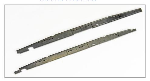
9. The center sill is modified by shortening and notching each end. In addition, the mounting tab is removed from each center sill's top.
