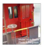
**Black Cat Publishing** has etched brass storm doors for both Canadian National and Canadian Pacific wood sheathed cabooses. CPR prototype doors had two window panes which were replaced in the summer with screens. CNR's wood storm doors have four
