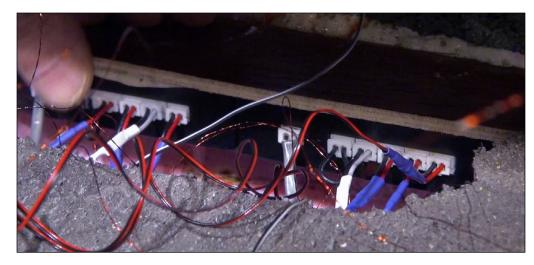
31. I plugged the five wired linker plug jacks into the open hubs on our light hubs one at a time, making sure they "clicked" when pressed in to ensure good conductivity of power for the diorama.
