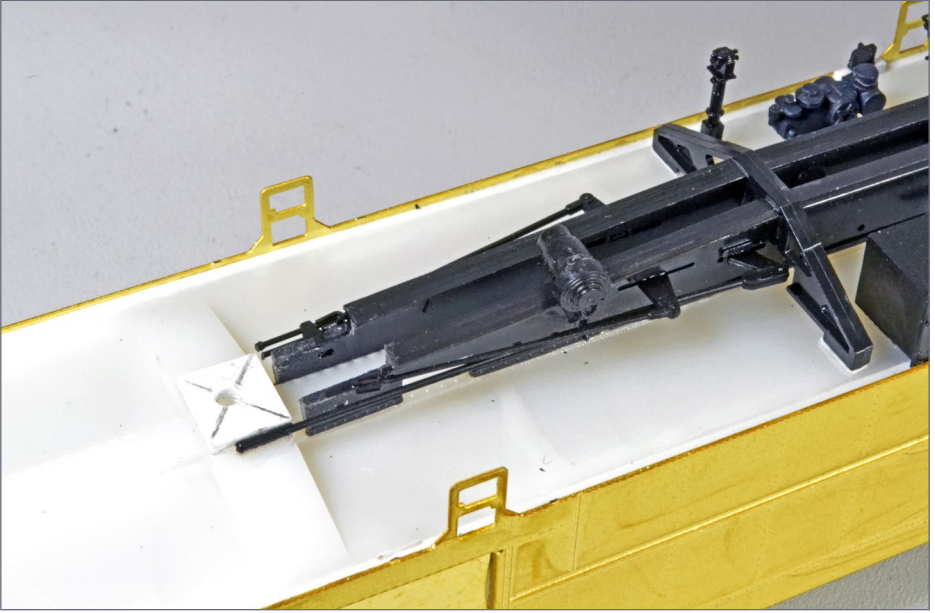
12. A closeup showing the brace beams, generator, and truck mounting plate.
