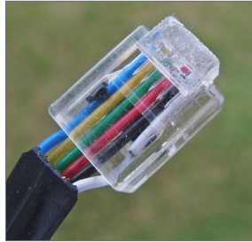
6. A damaged plug with the locking clip snapped off.
