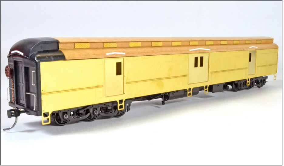
17. Overall view of the finished car after addition of the belt rail rivet strips before painting.
