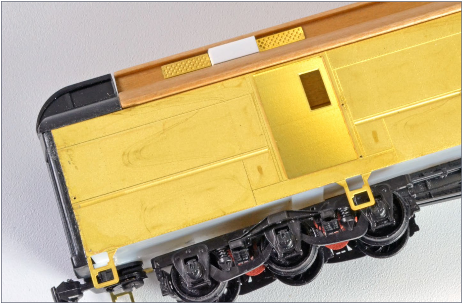
13. Eleven screen vents are super-glued to each side of the clerestory, using a styrene spacer.
