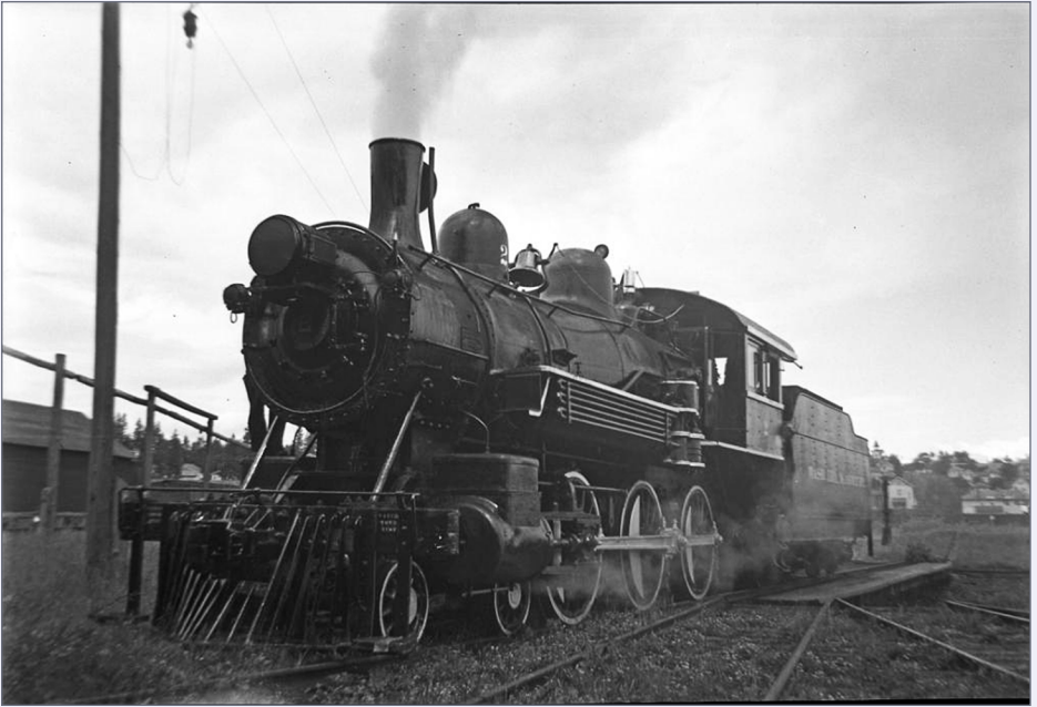
33. WI&M 2, also a 4-6-0, poses on the Potlatch turntable circa 1946. She had recently been overhauled, and decorated with white trim on the walkways and tires in hopes of attracting a buyer. Never outfitted with a superheater like her sister Number 1, she illustrates the as-built appearance of both engines with her original slide valves. Tom Kreutz photo, WI&M Ry. HPG collection
