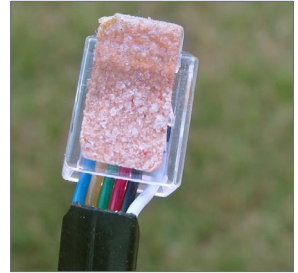
7. Attaching sandpaper holds the plug in place with friction and lasts much longer than the plastic locking clip.
