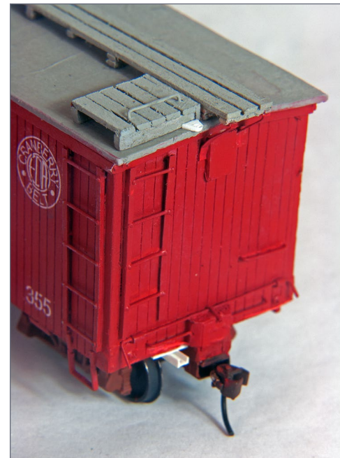
39. The upper brake shaft retainer is also cut from .020" styrene. Too small to really worry about the detail cast into the prototype.
