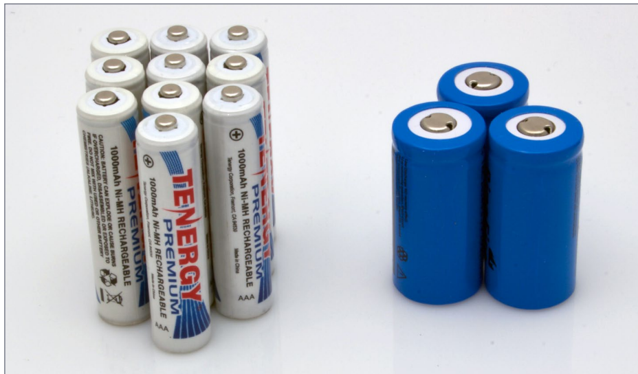
1. About 12 volts and 1000 mAh of storage: ten AAA NiMH cells or three (shorter) lithium ion cells. Bruce Petrarca photo
