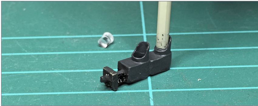
19. Light pipe being pushed into the housing opening.
