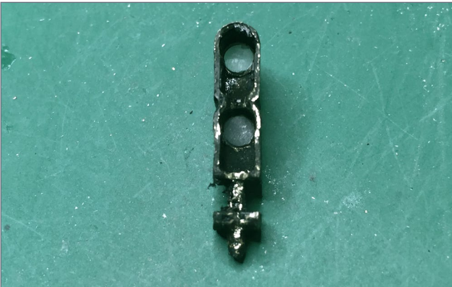
20. Light pipe in place from reverse side.
