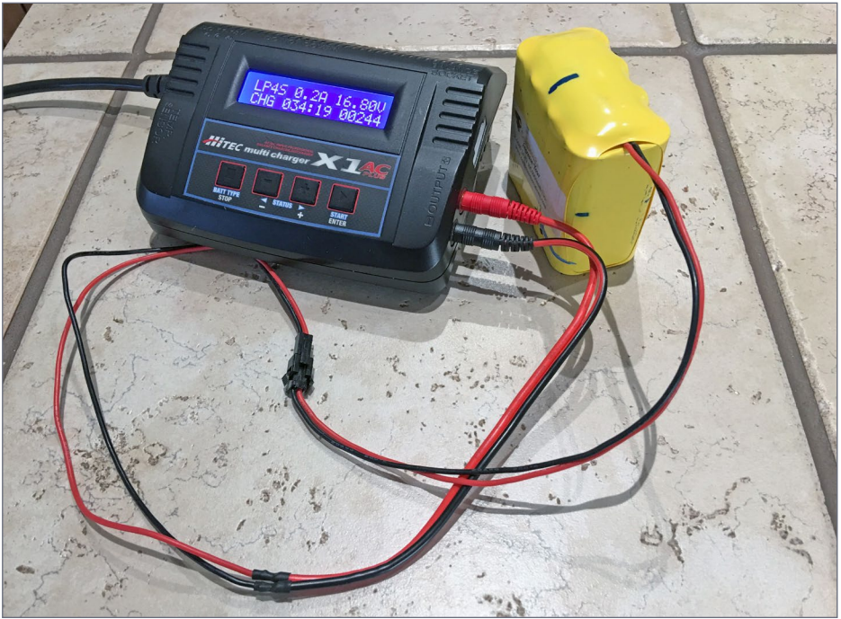
5. Charging a lithium pack on a nonflammable surface. Bruce Petrarca photo
