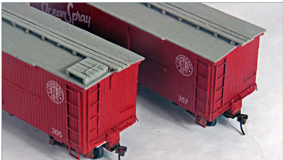
37. Showing the end platforms in place. Unlike those on most boxcars, the platforms were level and did not slope with the roof.
