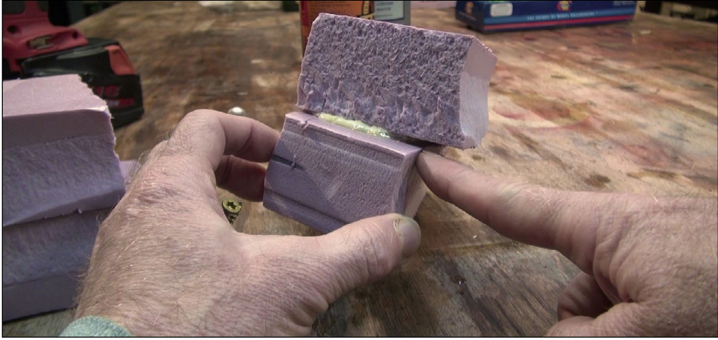
11. After 15 minutes, this joint shows signs of failure as the glue pushes the two foam sections apart.
