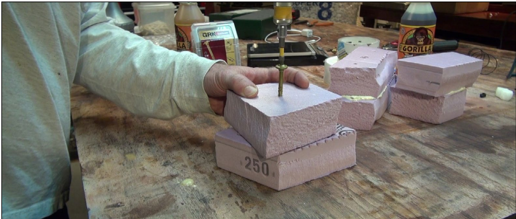
12. After thinking about it overnight, I picked up some 4-inch wood screws with large half-inch round pan heads. Using these larger screws, I repeated the experiment of gluing two sections of foam together using Gorilla Glue. After 30 minutes, the glue was hard with no visible expansion between the foam sections. I now had a good way to clamp/screw the foam in place while the glue cures and expands.
