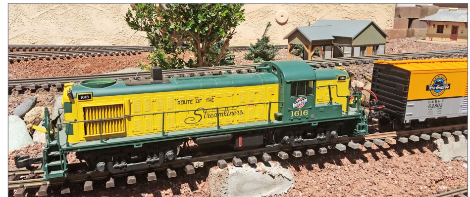
2. PCMRC's RS3 runs with a trailing battery car. Sharp-eyed readers will see the (silver-colored wire) antenna just sticking out in front of the exhaust stack and the inter-connecting cable of red and black wires between the loco and the Rio Grande box car. Bruce Petrarca photo
