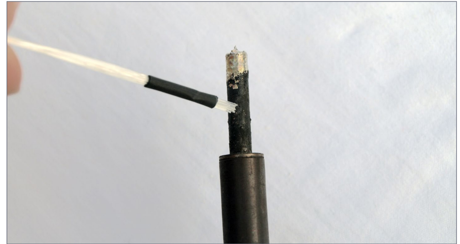
25. Using soldering iron to make light-gathering lenses.
