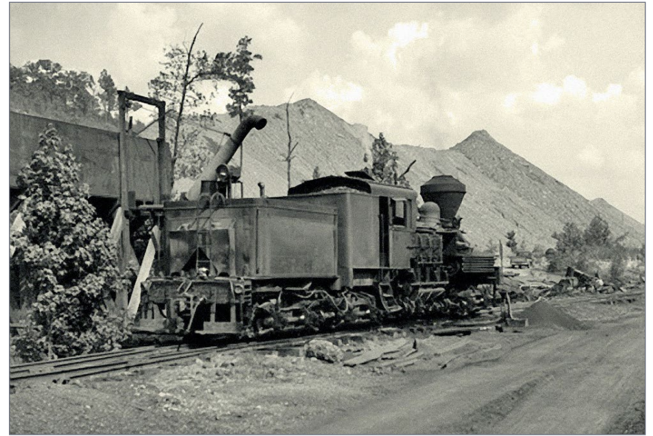
7. Shay No. 5 taking on water at the Kellerman water tank. The tank is a converted tender with a spout added. John C. Hawkins photo, hawkinsrails.net
