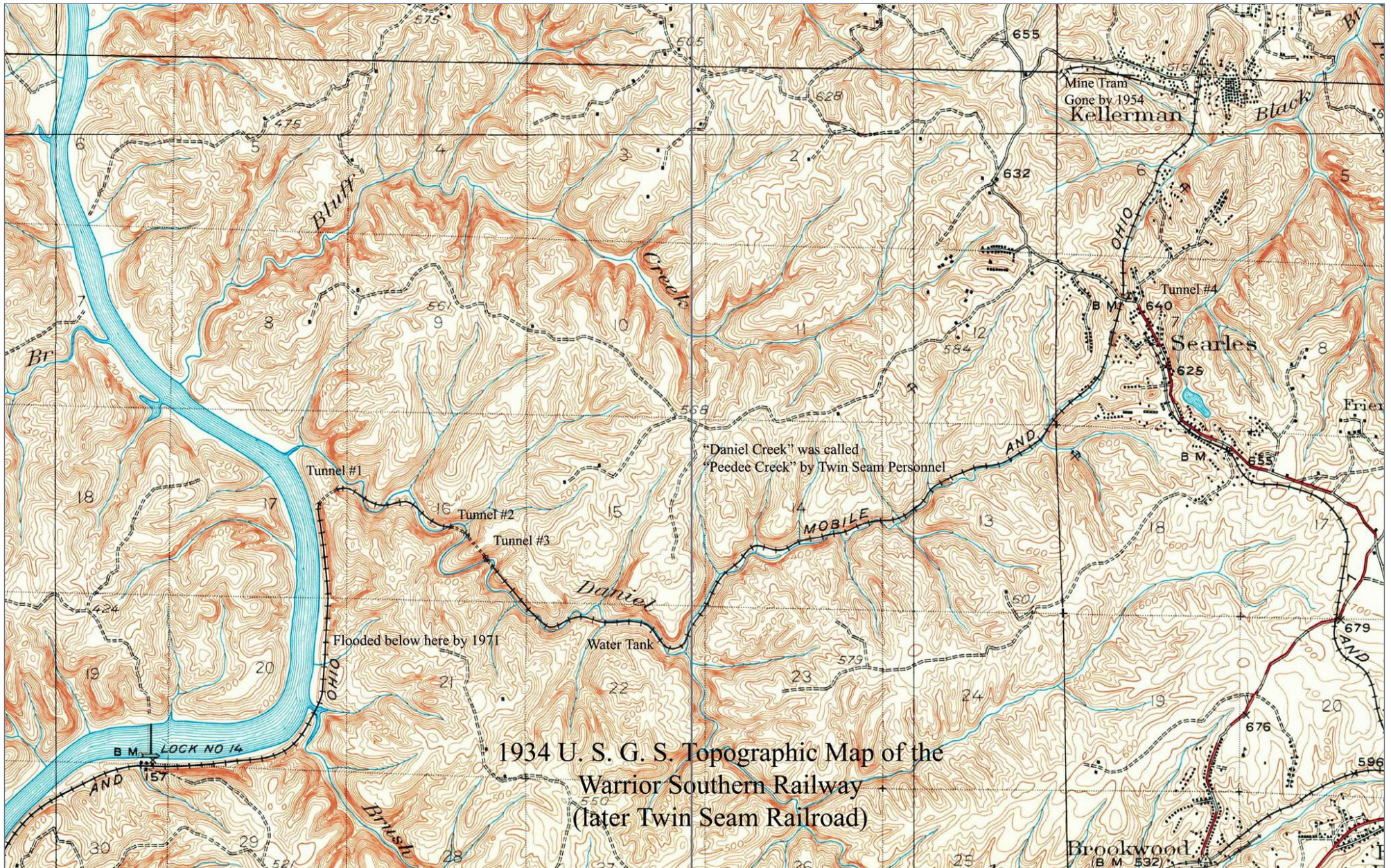
31. A 1934 topo map of the Warrior Southern Railway showing locations of tunnels and trestles
