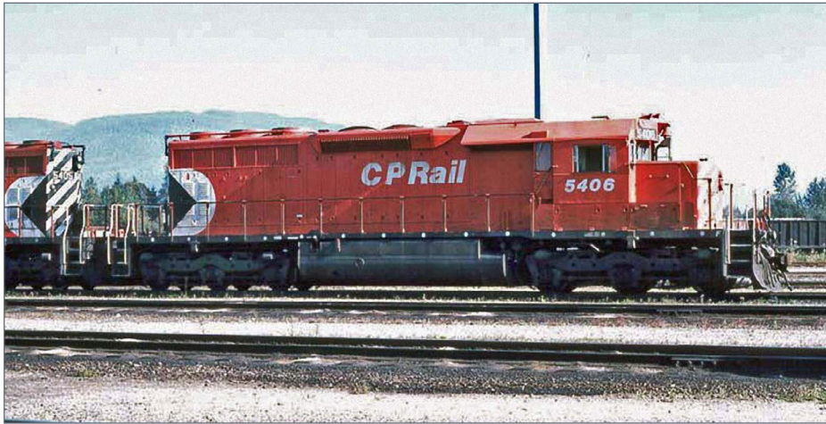
14. CP 5406 in Port Coquitlam, BC on October 11, 1986. Note the rounded dynamic brake fans. Claude Prutton mountainrailway.com
