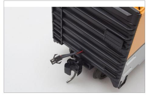
9. A-end of Piko battery car showing the male-pinned connector to mate with a loco. A bit of shrink tubing reduces the chafing on the wires when the connector is pushed back into the car after the loco connection has been made. *Bruce Petrarca photo*
