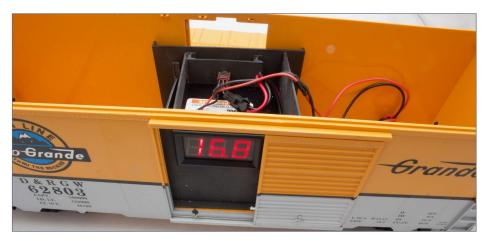
7. Side view of the Piko battery car showing the voltmeter. 16.8 volts indicates a fully charged battery. The batteries will hover between 15.25 and 14.75 volts for much of their life. Once they drop below 14 volts, it is time to turn off this battery car and charge it. *Bruce Petrarca photo*
