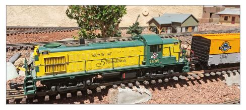
2. PCMRC's RS3 runs with a trailing battery car. Sharp -eyed readers will see the (silver-colored wire) antenna just sticking out in front of the exhaust stack and the interconnecting cable of red and black wires between the loco and the Rio Grande box car. *Bruce Petrarca photo*
