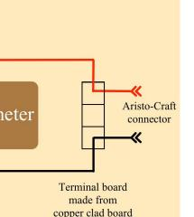
5. Schematic diagram for the battery car. I had no issues charging this battery with the digital meter connected. I used my X1 charger connected in place of the loco with the switch on. However, if your charger has issues connected this way, the charging connection shown (orange and gray wires in the diagram) could be added and used. If not needed, there is no reason for added confusion. *Bruce Petrarca diagram*
