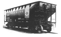
Kadee has scheduled an August release date for an HO scale ready-to-run version of this black Reading twin-bay coal hopper. Built in 1948, the AAR 50-ton car has flat ends and offset sides. All Kadee HO scale ready-to-run
