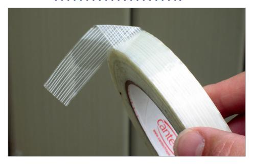
1. Ordinary reinforced packing tape is the key.
