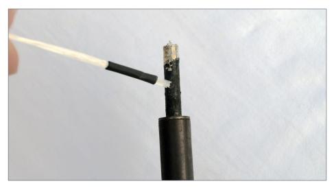
25. Using soldering iron to make light-gathering lenses.
