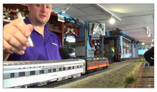
33. George backs a locomotive up to a car equipped with a Sound Car decoder. He waves a magnet across the roof of the passenger car and pushes F8 four times. This allows the freight car's decoder to look for or sense the locomotive decoder address and start making sounds when the locomotive is activated, to match the speed of the train. It's pretty amazing and watching the whole process in this month's video makes it look easy.
