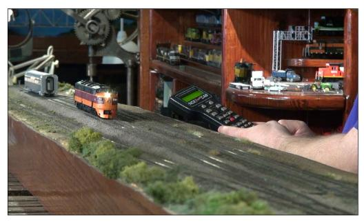
32. Because the E unit in this demo has two prime movers, George shows how to produce the 567 dual-prime mover sound by setting CV 123. When the model is started up on the layout, you hear each prime mover start up individually. Then he sets the bell type with CV 122. The decoder has 12 bells to choose from. The horn is programmed by setting CV 120 and there are 42 horn sounds in the decoder to match your locomotive.
