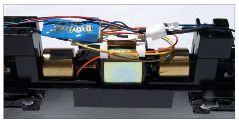
21. Completed wiring with orange and gray motor leads visible.
