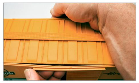
4. Removing the roof from the Piko box car. Open the doors, pull lightly out on the side wall just above each door. The tabs on the roof that engage the side walls should be able to be popped out, leaving the roof bowed from end to end. A slight tug on the end will release the end tabs. *Bruce Petrarca photo*
