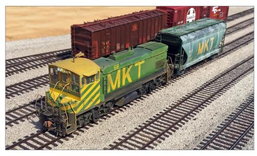
3. Scott Sanders modified a factory-painted Athearn Genesis MP15AC to match the MKT prototype engines. The big change needed was converting the Athearn MKT model from full-length handrails to the hand hold along the upper side of the locomotive found on Katy MP15ACs. Scott used. .012" brass wire to simulate this distinctive feature. For weathering, Scott used oils and powders. He shot the photo on his yard diorama depicting the locomotive flat switching at the Katy's Eureka Yard in Houston, TX.
