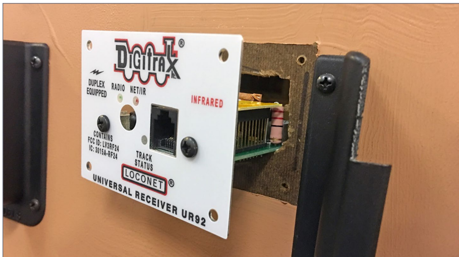
6. UR92 sitting in the fascia, ready to be screwed into place. Bruce Petrarca photo
