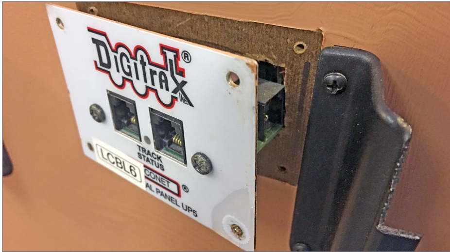
5. Mounting screws have been removed allowing the UP5 panel to slide out of the PCMR layout. Bruce Petrarca photo
