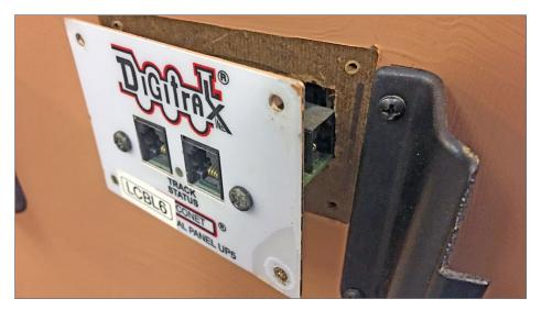
5. Mounting screws have been removed allowing the UP5 panel to slide out of the PCMRC layout. *Bruce Petrarca photo*
