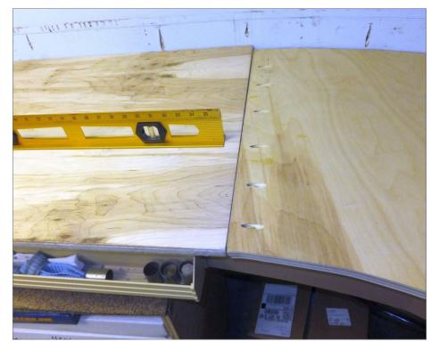
16. Since my clearances between the new Pittston Yard and the dropped staging yard were less than ideal, I decided not to use a conventional splice plate between the sub-roadbed sections and instead to use my new favorite tool: The Kreg Jig and pocket holes.
