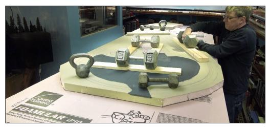
9. I place an assortment of weights and boards on top of this foam stack for about 30 minutes until the glue cures. Then, I cut around the edges of the new layer of foam until it is cut flush with the top layer.
