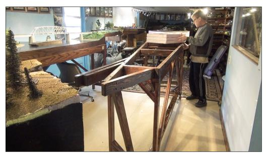
14. Now it is time to put all the pieces together. I roll the benchwork into position close to the bridge module that will connect with the sawmill diorama. If my measurements are correct, the rail height will match perfectly on both scenes as they go together. I slide the sawmill diorama on top of the smooth benchwork. I carefully position the foam even and square to the benchwork, matching marks I drew on the foam underneath to ensure an exact placement on top of the benchwork.
