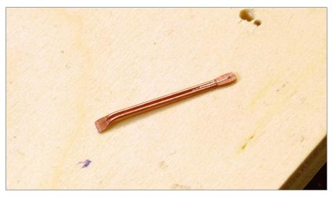
4. After flattening the ends, they need to be trimmed off and filed to make a smooth transition to the barrier.
