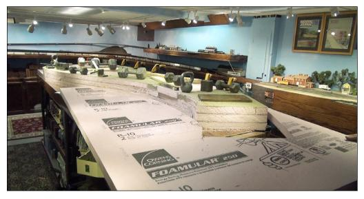
10. I repeated this process and glue a third layer of foam in to place, making the module six inches thick. I cut around this layer of foam with a Chinese pull saw, squaring off the sides of the module and pull away the excess foam to reveal the overall look.
