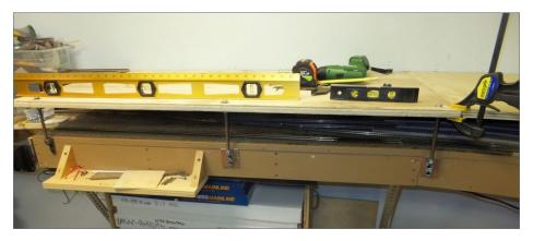
21. The temporary wood blocks have now been replaced by threaded rod. I recessed the nuts on top so they would not protrude above the cork. I'm using threaded pipe hangers as the bottom fastening point for the rod, since the new yard is slightly wider than the lower staging yard.
