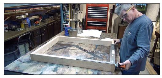
11. To hold the foam module I build benchwork from 2x4s, measuring from the floor to the top of the railhead. Every leg had to be cut to a different length as I was not going to use leg levelers on this project. Compensating for the uneven concrete floor ensures a level surface for the entire diorama.
