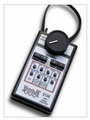
radio cabs from each other is the letter at the end of the model number (R = simplex; D = duplex) and the text near the model number ("RADIO EQUIPPED" vs. "DUPLEX EQUIPPED".)
