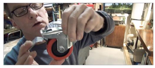
12. I attach these two-way locking wheels I found at Home Depot. It is very important to be able to both lock the wheel and to also lock the pivot. Locking this pivot point ensures the module won't wiggle from side to side, ensuring solid and tight benchwork.
