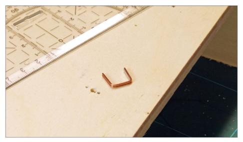
5. After bending the barrier to a U-shape, I soldered 0.5 mm (AWG 24) brass wire to it to make a mounting post.
