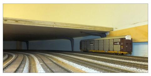
20. I'm using an autorack to check my clearances for the back track. Clearances are tight, but it works.
