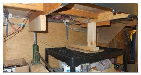
6. How do you raise a layout section by yourself? Why, with a hydraulic jack, of course! Once Ransom had been disconnected from the wall, it was simple to jack it to the correct height and reattach.
