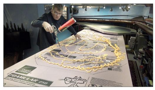
8. I then start stacking or layering two-inch-thick sheets of foam, gluing them together with Foam Pro Adhesive.
