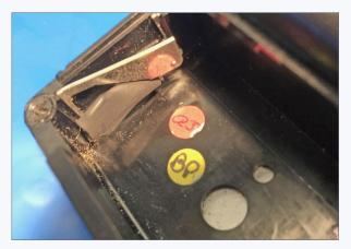
8. UT4 cab spring end. Shrink tubing has been added to the lower spring. This shows a "before and after" of the installation, making it easier for the shape of the metal spring to be seen in a photo.
