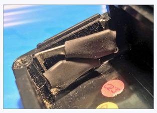
9. UT4 cab with the tubing installed and shrunk. I did both sides of the spring. Theoretically, only one needs to be insulated. However, I believe in over-kill for safety.
