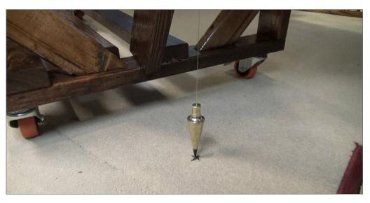
17. I also attach or hang brass plumb bobs to each end of the benchwork. These will point to an X on the floor when the benchwork is positioned in the room. This ensures the modules will be replaced in their exact location in the room after being moved for maintenance or photography. When the benchwork is back in its location, make sure each plumb bob points to its X. Then simply lock the wheels, slide the rail joiners on the track into position, and you're ready to run trains.
