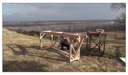
13. I rout all the corners on the wood benchwork with a  $\frac{1}{2}$ -inch curved bit. I then sand the wood with 150 grit fine sandpaper to make everything smooth to the touch. I then stain the benchwork with red oak stain and applied three coats of polyurethane to give the benchwork a furniture-quality appearance.
