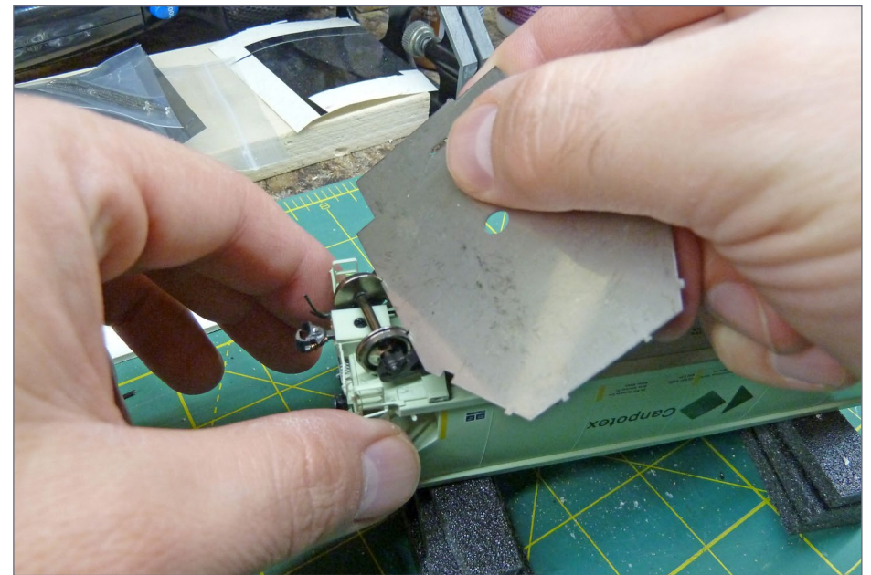
7-8. Checking the wheel gauge.
