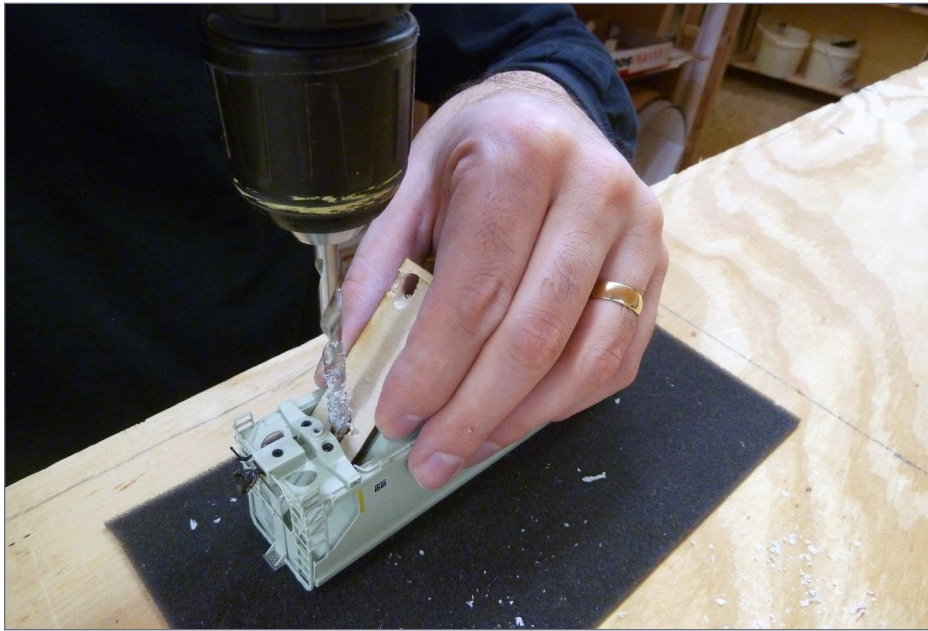
13. Drilling the openings.
