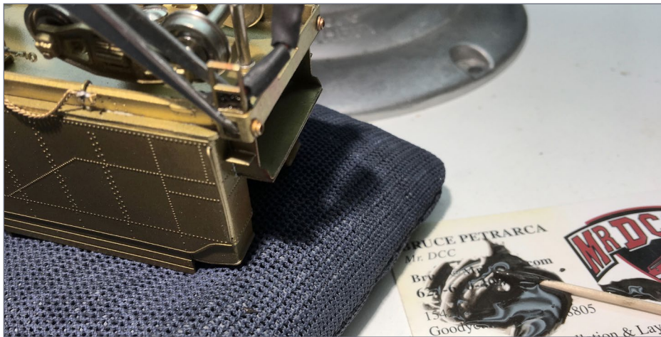
8. Applying JB Kwik Weld to hold heat-shrink tubing in place on a loco tender. Bruce Petrarca photo
