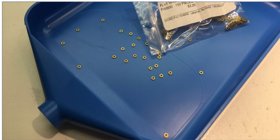
12. Small parts can be poured into a sorting tray, used and the remainder poured back into the bag. Bruce Petrarca photo
