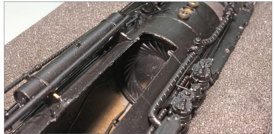
13. A 28mm speaker installed into the boiler of an HO 2-10-2. Bruce Petrarca photo
