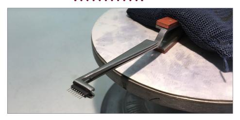
11. Clamping tweezers holding a multi-pin header. The tweezers are positioned on the decorating wheel by a shot bag. Bruce Petrarca photo
