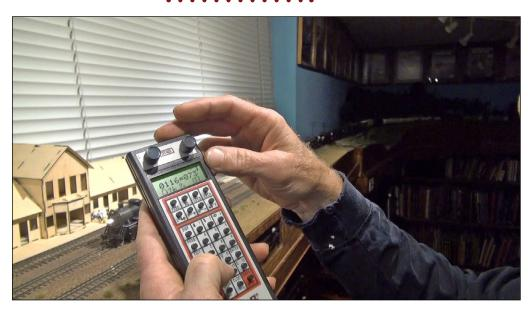
24. In the video, we take the model inside and set up the sound decoder's DCC quartering of the drivers and the delay or momentum to enhance the performance of the model. To match sound to the quartering of the drive wheels, we use CV 116. Through trial and error, I eventually found that programming CV 116 to 73 synchronized the wheels perfectly with four chuffs per revolution of the main driving wheels.
