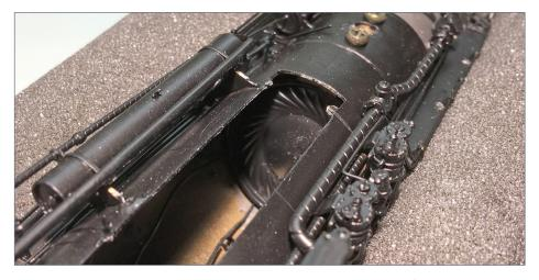
13. A 28mm speaker installed into the boiler of an HO 2-10-2. Bruce Petrarca photo
