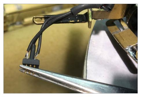
2. Three-pin male connector being wired to the loco. *Bruce Petrarca photo*
