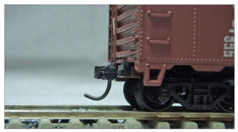
4. "Dilberted" gladhand that has been bent up too far. This coupler won't work correctly over magnets.
