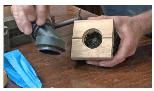
10. After cutting off the brush handles, I start making a vacuum attachment by cutting the synthetic fibers off of a two-inch round brush. Once the fibers are cut off, match the diameter of a Forstner wood hole cutting bit to match of the diameter of the vacuum cleaner attachment. Drill this hole through the fibers, wood, and nails holding the fiber hair in place in the brush. Then, test-fit the black brush attachment into the hole. Everything should fit together perfectly.
