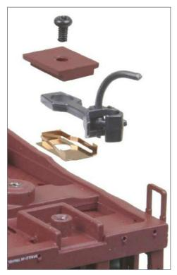
3. Kadee #5 coupler and spring installation, done correctly. *Photo courtesy Kadee, Inc.*
