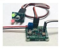
Tam Valley Depot has introduced The Turtle, a stall motor driver and DCC decoder capable of driving a Tortoise switch machine as well as other stall-motor based switch machines including Switch Masters, Cobalt, and higher current MP1 and MP5 units. For complete details and ordering instructions visit tamvalleydepot.com.
