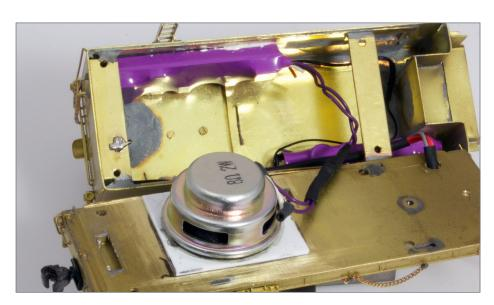
7. Tsunami decoder and CurrentKeeper mounted in tender shell. *Bruce Petrarca photo*
