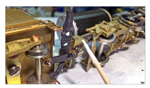
6. Marking the correct polarity on a plug and socket with a toothpick and white paint. *Bruce Petrarca photo*
