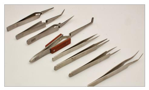
10. I use a bunch of tweezers, both regular and clamping styles. I prefer non-magnetic stainless steel whenever I can get it – most of the clamping ones are magnetic, alas. My favorite is the curved version in front. *Bruce Petrarca photo*
