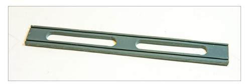
4. MLR Engineering produced this 8" resin tool for aligning flex track. It's also useful for cutting rail ends to match. Hardwood or aluminum could be used to make a similar tool. MRH photo
