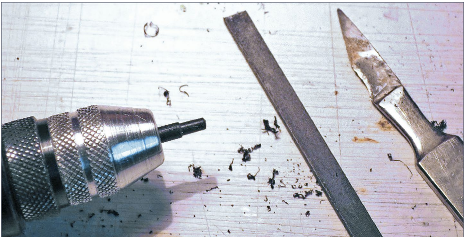
22. Using the sprue as a starter piece, I turned the parts.
