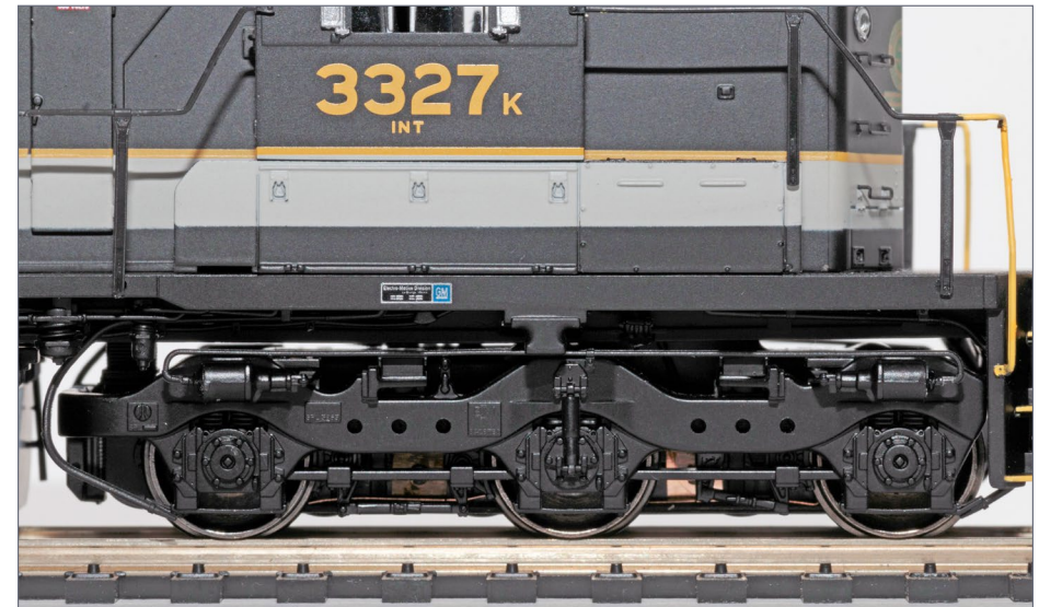
3. Closeup of HT-C truck and builders plate detail.
