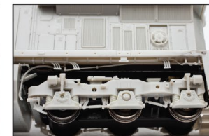
Separately-applied plumbing and traction motor cables.
