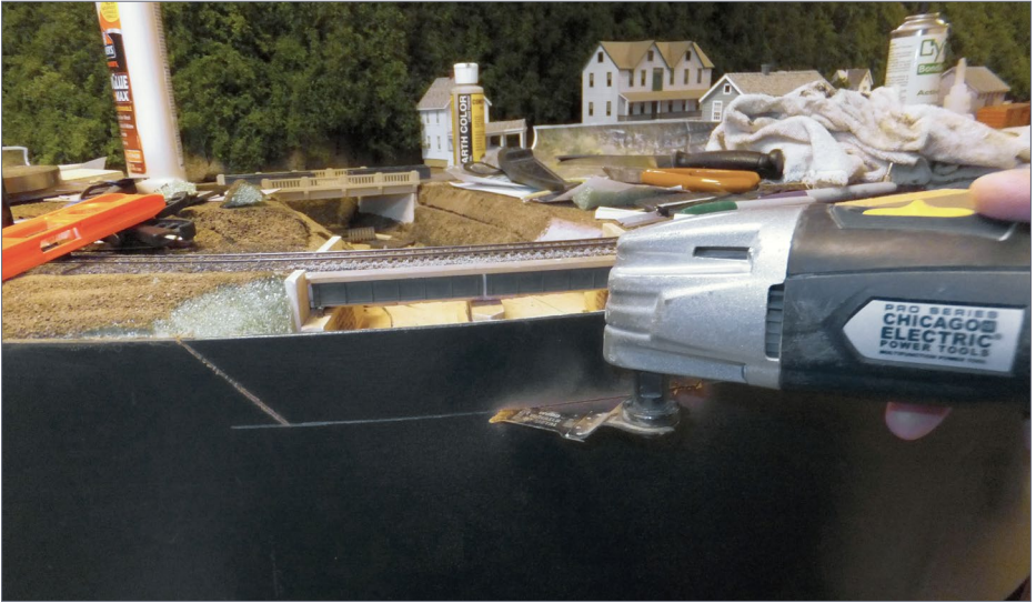
49. The horizontal cut was easily made with an oscillating “vibro saw.”
