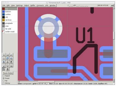
8. Thermals connect a SMT pad (top) and a via (bottom) to the power and ground planes. The board is seen from the top. The blue color shows areas where there is copper on the bottom layer but not on the top layer, and the white area is where there is no copper on either side of the board.
