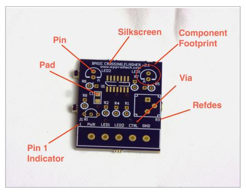
3. This is the completed example circuit board, with examples of the different parts identified.
