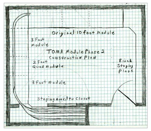
10. Phase Two plan showing the staging yard section moved to the closet, and three additional modules added to the left side of the room.
