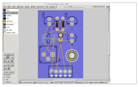
7. I cover the top (red) and bottom (blue) of the board with copper planes (board rotated vertical here). When I later draw traces, they will be carved out of the planes, leaving as much of the board as possible covered in copper.
