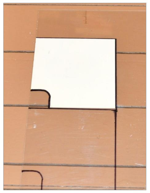
13. I didn't have enough corner pieces for the intersection, so I made my own from styrene using a clear plastic template drawn using one of the kit pieces.
