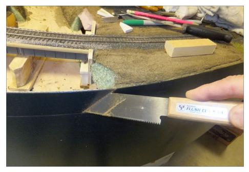
48. Side angle cuts were done by hand with a flush-cut saw.
