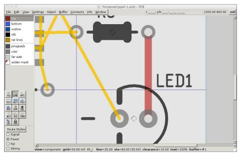
6. Yellow "ratlines" show wiring connections that have not yet been "routed" or drawn on the board. The red line is a "trace" (connection) that has been routed on the top copper layer.
