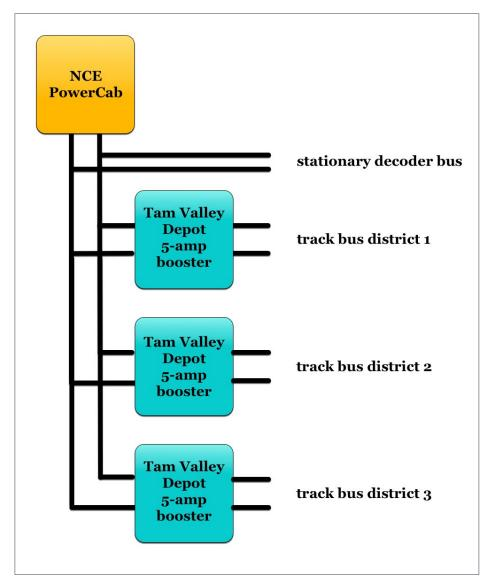
7. Using a NCE PowerCab and Tam Valley Depot boosters to provide three 5-amp districts without the use of circuit breakers. This version provides more power for less money than a five-amp system with three circuit breakers. *Bruce Petrarca diagram*
