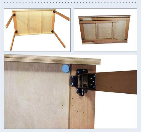
16. (Left bottom) This photograph from Kam Konnect shows how a dropdown module is built with 18mm Baltic Birch (13 plies thick, total 3/4") plywood sides and ends. The base is 1/4" hardboard with 1/2" foam board for scenery. I will add 12mm (1/2") cabinet-grade plywood for the track roadbed.
