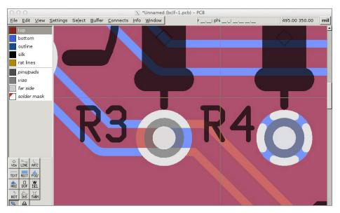
9. The pin on resistor R3 acts as a via for the trace connected to it. The pin on R4 is connected to the ground plane (blue) on the back side of the board with a thermal.
