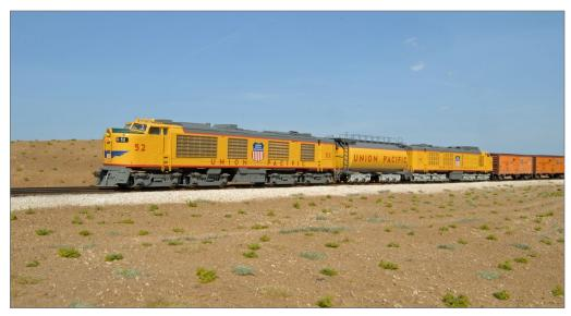
12-13. In 1958, UP ran two turbines back to back for six months. Turbines 59 and 60 became a 9000-horsepower set with a fuel tender coupled between the units. All the standard turbines were retired by 1964.
