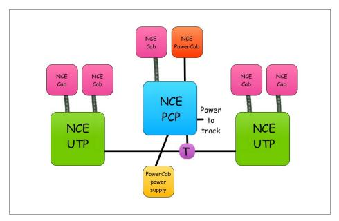
8. Cab bus diagram to allow multiple points for connection of NCE cabs to the system shown in [7]. The PowerCab will not support as many additional cabs as shown in this figure, typically three of the five shown. *Bruce Petrarca diagram*
