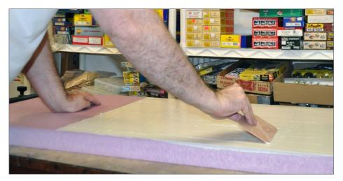
10. I applied Liquid Nails adhesive evenly to one piece of foam in preparation for laminating it to another piece of foam.
