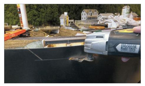
49. The horizontal cut was easily made with an oscillating "vibro saw."
