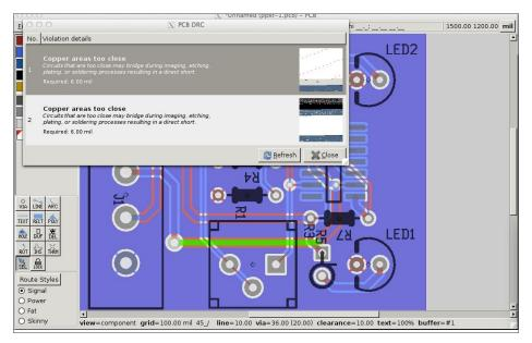
11. The DRC tool highlights a trace that is too close to other traces in bright green. If the trace is not moved, variations in the manufacturing of the board may cause the trace to short out to adjacent traces.
