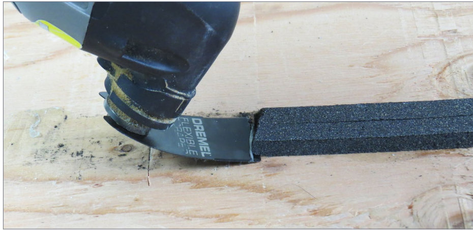
12. The flexible scraper works great for lifting cork roadbed.
