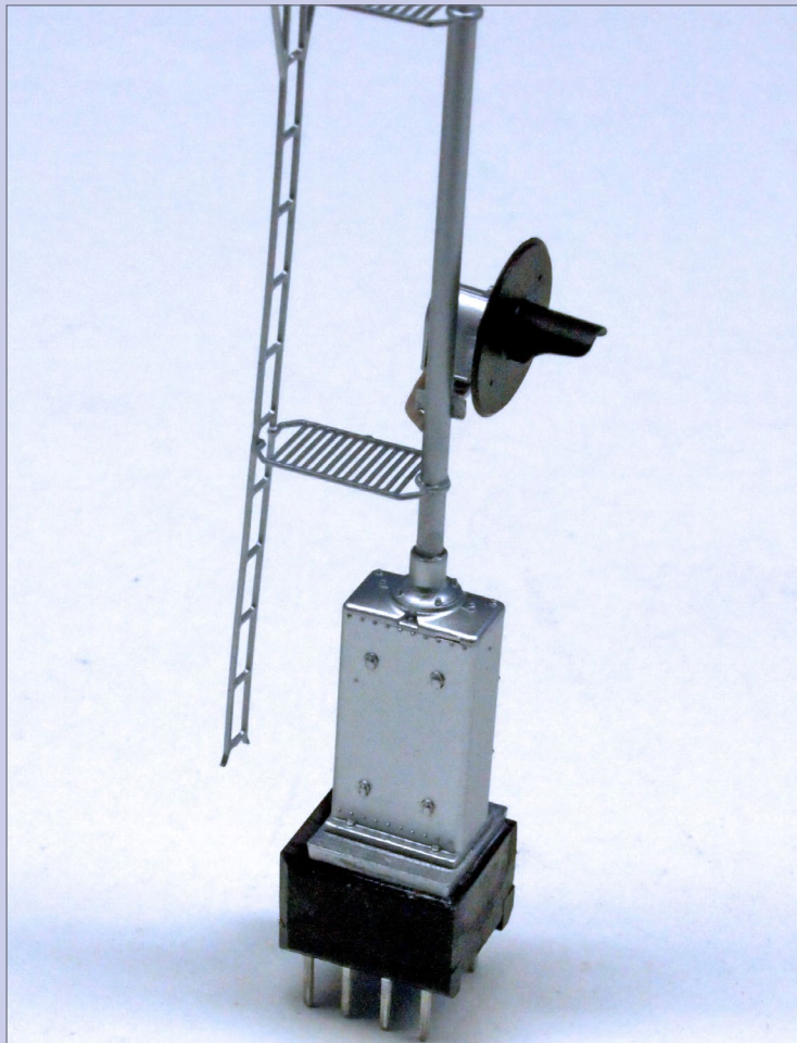
18. Finished DIP plug base on the signal, snapped together and ready for final testing.
