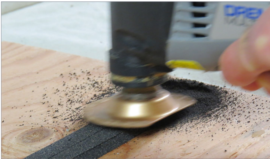
9. The grinding attachment makes short work of tapering cork road bed.
