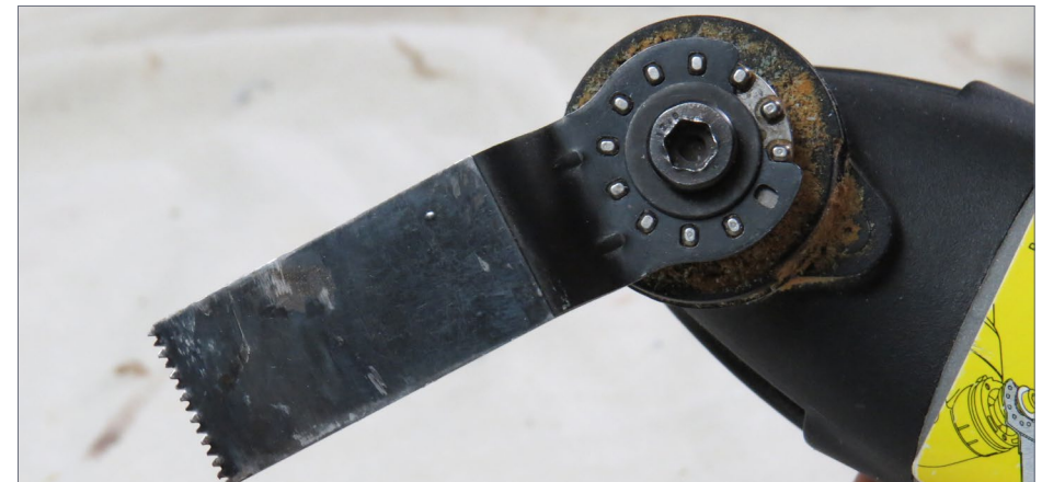
7. The tool's unique blade attachment system allows almost unlimited angles for attaching blades. This is fantastic for tight spaces.
