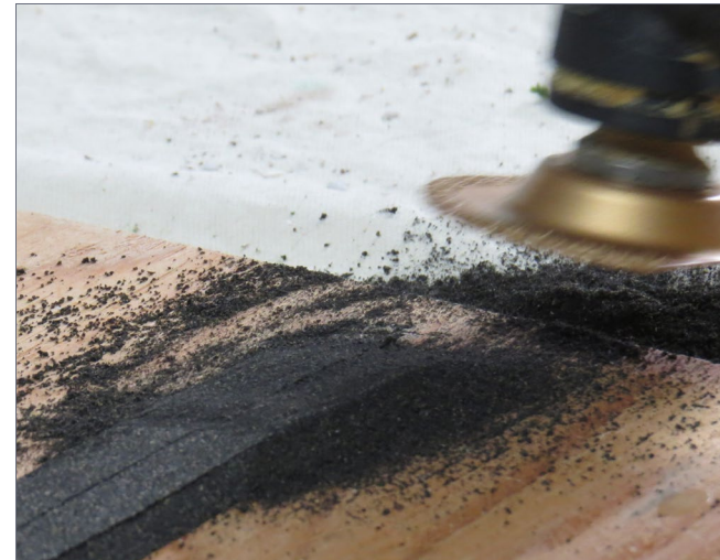
10. The grinding attachment is touted as being for tile grout removal, so you will get a lot of roadbed tapered before it wears out!
