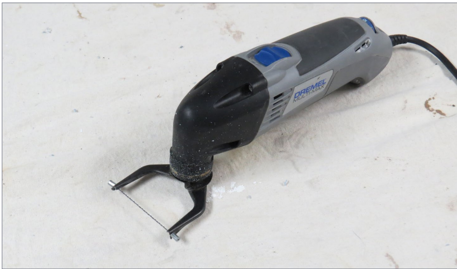
13. Here is the coping blade attachment.
