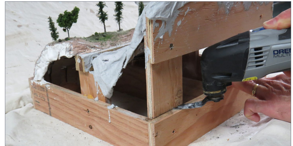
6. Here is a great example of the flush-cutting capabilities of the tool.
