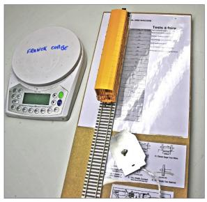
4. A test plank gathers all the tools and tests needed to check a car or locomotive before it is handed off to operating crews on the layout, and is useful in any scale and gauge. Tethering the NMRA gauge keeps it from walking away. Franck Combe photo
