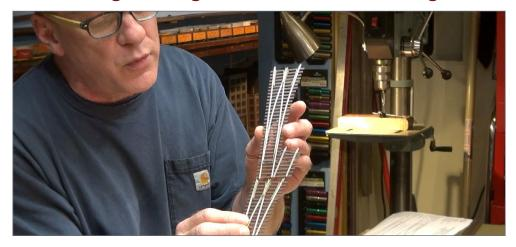
12. This past year, Micro Engineering introduced a new ladder track building system using very specialized #5 turnouts where the points for the next turnout start directly after the frog.
