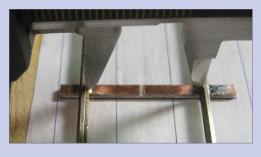
gauge to double check track spacing before and after soldering. Note that the track gauges are only useful until the stock rails begin to diverge. After that, you will need to rely on your printed plan for placing the curved stock rail. This is okay, because we will use the track gauge later to make sure everything is correct when soldering the point rails [16].
