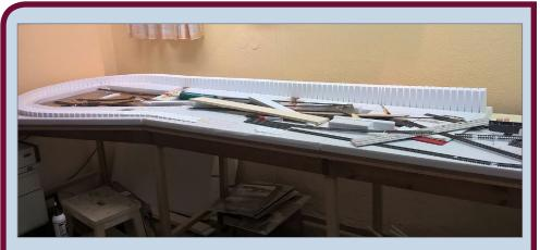
2. All grades on the layout are 2% and made with Woodland Scenics Subterrain foam products. That proved to be a most elegant solution, especially for a sectional layout where there is a need to cut the grade in several places due to the length of the modules.
