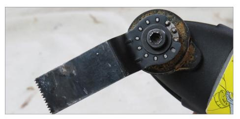
7. The tool's unique blade attachment system allows almost unlimited angles for attaching blades. This is fantastic for tight spaces.
