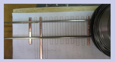
**10. Position the stock rails:** When the two stock rails are ready, carefully align them on the PC Board ties and weight them down so they don't move. I use spools of solder as weights since they are very heavy, flat on the bottom, and just about the right size.
