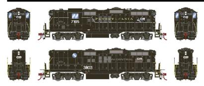
A Conrail GP9 will be offered (No. 7105) as well as a cabless GP9B unit (No. 3803). Both are ex-PRR diesels decorated in Athearn's faded Primed-for-Grime paint scheme.
