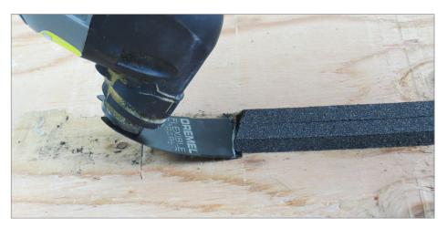
12. The flexible scraper works great for lifting cork roadbed.
