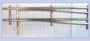
cedure, weighting the rail and checking gauge as I went, except when I reached the throwbar. The points must be able to move, so to accomplish this, I placed a PC board tie as a shim temporarily between the straight stock rail and the curved point rail. I soldered the point rail to the throwbar and then removed the temporary PC tie shim. This left a gap that allows the points to move. I then removed the completely soldered scale track from the template.
