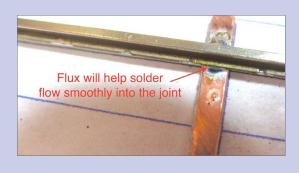
dering iron against the web of the rail. I placed the solder against the PC Board tie at the base of the rail, and kept the hot iron on the joint until the solder flowed. The solder should flow *under* the rail making a solid joint. Excess solder outside the joint is not necessary. The Fast Tracks site has some excellent videos on proper soldering techniques: [handlaidtrack.com/FTV-Turnouts-5].
