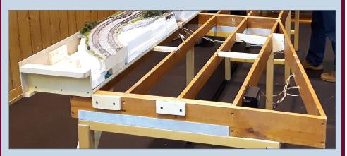
3. The image shows what the sub-base frames look like before adding the module board. At the back side there is a 10" popular board fixed to the frame, carrying the tracks and some backdrop scenery. This way Erik could handle and carry the frames with ease.
