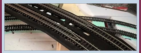
5. I made the long bridge that spans over three modules removable as well. With it spanning three module sections you would at first think it also should be three pieces, but that is not something I would recommend. I made the bridge deck as a single piece from two thin MDF boards (with laser cut openings) and laminated them together for additional strength.
