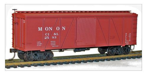
3. Accurail's new Fowler boxcar kit is a good example of a 1920s freight car, with wood sides and ends, stem-winder brake wheel, and a relatively low interior height. *Accurail photo*
