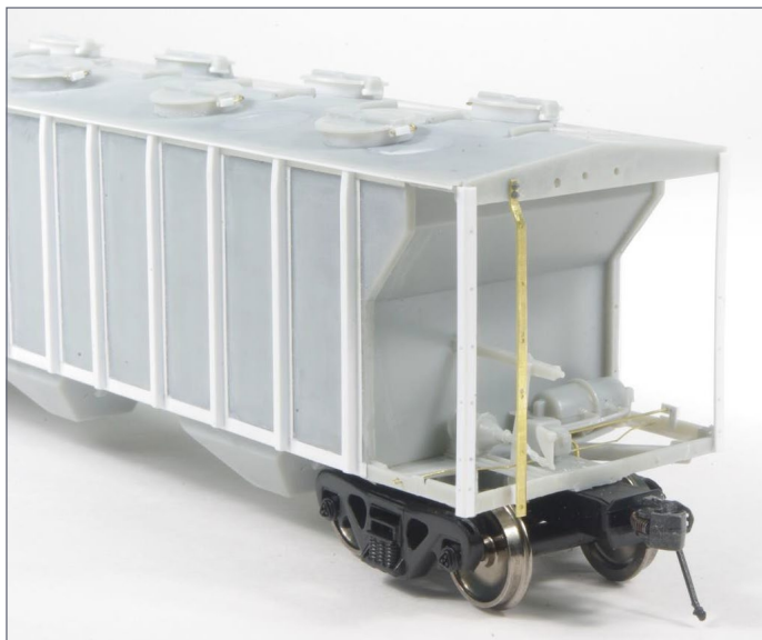
20. New corner posts and ladder post glued in place.
