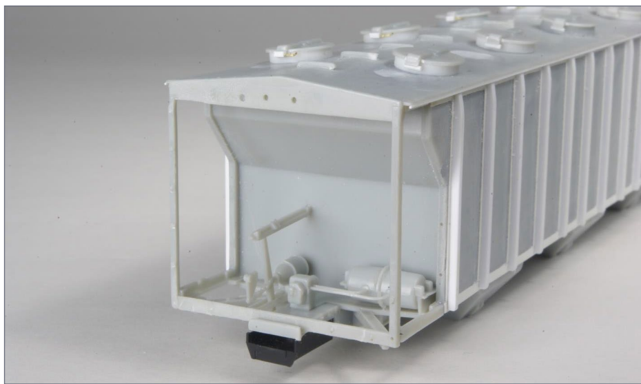
13. End cage frame glued in place with vertical posts removed.
