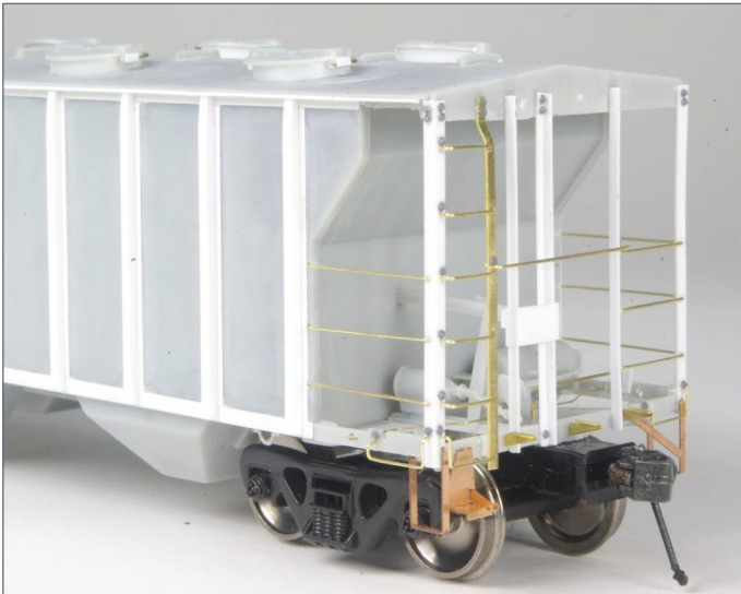
22. B end of car with grab irons, stirrups, and other details in place.
