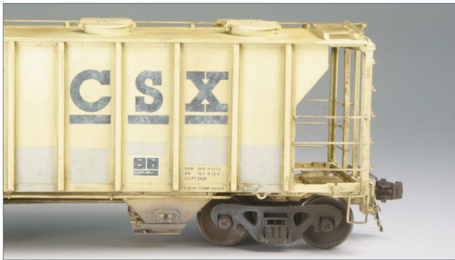
40. Patches added to side of CSXT 223144.
