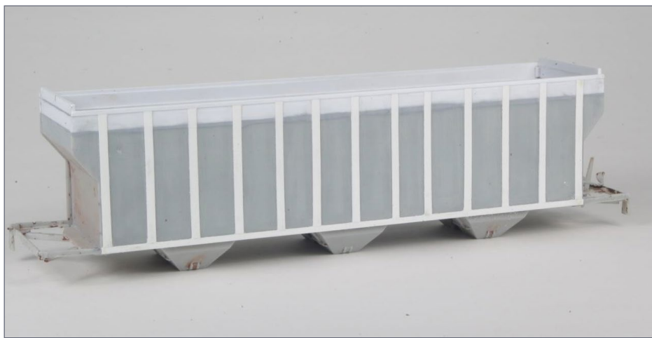
34. Hopper body extensions complete, including ends.
