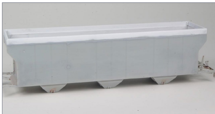
31. Extension added to hopper body.
