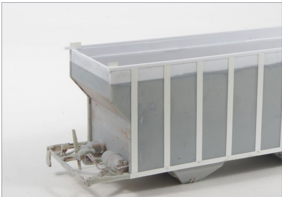
33. Pieces of .005" styrene added to hopper ends. They still need to be trimmed.
